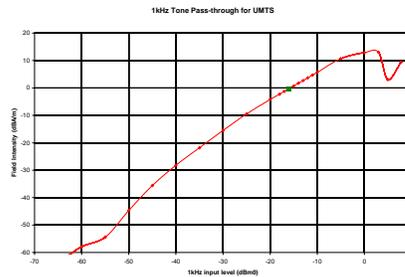
This model was verified to be within the linear region for ABM1 measurements at -18 dBm0 for CDMA. This measurement was taken in the axial configuration above the maximum location.
