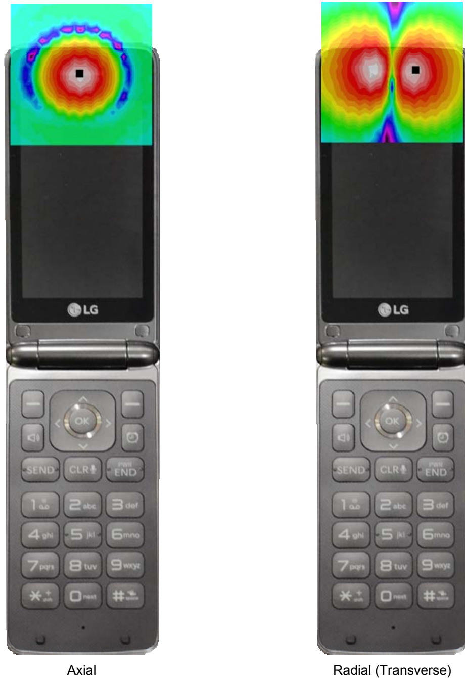
Figure 13-3 T-Coil Scan Overlay Magnetic Field Distributions
