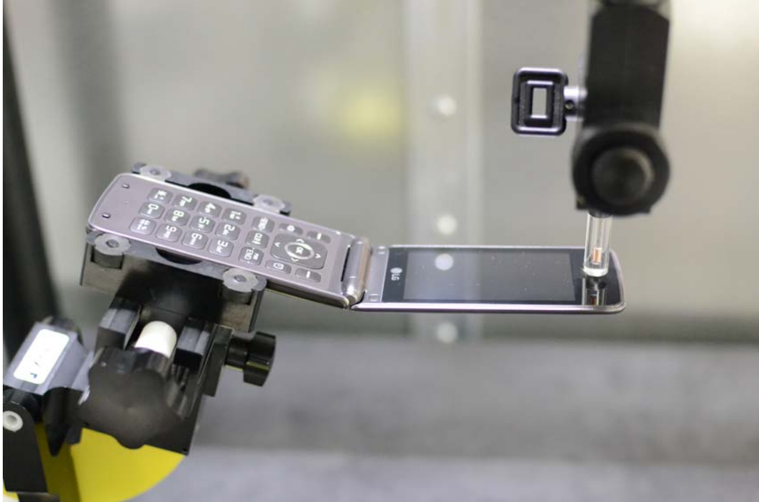
Figure 13-1 Test Setup for Wireless Device
