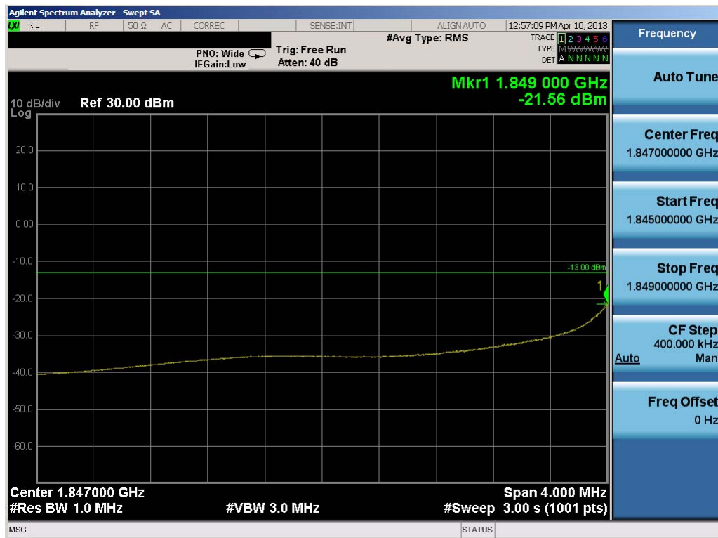
Plot 7-15. 4MHz Span Plot (PCS CDMA Mode – Ch. 25)
