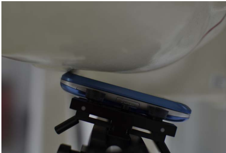
SAR Test Setup Photo 2: Right Tilt
