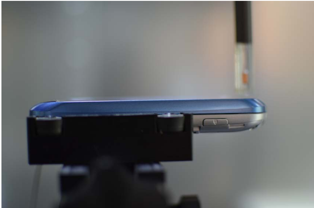
Figure 13-2 Test Setup for Wireless Device
