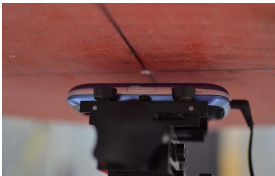
SAR Test Setup Photo 6: Back side at 1.5 cm with headphones
