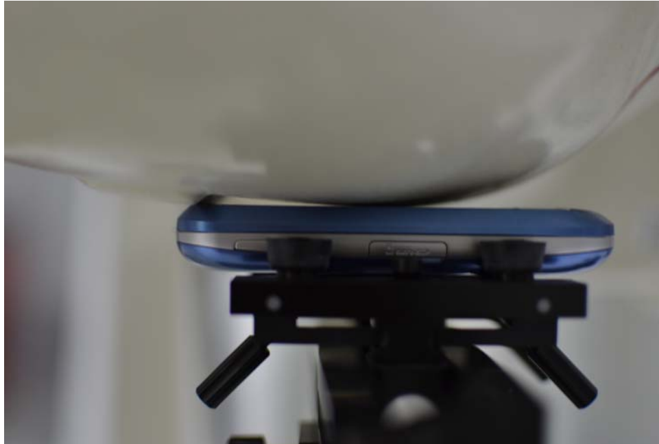
SAR Test Setup Photo 1: Right Cheek
