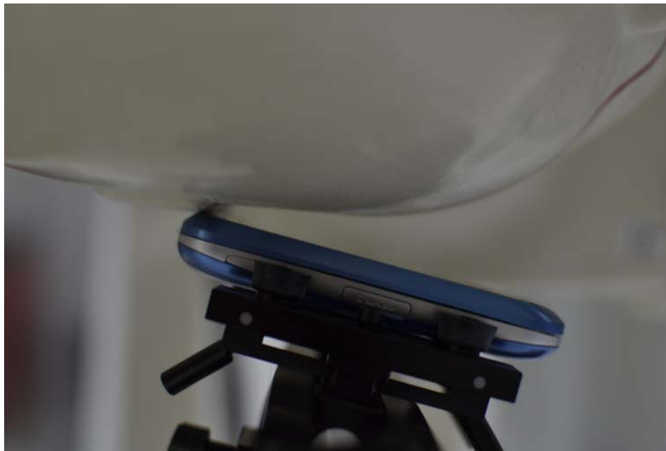
SAR Test Setup Photo 2: Right Tilt
