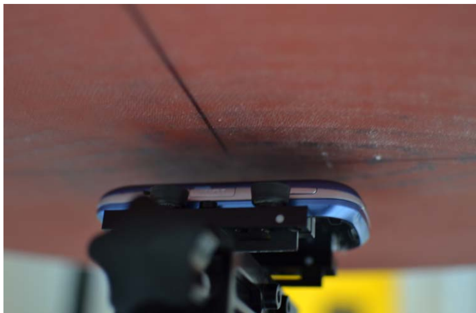
SAR Test Setup Photo 5: Back side at 1.5 cm
