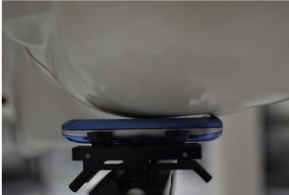
SAR Test Setup Photo 3: Left Cheek
