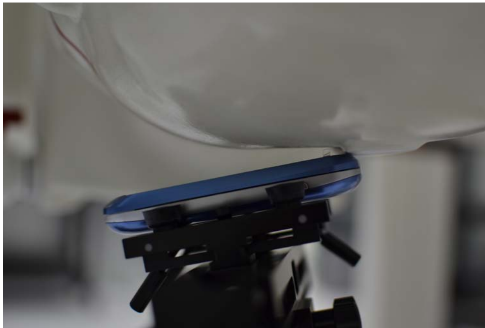
SAR Test Setup Photo 4: Left Tilt
