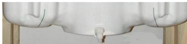
Figure 7-2 SAM Twin Phantom Shell
