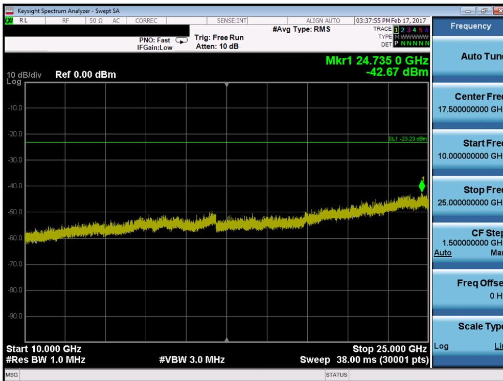
Plot 7-13. Conducted Spurious Plot (Bluetooth (LE) – Ch. 0)
