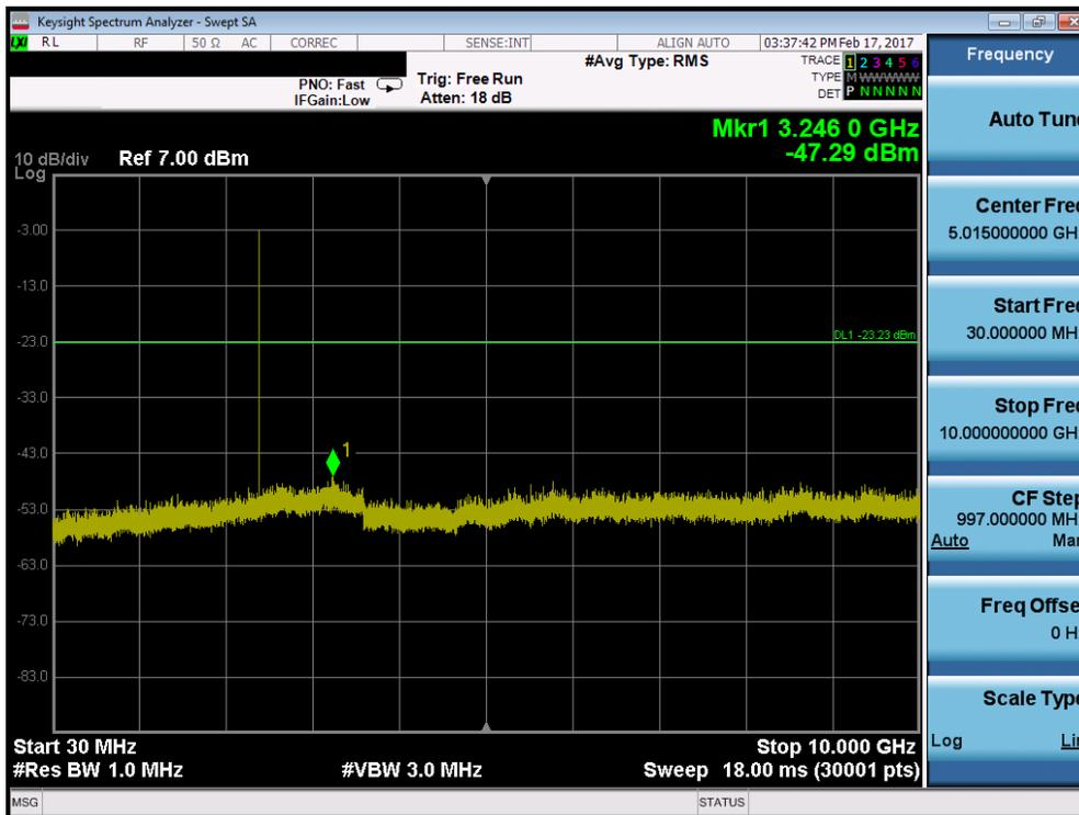
Plot 7-12. Conducted Spurious Plot (Bluetooth (LE) – Ch. 0)
