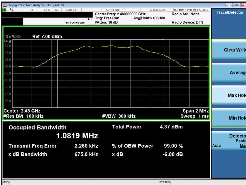
Plot 7-3. 6dB Bandwidth Plot (Bluetooth (LE) – Ch. 39)
