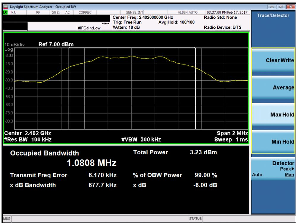
**Plot 7-1. 6dB Bandwidth Plot (Bluetooth (LE) – Ch. 0)**
