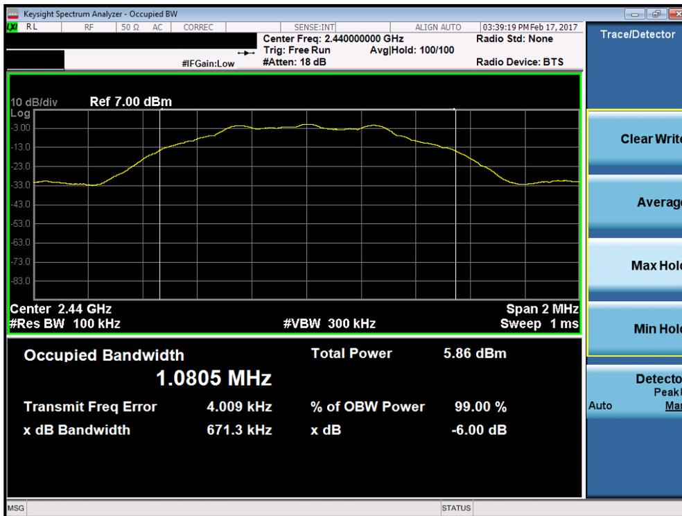
Plot 7-2. 6dB Bandwidth Plot (Bluetooth (LE) – Ch. 19)
