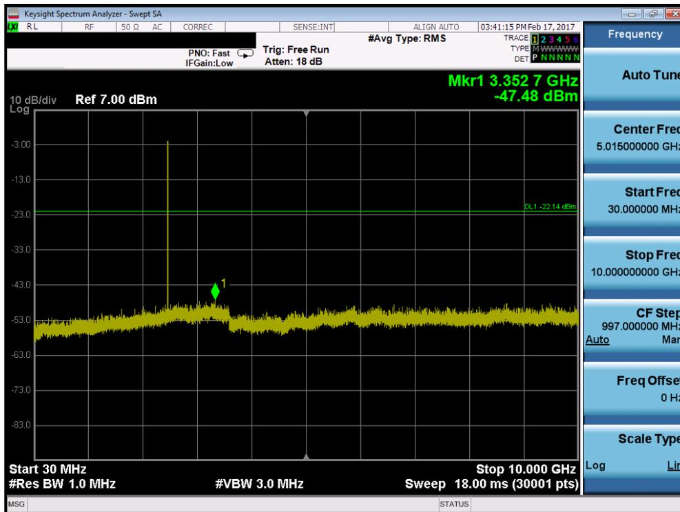
Plot 7-16. Conducted Spurious Plot (Bluetooth (LE) – Ch. 39)
