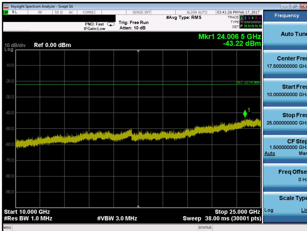
Plot 7-17. Conducted Spurious Plot (Bluetooth (LE) – Ch. 39)
