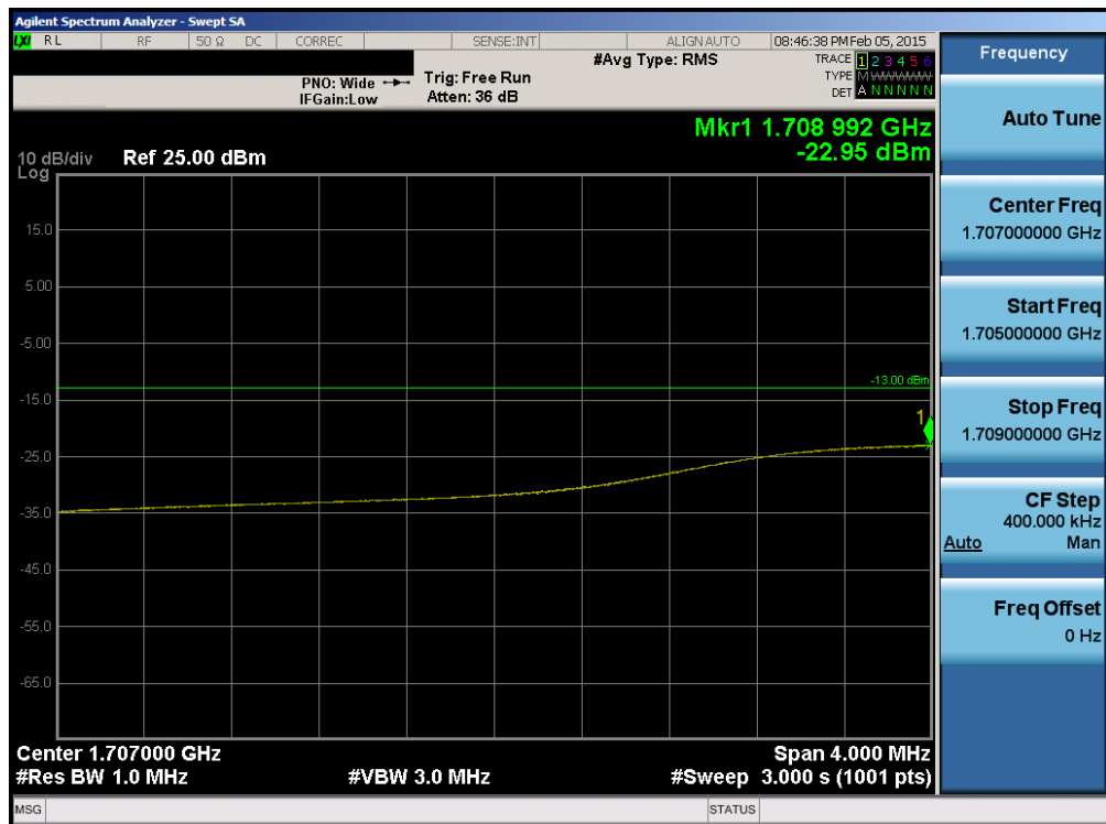
Plot 6-230. Lower Extended Band Edge Plot (Band 4 – 10.0MHz QPSK – RB Size 50)
