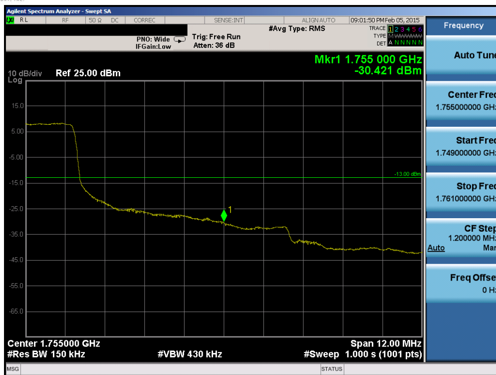
Plot 6-235. Upper Band Edge Plot (Band 4 – 15.0MHz QPSK – RB Size 75)
