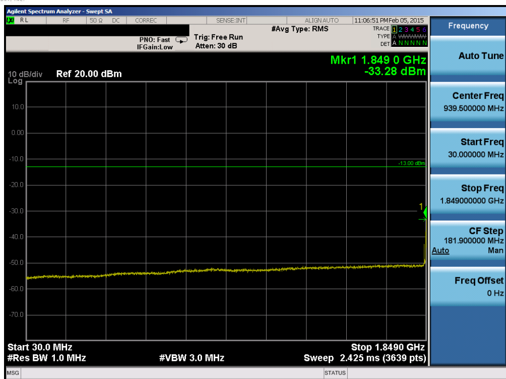
Plot 6-175. Conducted Spurious Plot (Band 2 – 15.0MHz QPSK – RB Size 1, RB Offset 0 – Low Channel)
