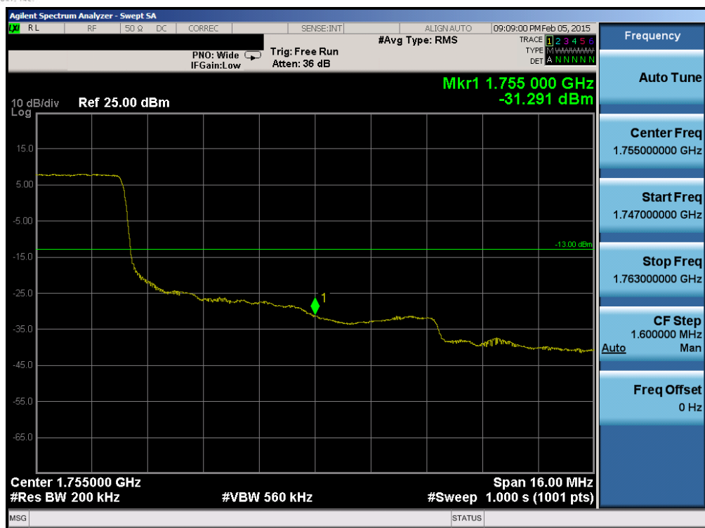
Plot 6-239. Upper Band Edge Plot (Band 4 – 20.0MHz QPSK – RB Size 100)
