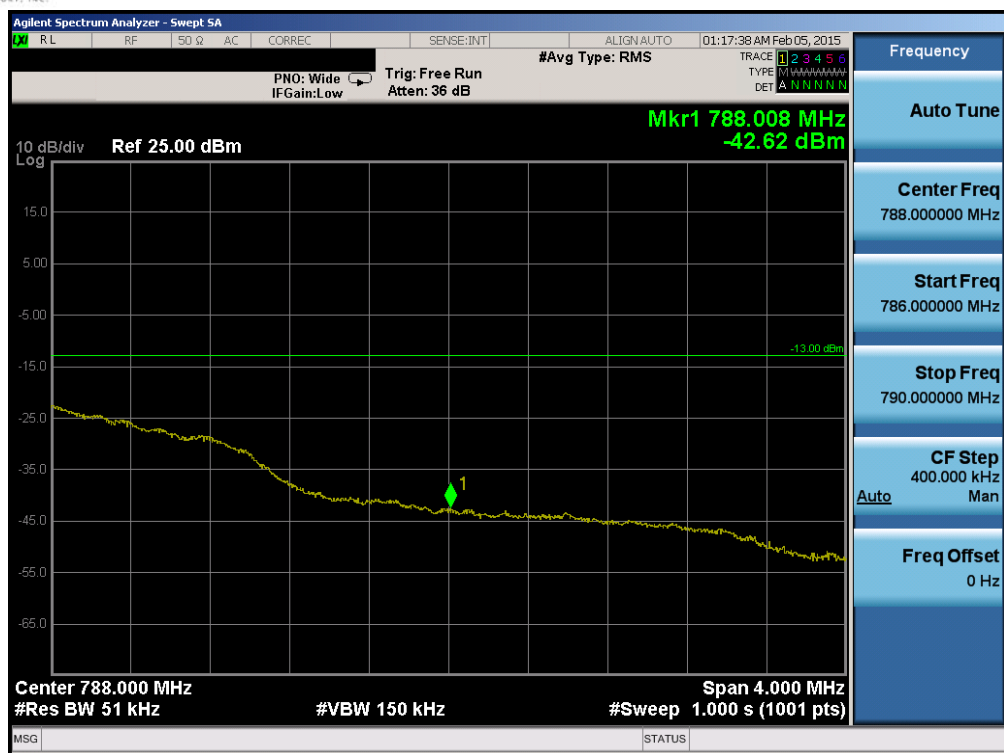
Plot 6-195. Upper Band Edge Plot (Band 13 – 5.0MHz QPSK – RB Size 25)
