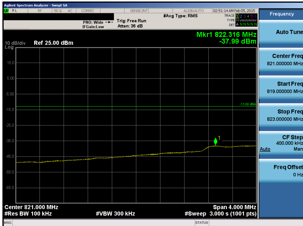
Plot 6-214. Lower Extended Band Edge Plot (Band 5 – 10.0MHz QPSK – RB Size 50)
