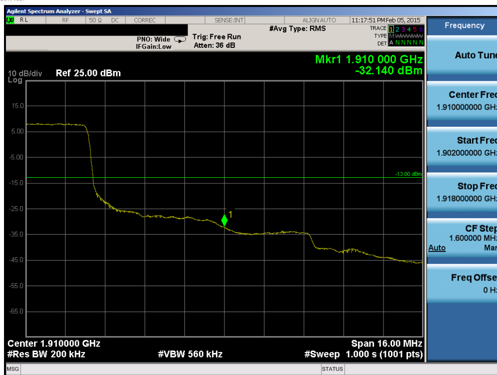
Plot 6-263. Upper Band Edge Plot (Band 2 – 20.0MHz QPSK – RB Size 100)
