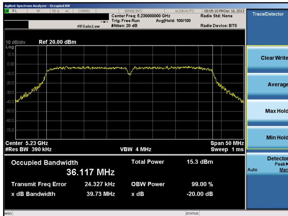
Plot 6-28. 20dB Bandwidth Plot (40MHz BW 802.11n (UNII Band 2A) – Ch. 46)
