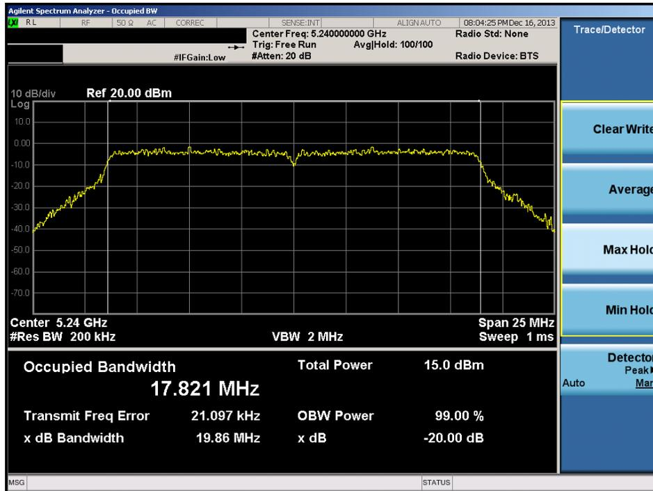
Plot 6-27. 20dB Bandwidth Plot (20MHz BW 802.11n (UNII Band 2A) – Ch. 48)
