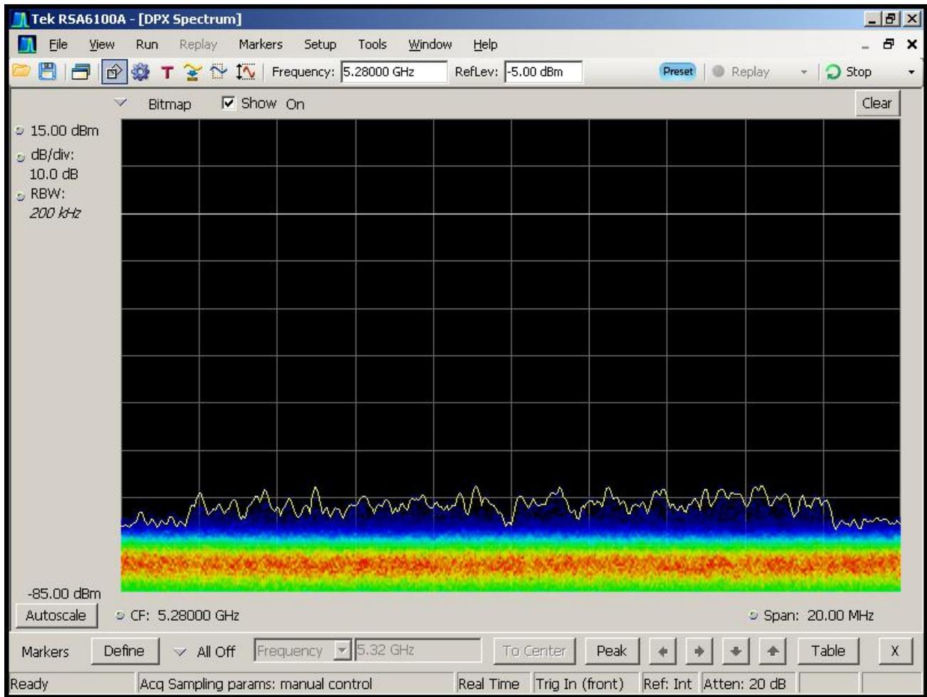
**Figure 5-2. Real-Time Spectrum Display, No WLAN Traffic**
