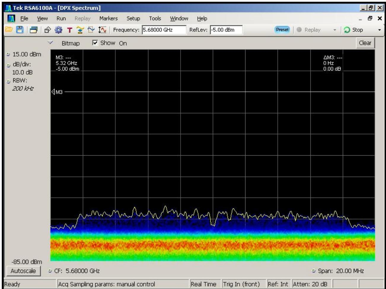
**Figure 6-2. Real-Time Spectrum Display, No WLAN Traffic**
