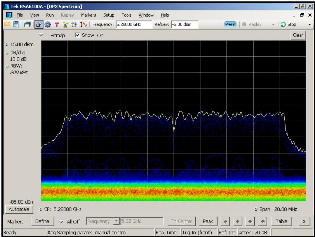
**Figure 5-3. Real-Time Spectrum Display, WLAN Traffic (Streaming Video)**
