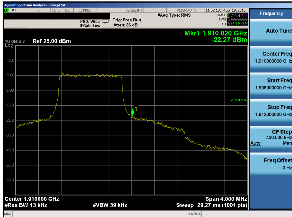
Plot 6-144. Upper Band Edge Plot (Band 2 – 1.4MHz QPSK – RB Size 6)
