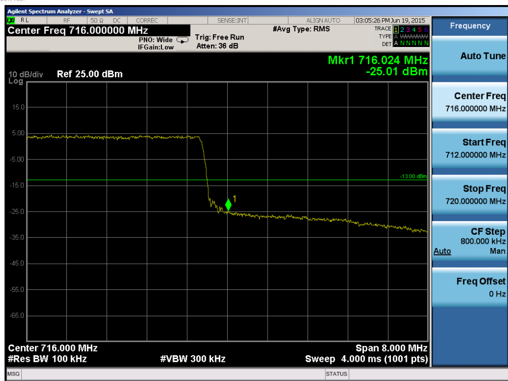
Plot 6-103. Upper Band Edge Plot (Band 12 – 10.0MHz QPSK – RB Size 50)
