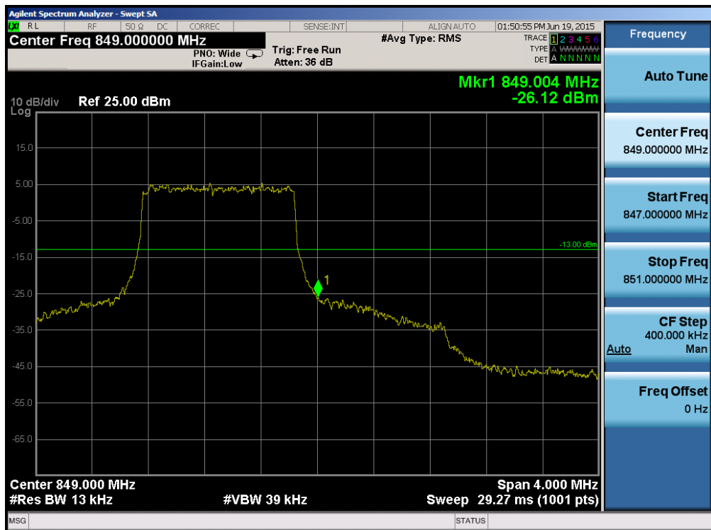
Plot 6-106. Upper Band Edge Plot (Band 5 – 1.4MHz QPSK – RB Size 6)
