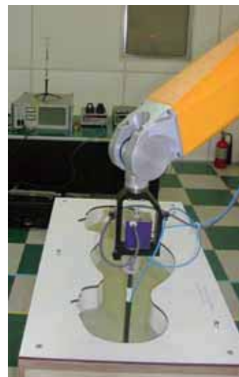
Figure 3. Photograph of the probe and the Phantom
