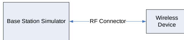
Figure 9-4 Power Measurement Setup
