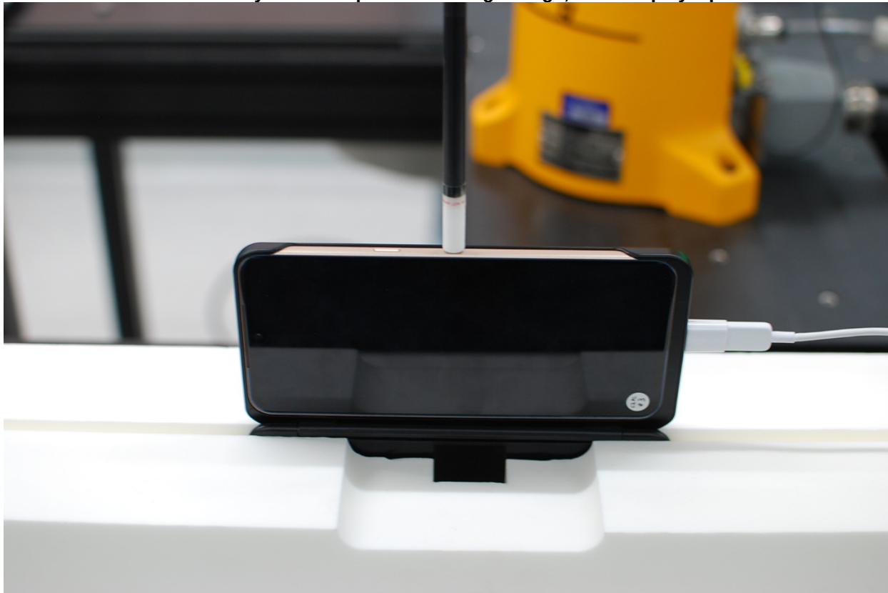
Near-Field Power Density Test Setup Photo 7 – Right Edge, Dual Display Open 180 at 2 mm
