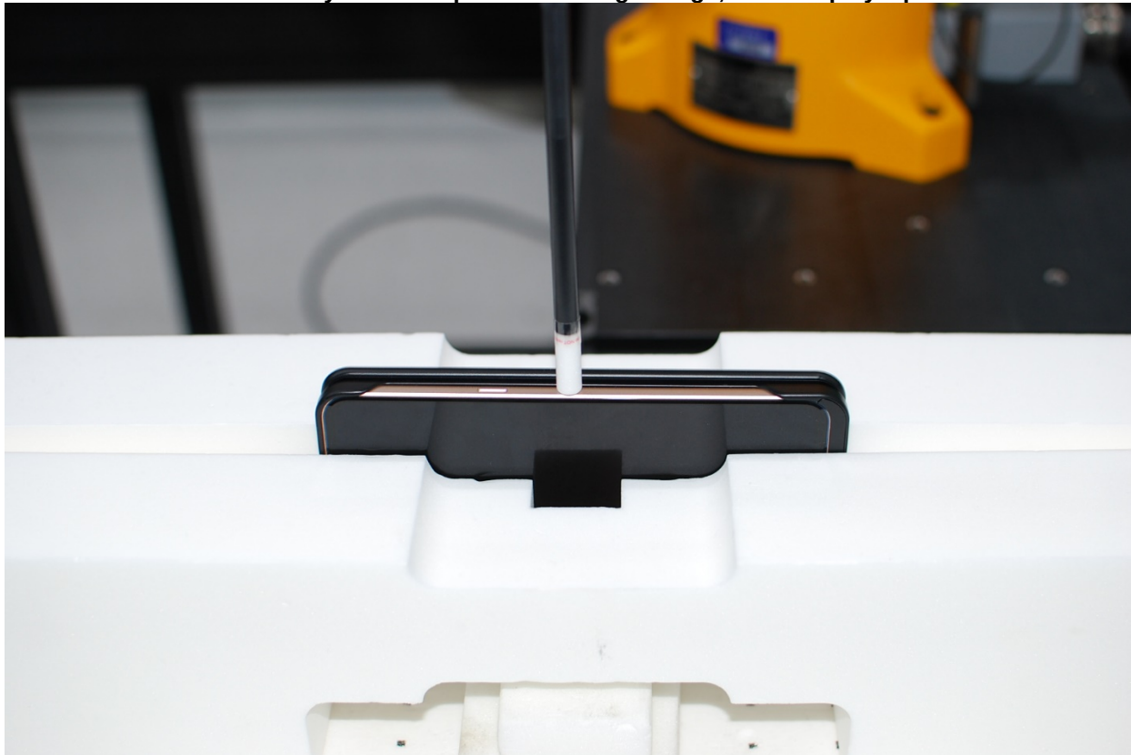
Near-Field Power Density Test Setup Photo 8 – Right Edge, Dual Display Open 360 at 2 mm
