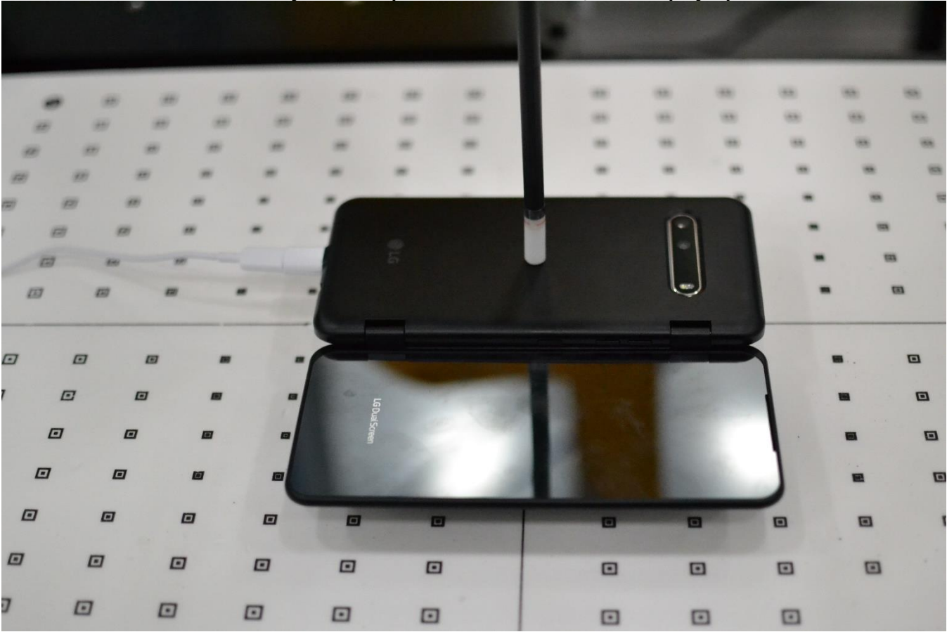
Near-Field Power Density Test Setup Photo 7 - Back Side, Dual Display Open 180 at 2 mm
