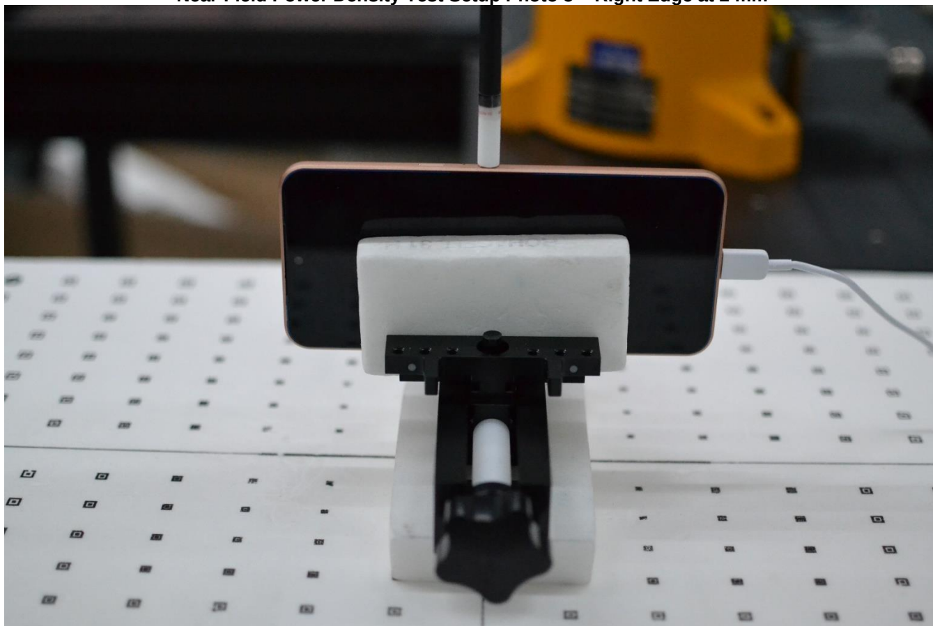
Near-Field Power Density Test Setup Photo 5 – Right Edge at 2 mm
