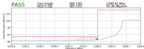
Plot 7-31. Radiated Restricted Lower Band Edge Measurement MIMO (Average)
