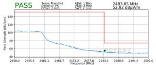
Plot 7-26. Radiated Restricted Upper Band Edge Measurement SISO ANT2 (Peak)
