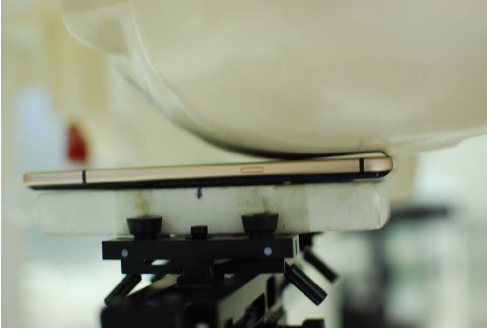
SAR Test Setup Photo 3 – Left Cheek
