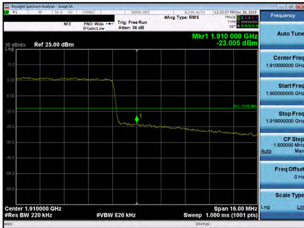
Plot 7-407. Upper Band Edge Plot (5G NR n2 - 20.0MHz QPSK - DFT-s - Full RB Configuration)
