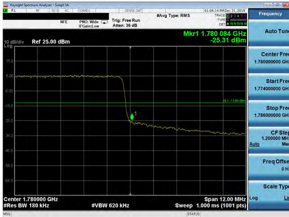
Plot 7-369. Upper Band Edge Plot (5G NR n66 - 15.0MHz QPSK - CP - Full RB Configuration)
