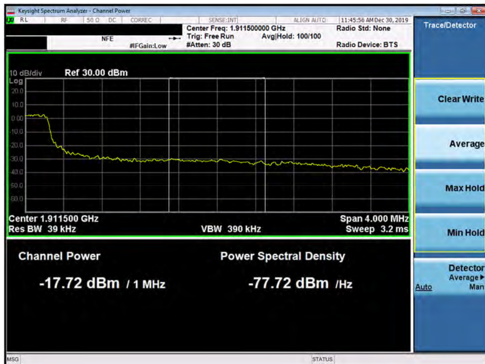
Plot 7-386. Upper Extended Band Edge Plot (5G NR n2 - 5.0MHz QPSK - CP - Full RB Configuration)
