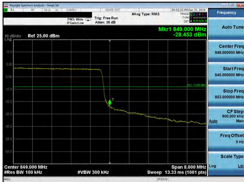
Plot 7-338. Upper Band Edge Plot (5G NR n5 - 10.0MHz QPSK - CP - Full RB Configuration)
