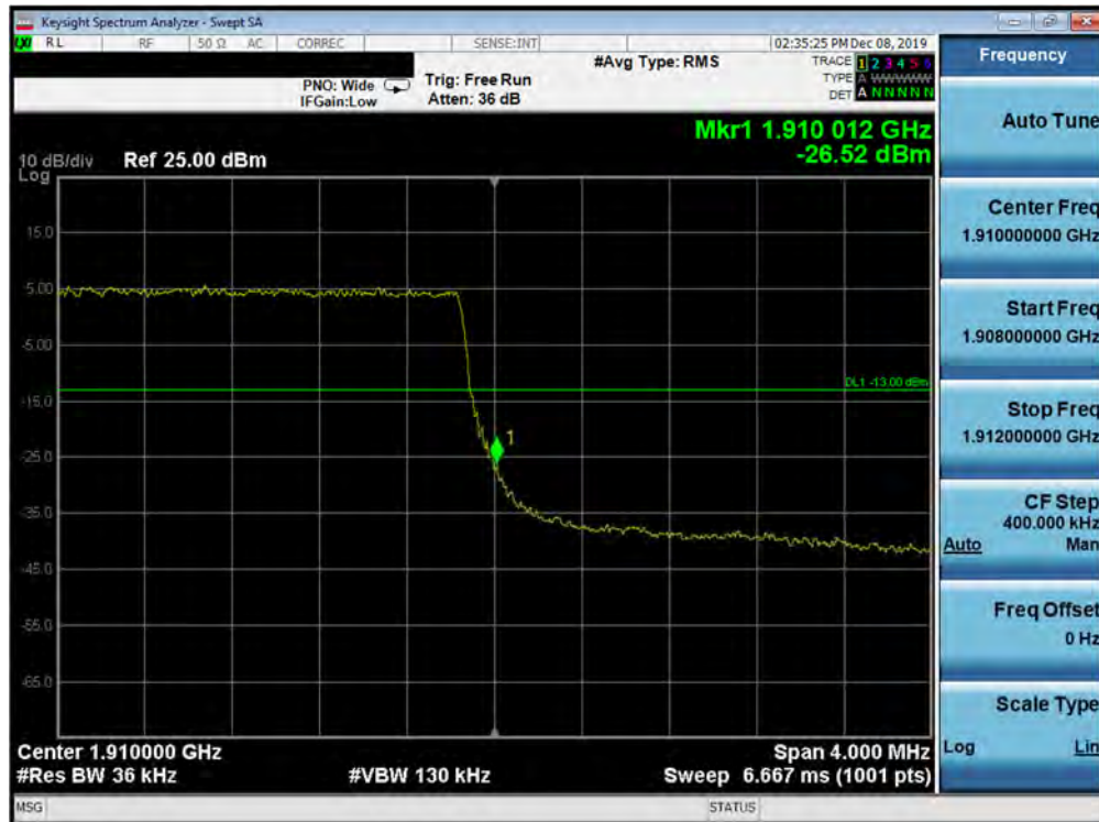
Plot 7-296. Upper Band Edge Plot (Band 2 - 3.0MHz QPSK - Full RB Configuration)
