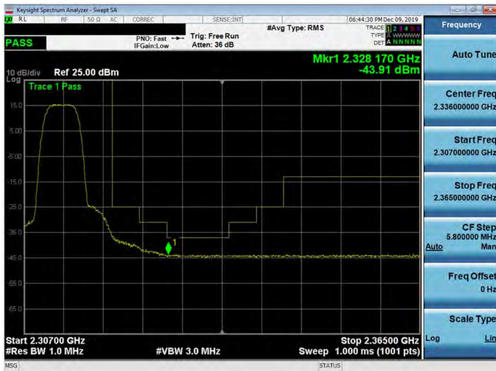
Plot 7-316. Upper Extended Band Edge Plot (Band 30 - 5.0MHz QPSK - Full RB Configuration)
