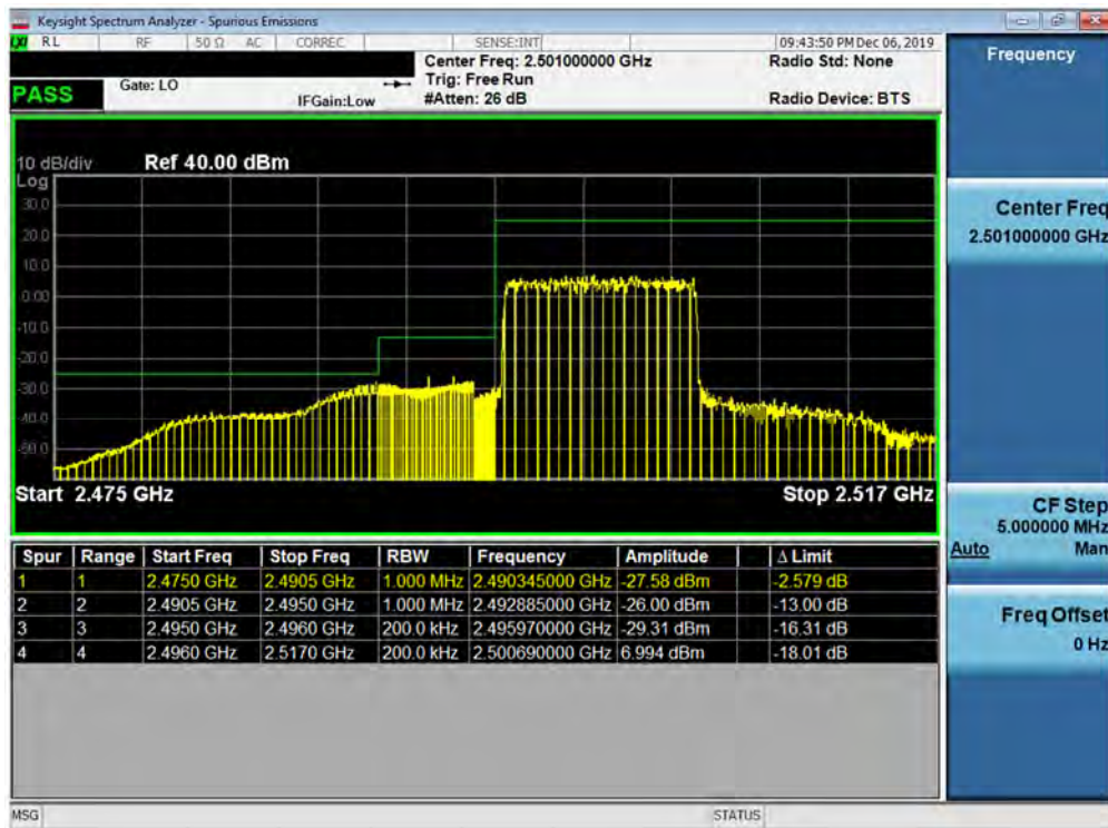
Plot 7-325. Lower ACP Plot at 2496 MHz (Band 41 - 10.0MHz QPSK - Full RB Configuration)
