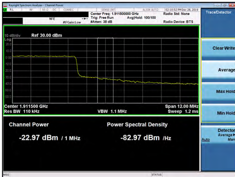
Plot 7-402. Upper Extended Band Edge Plot (5G NR n2 - 15.0MHz QPSK - CP - Full RB Configuration)
