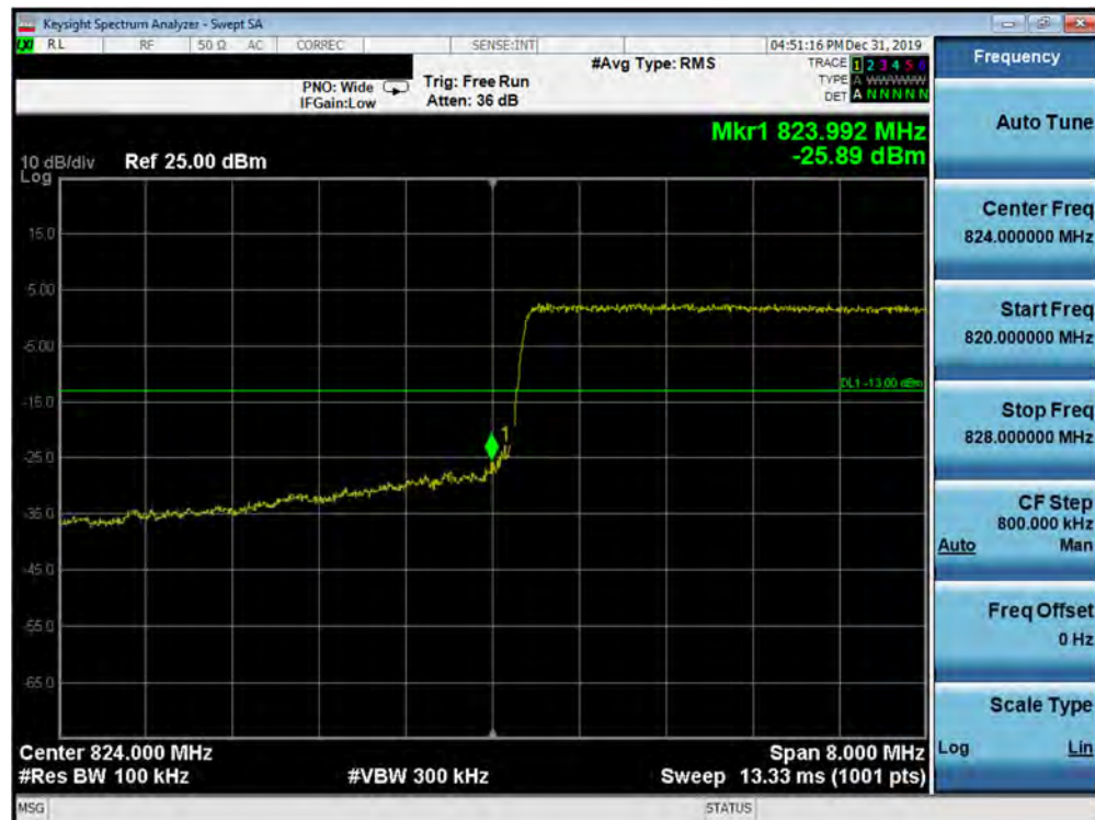
Plot 7-336. Lower Band Edge Plot (5G NR n5 - 10.0MHz QPSK - CP - Full RB Configuration)
