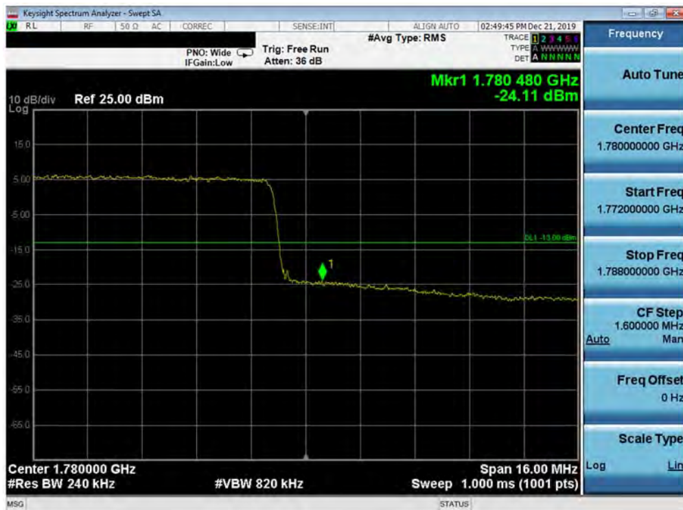
Plot 7-288. Upper Band Edge Plot (Band 66 - 20.0MHz QPSK - Full RB Configuration)
