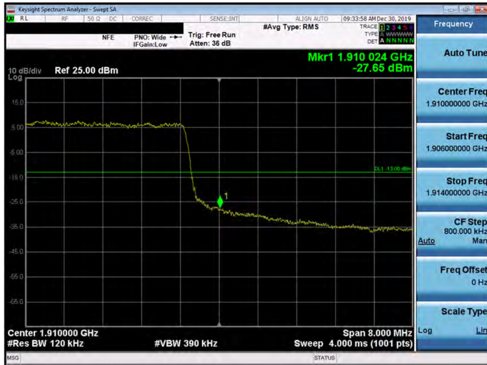
Plot 7-391. Upper Band Edge Plot (5G NR n2 - 10.0MHz QPSK - DFT-s - Full RB Configuration)
