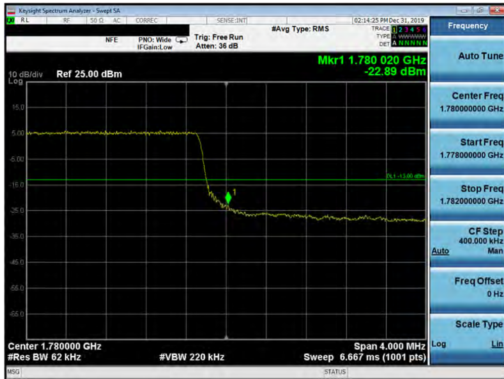
Plot 7-353. Upper Band Edge Plot (5G NR n66 - 5.0MHz QPSK - CP - Full RB Configuration)
