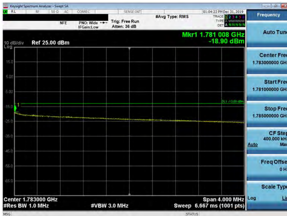
Plot 7-370. Upper Extended Band Edge Plot (5G NR n66 - 15.0MHz QPSK - CP - Full RB Configuration)
