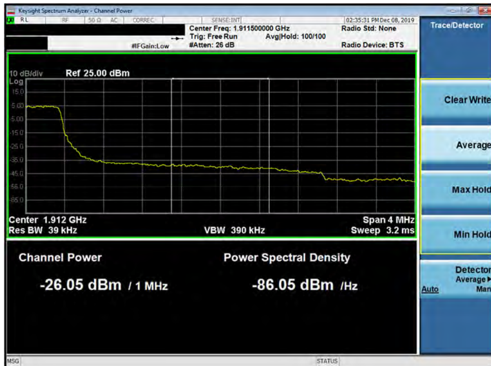
Plot 7-297. Upper Extended Band Edge Plot (Band 2 - 3.0MHz QPSK - Full RB Configuration)
