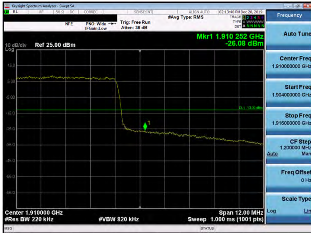
Plot 7-399. Upper Band Edge Plot (5G NR n2 - 15.0MHz QPSK - DFT-s - Full RB Configuration)
