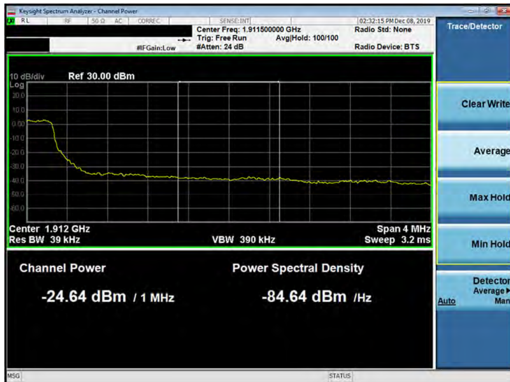
Plot 7-301. Upper Extended Band Edge Plot (Band 2 - 5.0MHz QPSK - Full RB Configuration)
