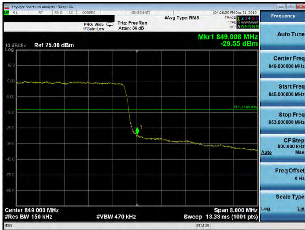
Plot 7-341. Upper Band Edge Plot (5G NR n5 - 15.0MHz QPSK - DFT-s - Full RB Configuration)
