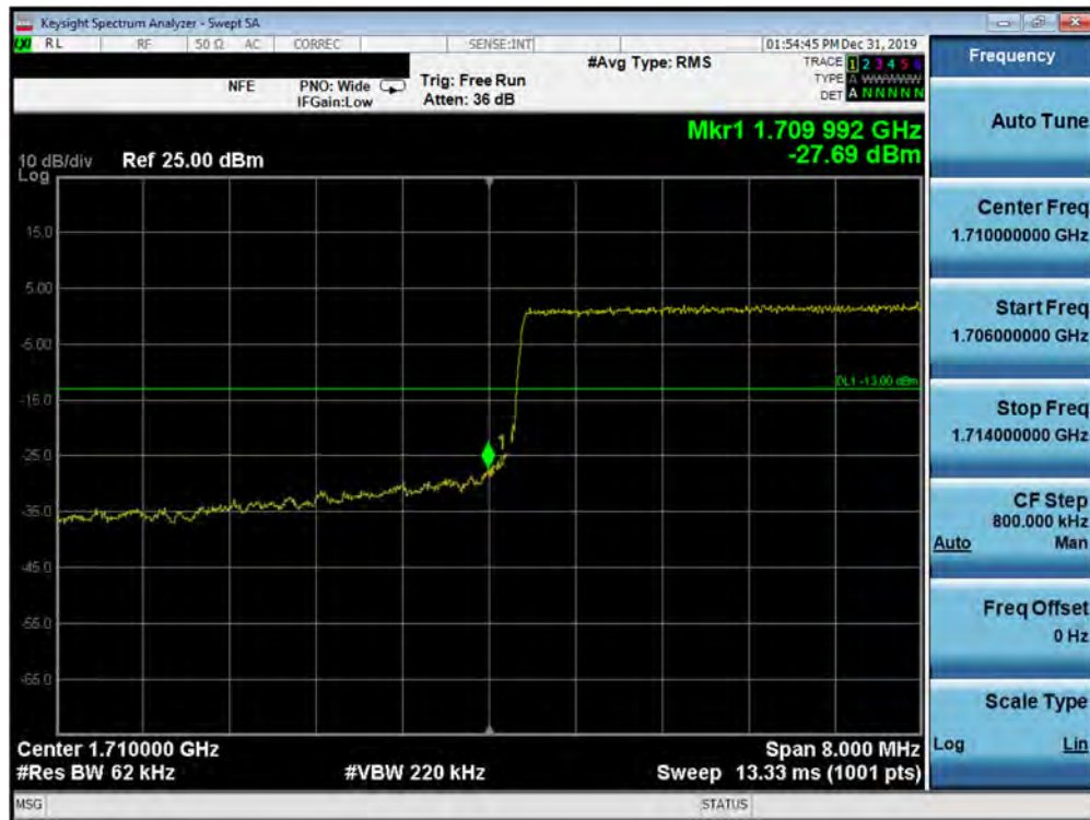
Plot 7-357. Lower Band Edge Plot (5G NR n66 - 10.0MHz QPSK - CP - Full RB Configuration)
