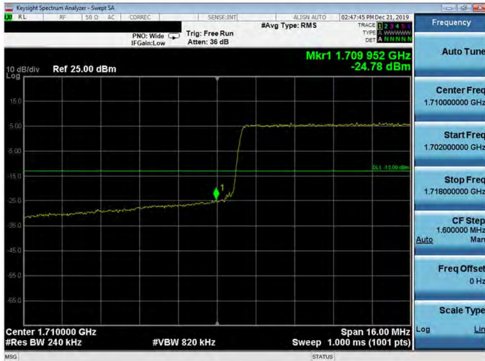
Plot 7-284. Lower Band Edge Plot (Band 66/4 - 20.0MHz QPSK - Full RB Configuration)
