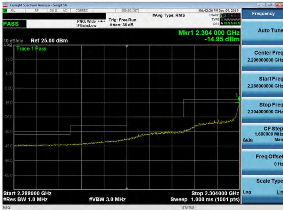
Plot 7-315. Lower Extended Band Edge Plot (Band 30 - 5.0MHz QPSK - Full RB Configuration)
