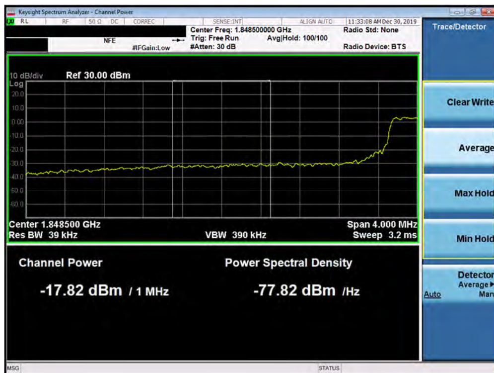
Plot 7-382. Lower Extended Band Edge Plot (5G NR n2 - 5.0MHz QPSK - CP - Full RB Configuration)
