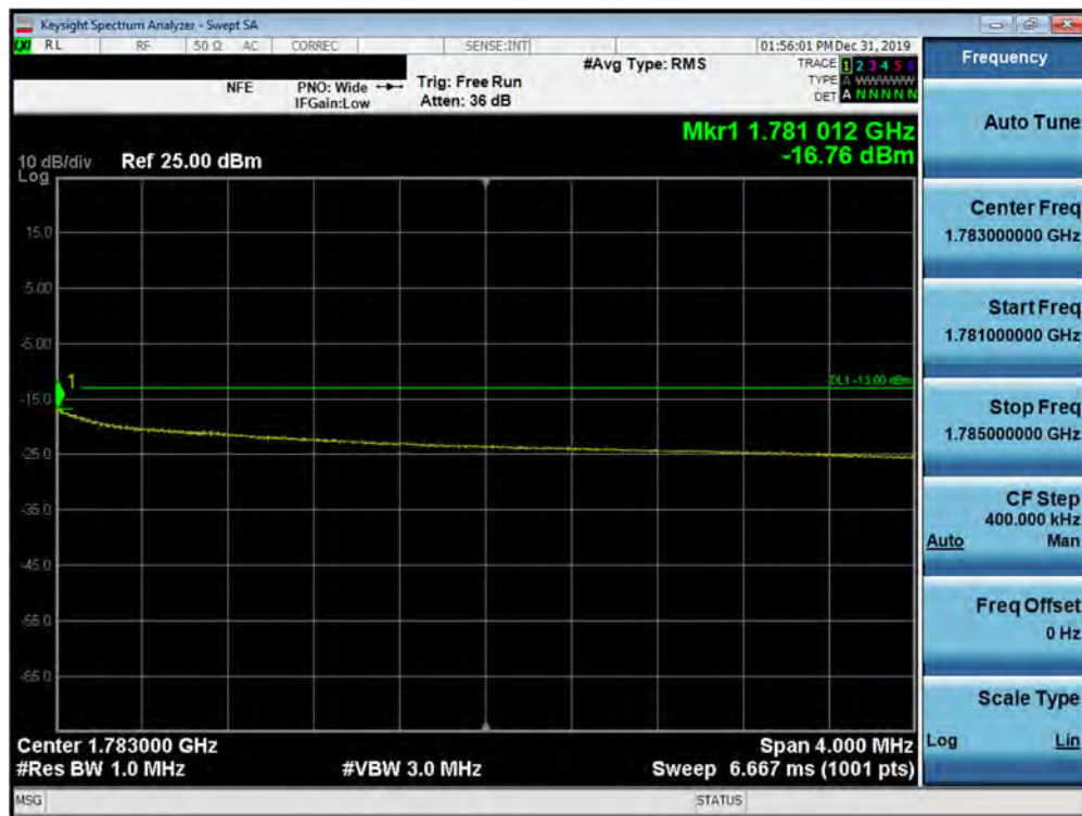
Plot 7-362. Upper Extended Band Edge Plot (5G NR n66 - 10.0MHz QPSK - CP - Full RB Configuration)
