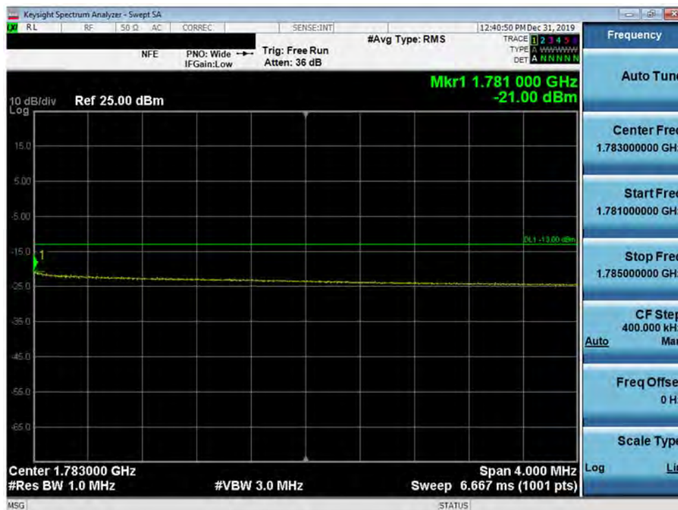
Plot 7-378. Upper Extended Band Edge Plot (5G NR n66 - 20.0MHz QPSK - CP - Full RB Configuration)
