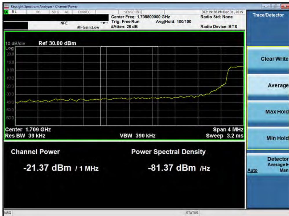
Plot 7-348. Lower Extended Band Edge Plot (5G NR n66 - 5.0MHz QPSK - DFT-s - Full RB Configuration)
