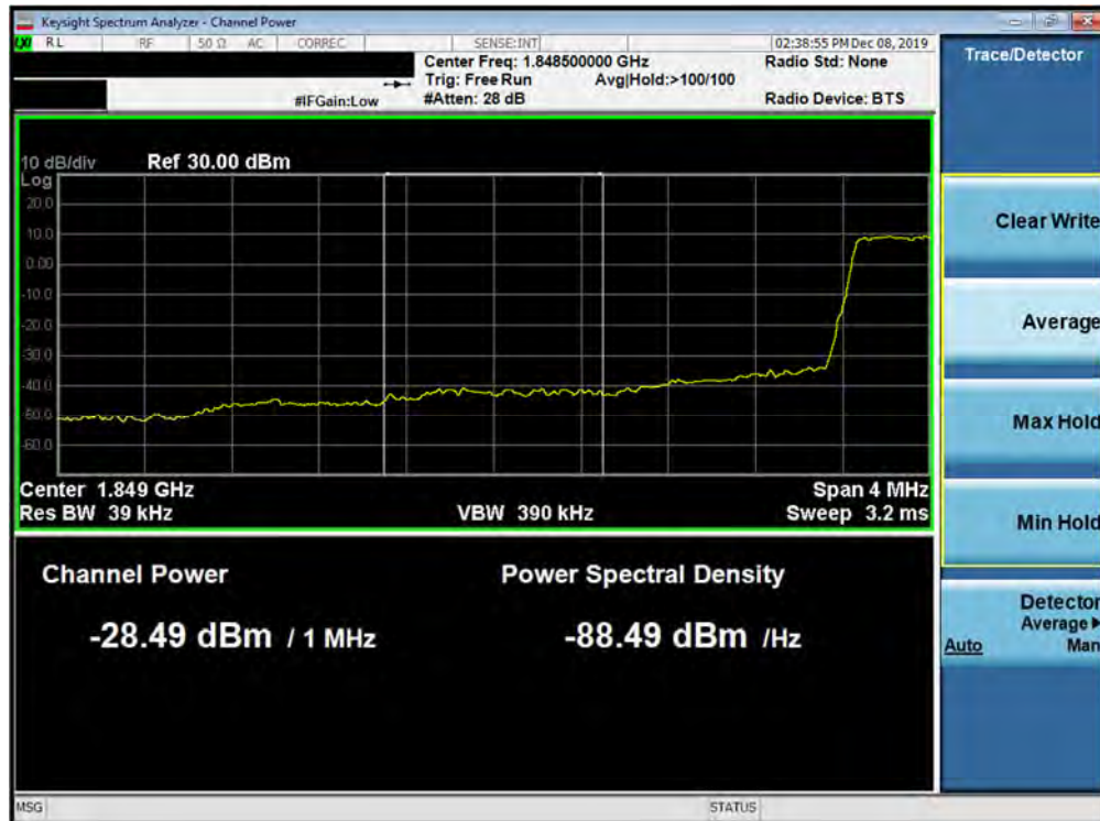
Plot 7-291. Lower Extended Band Edge Plot (Band 2 - 1.4MHz QPSK - Full RB Configuration)
