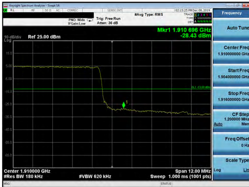
Plot 7-308. Upper Band Edge Plot (Band 2 - 15.0MHz QPSK - Full RB Configuration)
