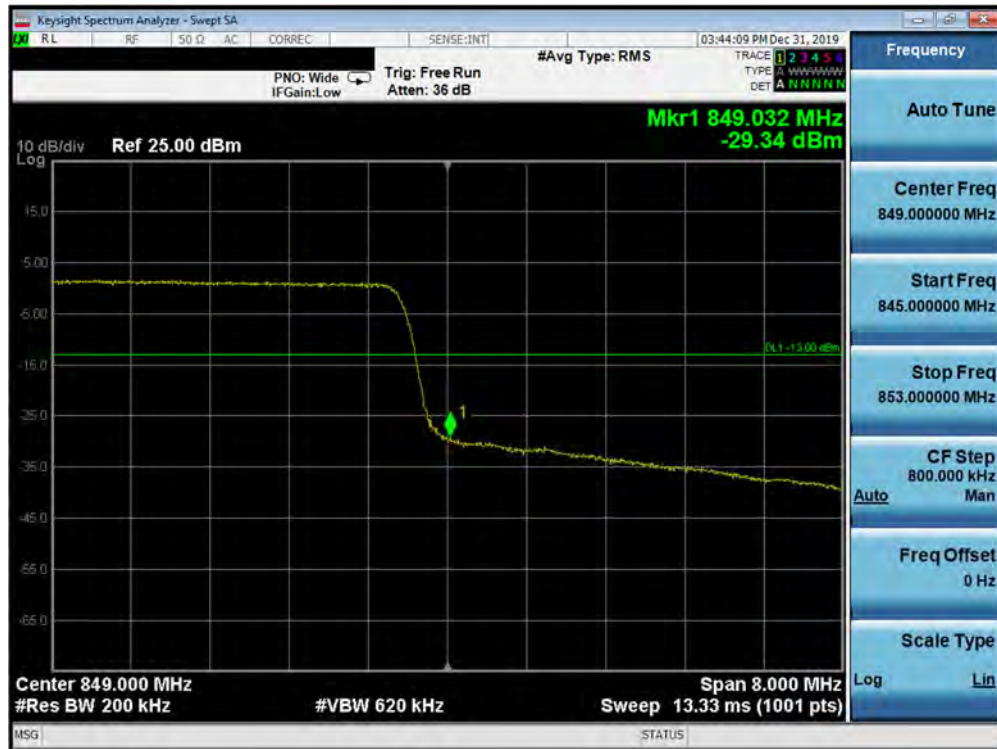
Plot 7-345. Upper Band Edge Plot (5G NR n5 - 20.0MHz QPSK - DFT-s - Full RB Configuration)
