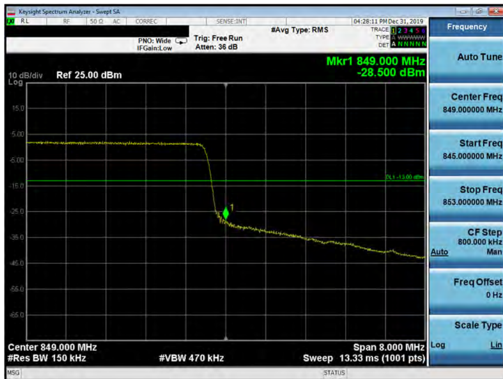
Plot 7-342. Upper Band Edge Plot (5G NR n5 - 15.0MHz QPSK - CP - Full RB Configuration)
