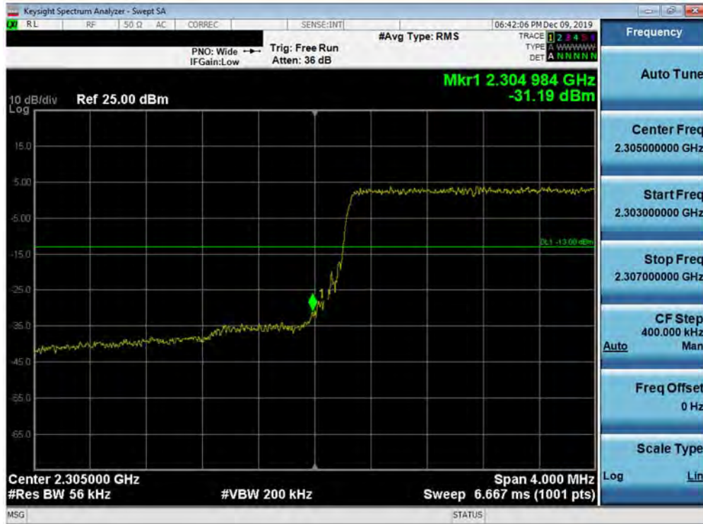
Plot 7-314. Lower Band Edge Plot (Band 30 - 5.0MHz QPSK - Full RB Configuration)
