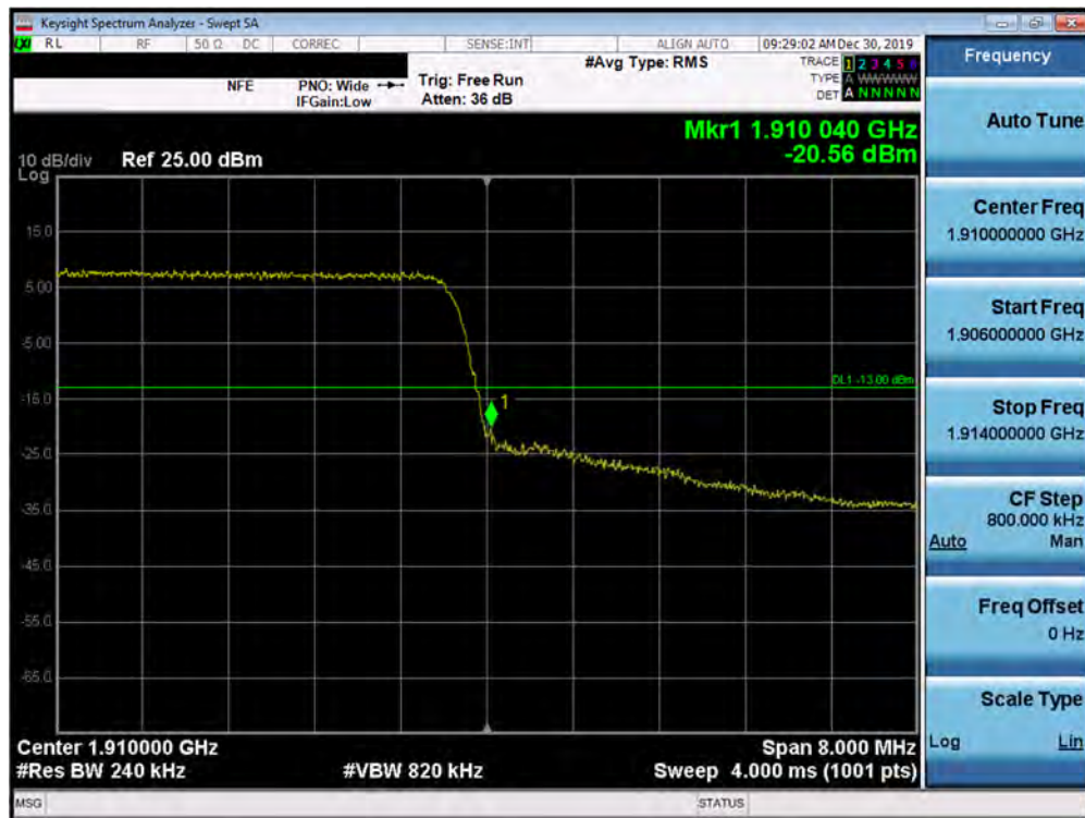
Plot 7-393. Upper Band Edge Plot (5G NR n2 - 10.0MHz QPSK - CP - Full RB Configuration)
