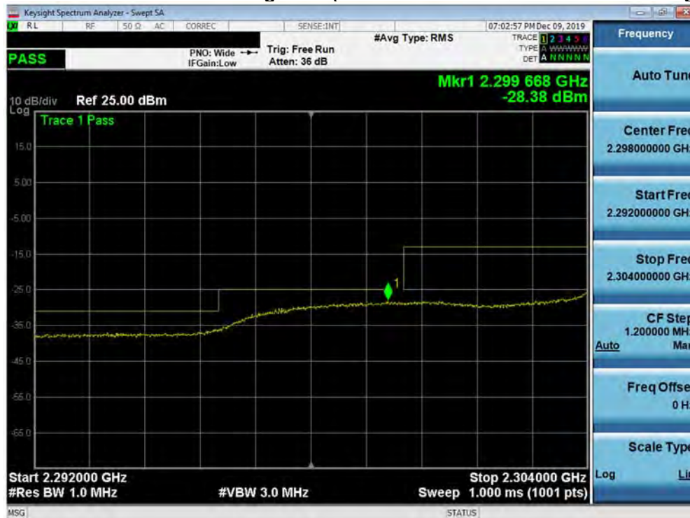
Plot 7-321. Lower Extended Band Edge Plot (Band 30 - 5.0MHz QPSK - Full RB Configuration)
