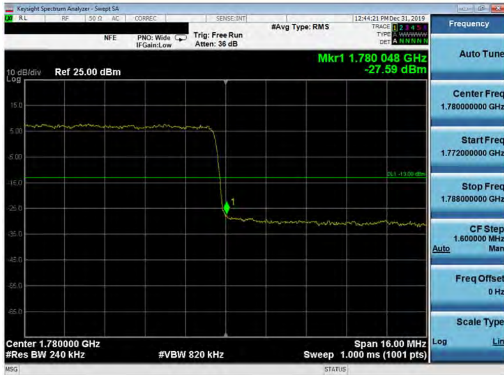
Plot 7-375. Upper Band Edge Plot (5G NR n66 - 20.0MHz QPSK - DFT-s - Full RB Configuration)
