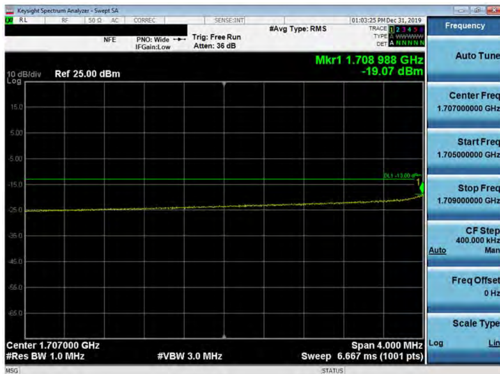
Plot 7-366. Lower Extended Band Edge Plot (5G NR n66 - 15.0MHz QPSK - CP - Full RB Configuration)
