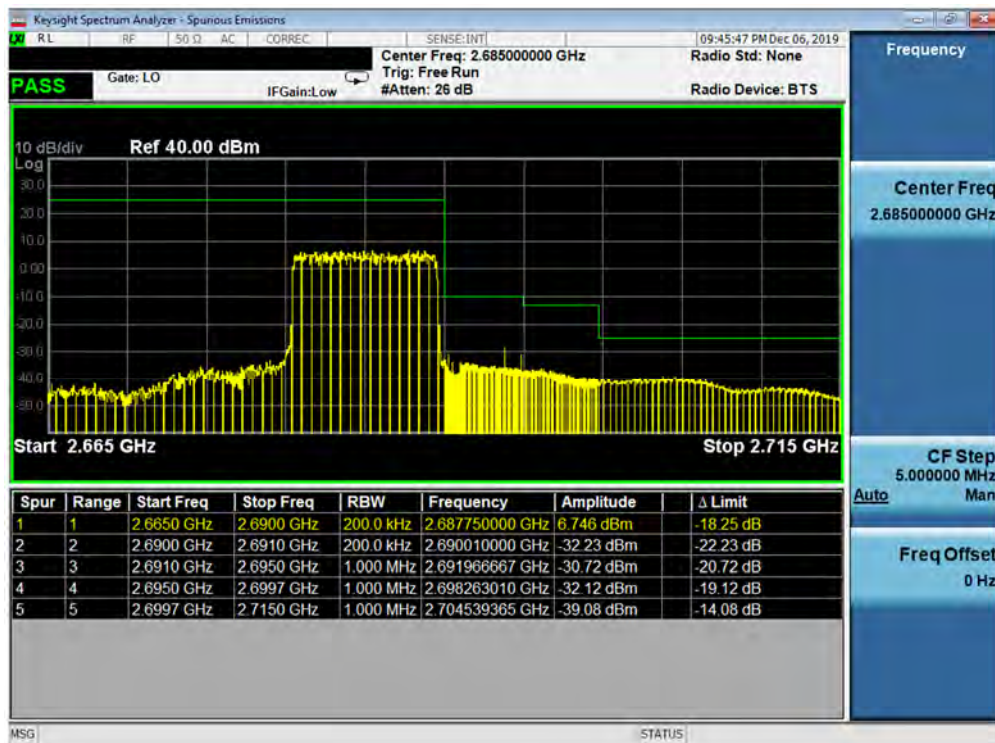
Plot 7-326. Upper ACP Plot (Band 41 - 10.0MHz QPSK - Full RB Configuration)
