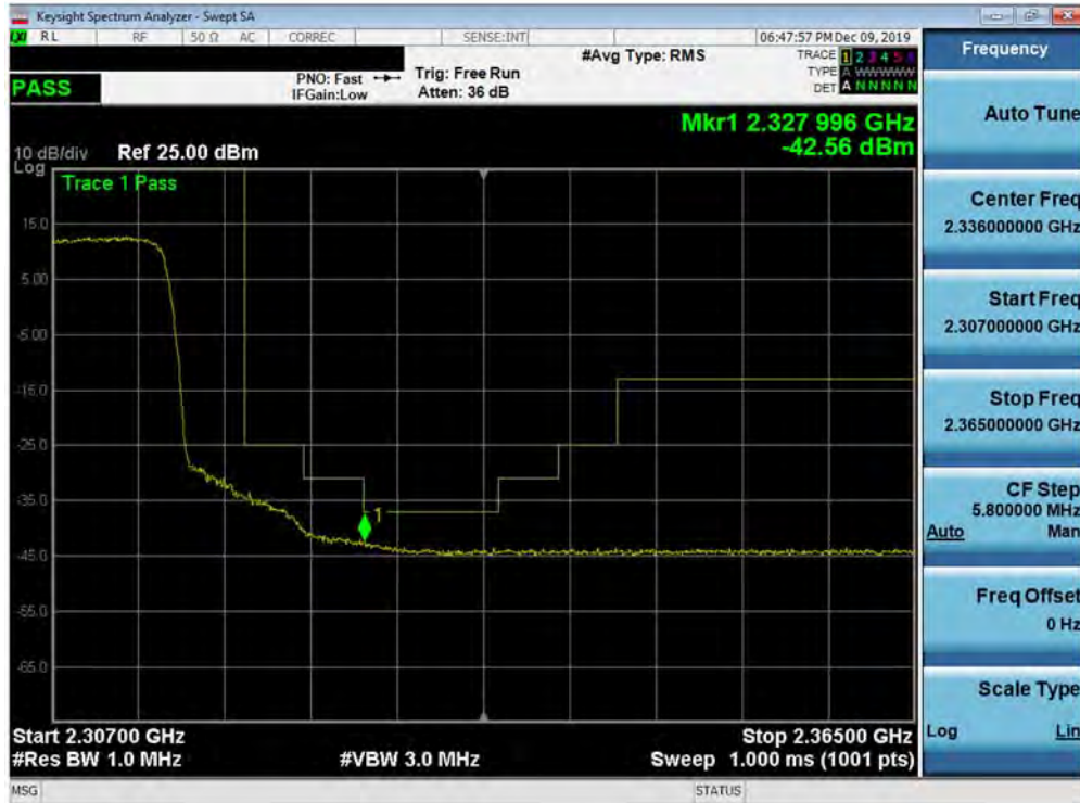
Plot 7-322. Upper Extended Band Edge Plot (Band 30 - 10.0MHz QPSK - Full RB Configuration)
