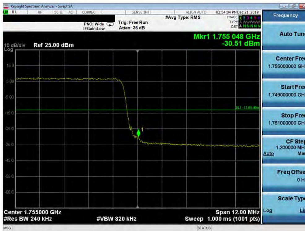
Plot 7-280. Upper Band Edge Plot (Band 4 - 15.0MHz QPSK - Full RB Configuration)
