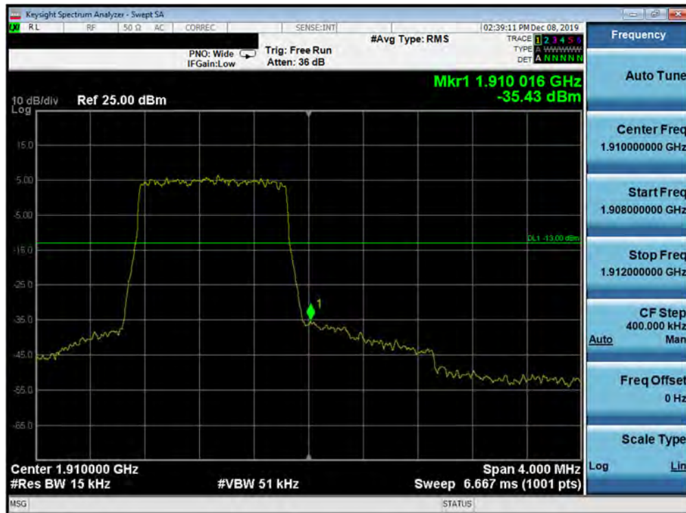
Plot 7-292. Upper Band Edge Plot (Band 2 - 1.4MHz QPSK - Full RB Configuration)
