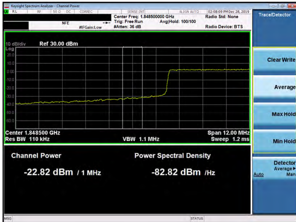
Plot 7-398. Lower Extended Band Edge Plot (5G NR n2 - 15.0MHz QPSK - CP - Full RB Configuration)
