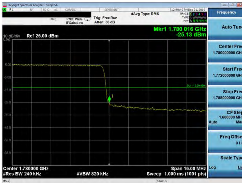
Plot 7-377. Upper Band Edge Plot (5G NR n66 - 20.0MHz QPSK - CP - Full RB Configuration)
