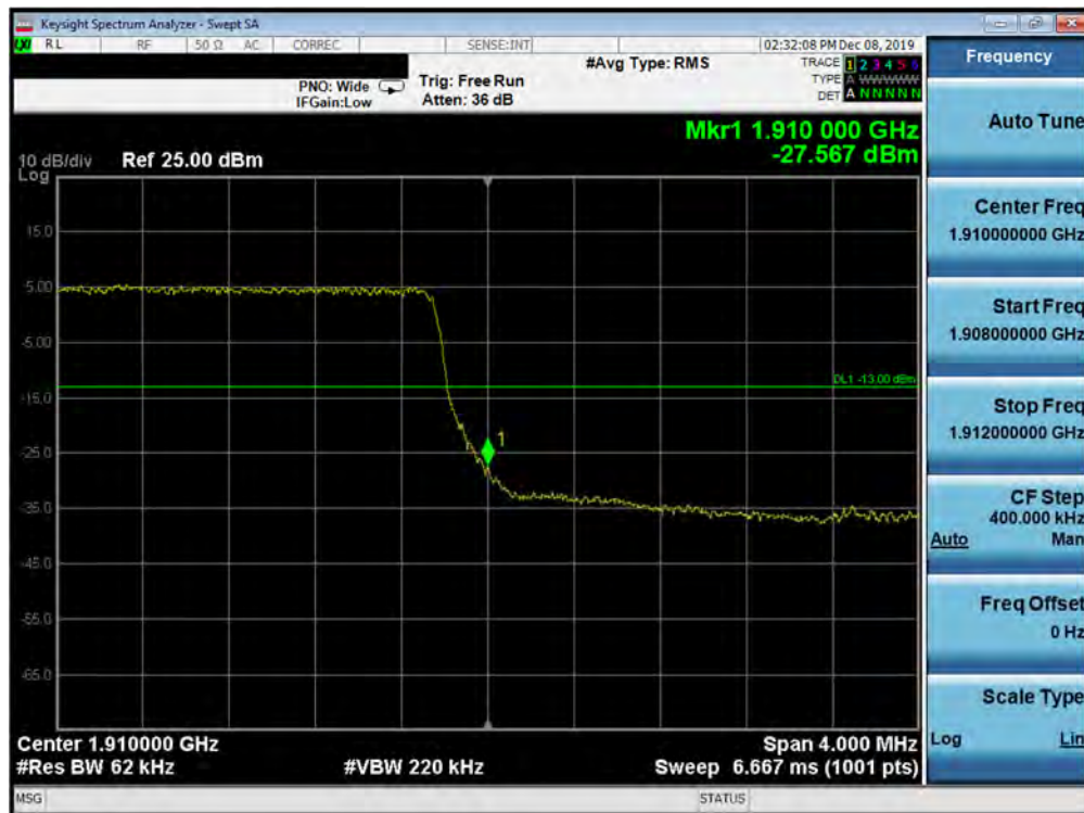
Plot 7-300. Upper Band Edge Plot (Band 2 - 5.0MHz QPSK - Full RB Configuration)
