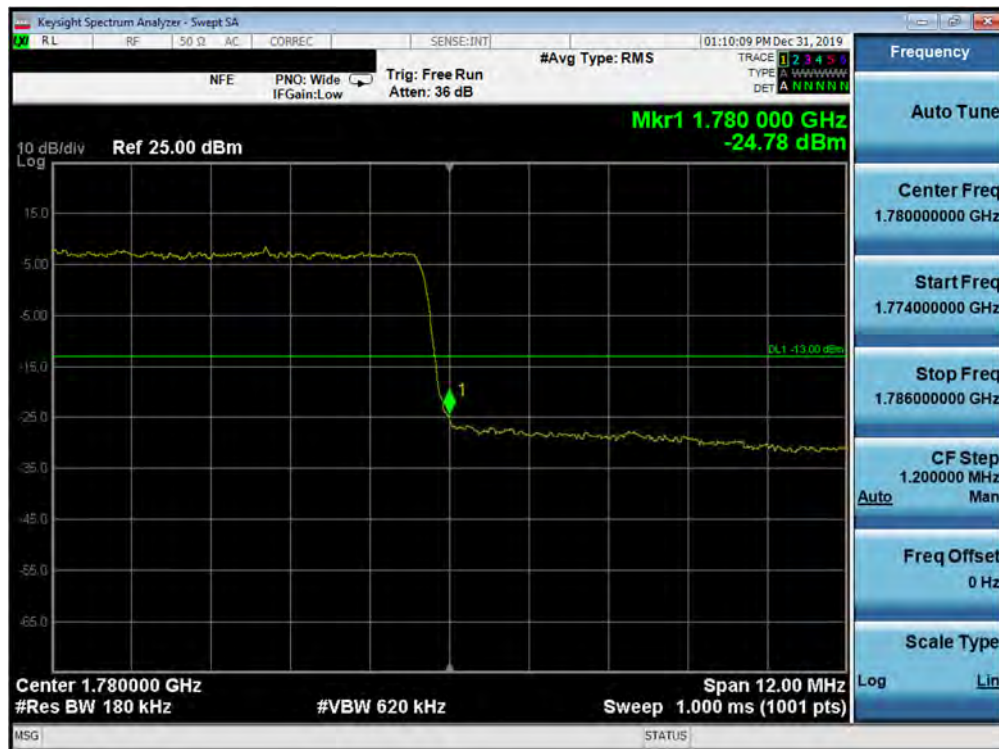
Plot 7-367. Upper Band Edge Plot (5G NR n66 - 15.0MHz QPSK - DFT-s - Full RB Configuration)
