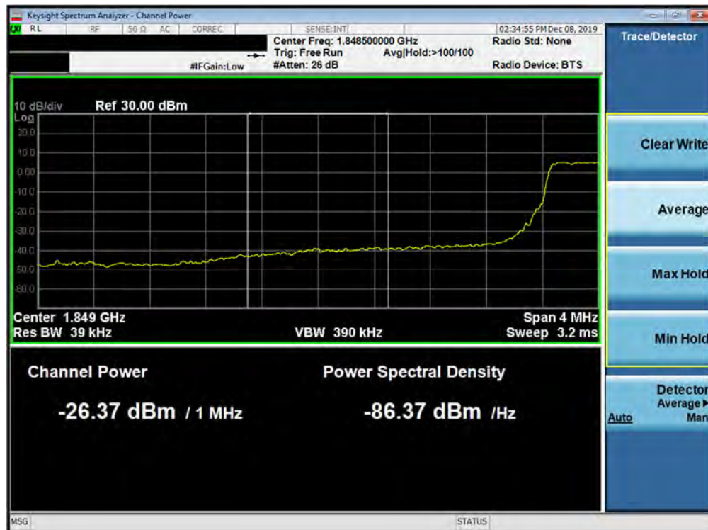
Plot 7-295. Lower Extended Band Edge Plot (Band 2 - 3.0MHz QPSK - Full RB Configuration)
