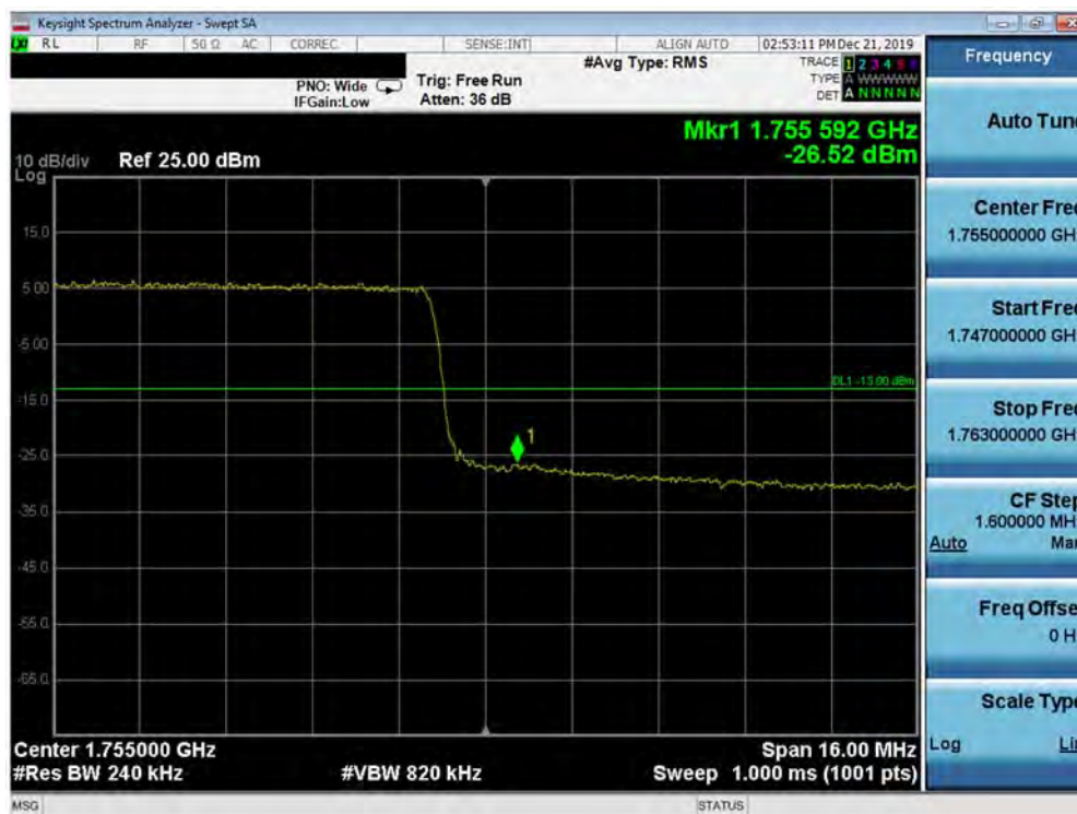
Plot 7-286. Upper Band Edge Plot (Band 4 - 20.0MHz QPSK - Full RB Configuration)
