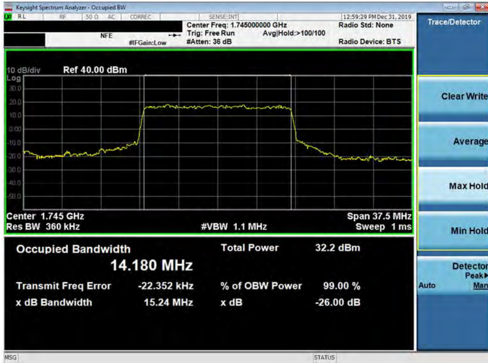
Plot 7-137. Occupied Bandwidth Plot (5G NR n66 - 15.0MHz QPSK - CP - CP - Full RB Configuration)
