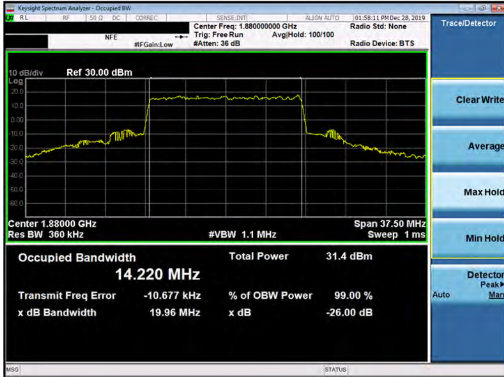
Plot 7-155. Occupied Bandwidth Plot (5G NR n2 - 15.0MHz 64-QAM - CP - Full RB Configuration)
