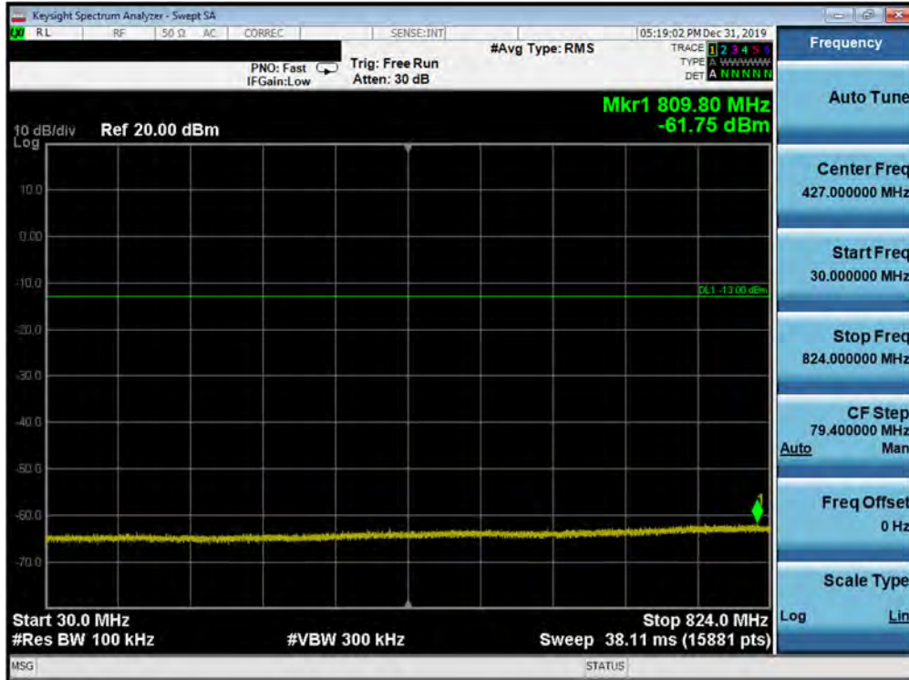
Plot 7-209. Conducted Spurious Plot (5G NR n5 - 5.0MHz QPSK - CP - CP - RB Size 1, RB Offset 0 - High Channel)
