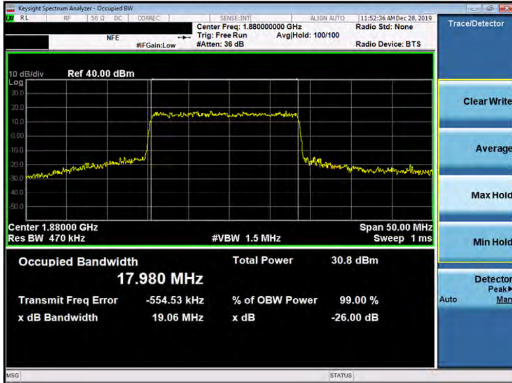
Plot 7-159. Occupied Bandwidth Plot (5G NR n2 - 20.0MHz 64-QAM - CP - Full RB Configuration)
