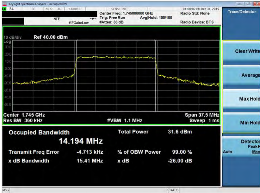
Plot 7-139. Occupied Bandwidth Plot (5G NR n66 - 15.0MHz 64-QAM - CP - Full RB Configuration)
