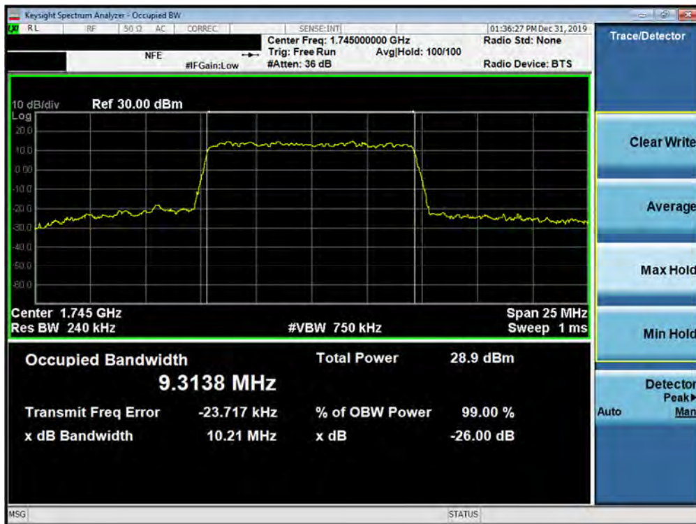
Plot 7-136. Occupied Bandwidth Plot (5G NR n66 - 10.0MHz 256-QAM - CP - Full RB Configuration)
