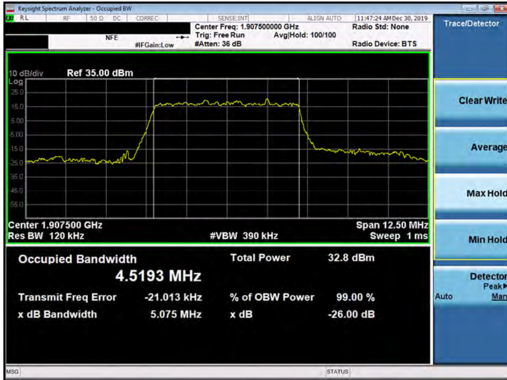
Plot 7-145. Occupied Bandwidth Plot (5G NR n2 - 5.0MHz QPSK - CP - CP - Full RB Configuration)
