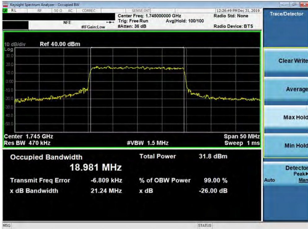
Plot 7-143. Occupied Bandwidth Plot (5G NR n66 - 20.0MHz 64-QAM - CP - Full RB Configuration)
