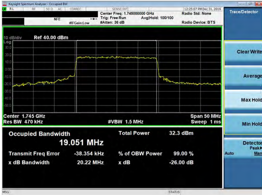
Plot 7-141. Occupied Bandwidth Plot (5G NR n66 - 20.0MHz QPSK - CP - CP - Full RB Configuration)
