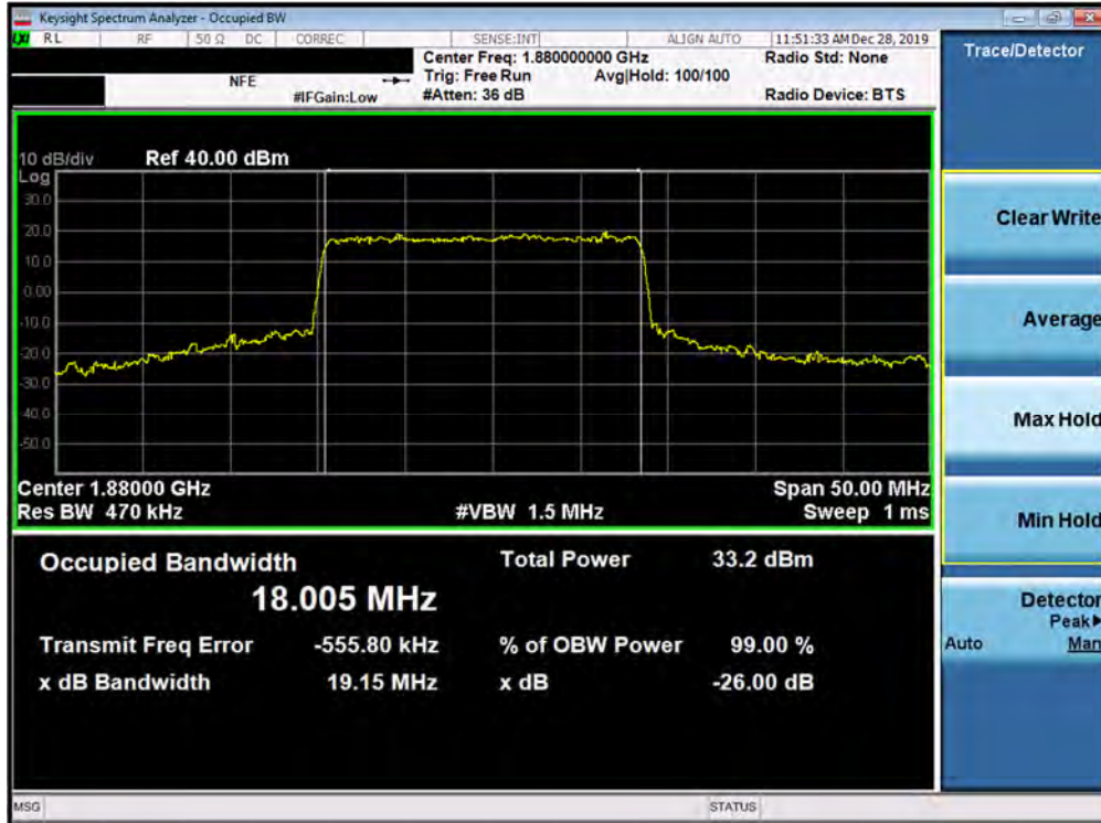
Plot 7-157. Occupied Bandwidth Plot (5G NR n2 - 20.0MHz QPSK - CP - CP - Full RB Configuration)
