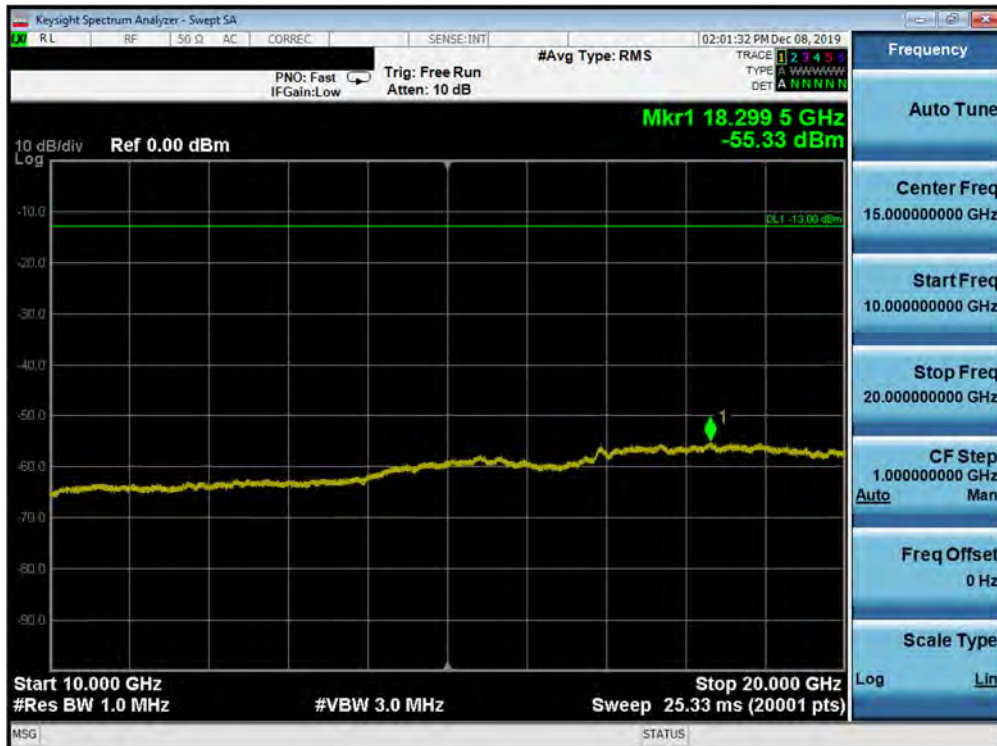
Plot 7-187. Conducted Spurious Plot (Band 2 - 10.0MHz QPSK - RB Size 1, RB Offset 0 - Mid Channel)
