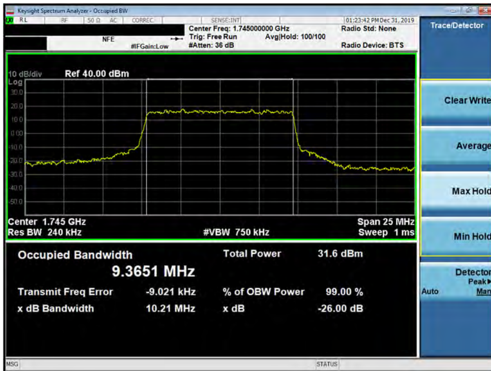
Plot 7-134. Occupied Bandwidth Plot (5G NR n66 - 10.0MHz 16-QAM - CP - Full RB Configuration)
