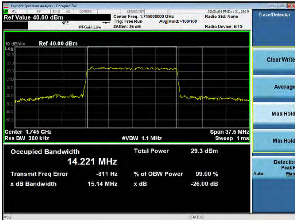
Plot 7-140. Occupied Bandwidth Plot (5G NR n66 - 15.0MHz 256-QAM - CP - Full RB Configuration)
