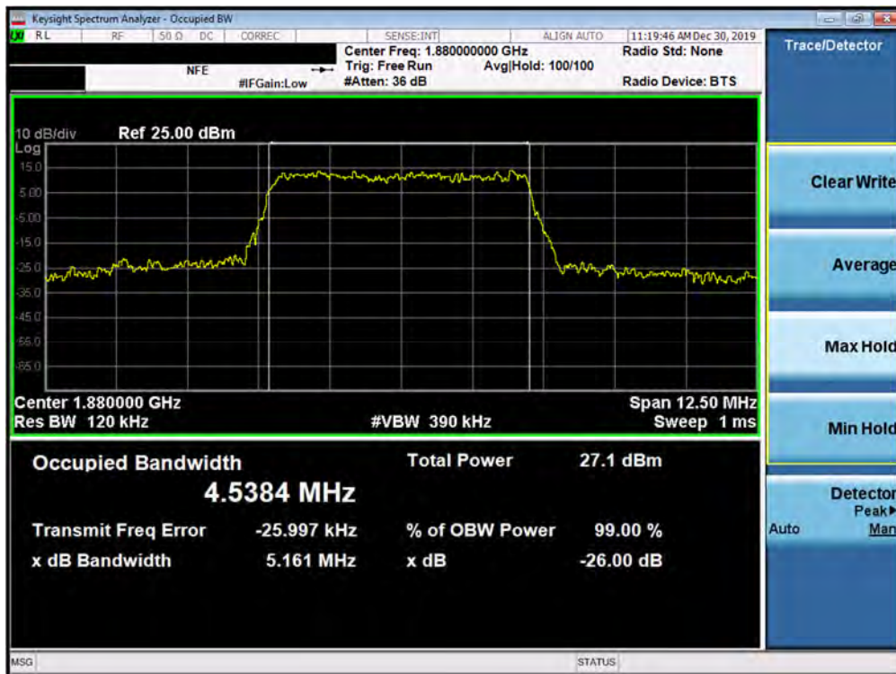
Plot 7-148. Occupied Bandwidth Plot (5G NR n2 - 5.0MHz 256-QAM - CP - Full RB Configuration)
