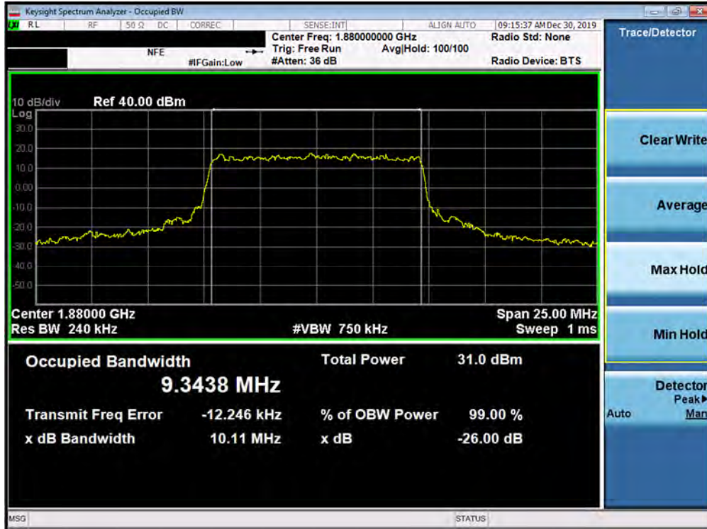
Plot 7-151. Occupied Bandwidth Plot (5G NR n2 - 10.0MHz 64-QAM - CP - Full RB Configuration)
