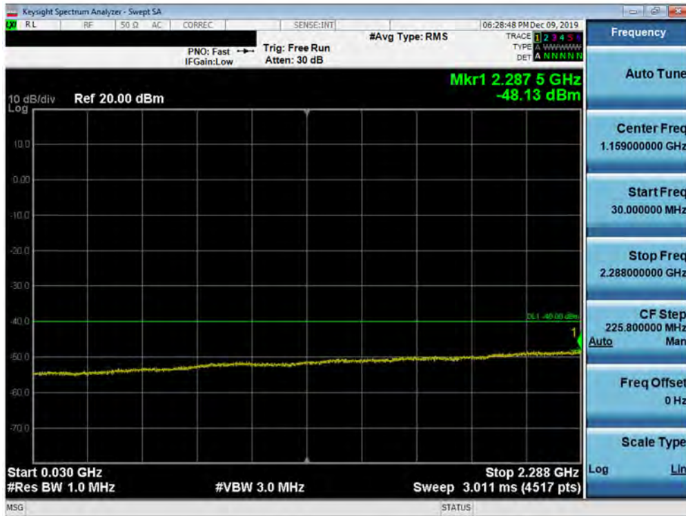
Plot 7-191. Conducted Spurious Plot (Band 30 - 10.0MHz QPSK - RB Size 1, RB Offset 0 – Mid Channel)
