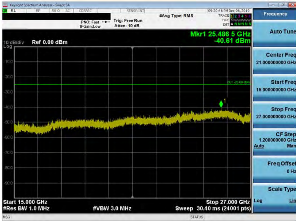
Plot 7-196. Conducted Spurious Plot (Band 41 - 20.0MHz QPSK - RB Size 1, RB Offset 0 - Low Channel)
