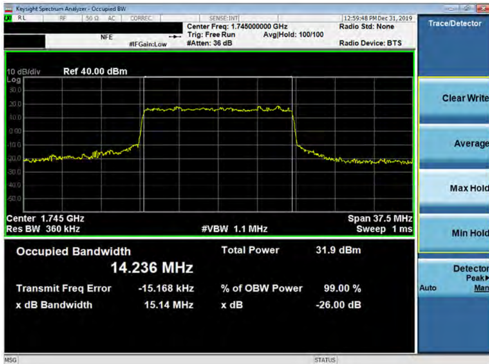
Plot 7-138. Occupied Bandwidth Plot (5G NR n66 - 15.0MHz 16-QAM - CP - Full RB Configuration)
