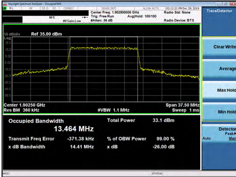
Plot 7-153. Occupied Bandwidth Plot (5G NR n2 - 15.0MHz QPSK - CP - CP - Full RB Configuration)
