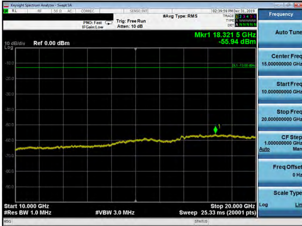
Plot 7-220. Conducted Spurious Plot (5G NR n66 - 15.0MHz QPSK - CP - CP - RB Size 1, RB Offset 0 - High Channel)
