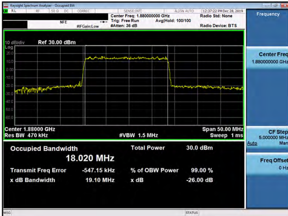
Plot 7-160. Occupied Bandwidth Plot (5G NR n2 - 20.0MHz 256-QAM - CP - Full RB Configuration)
