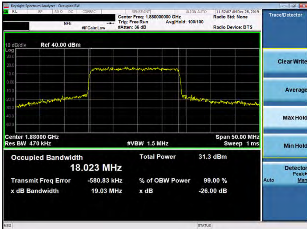
Plot 7-158. Occupied Bandwidth Plot (5G NR n2 - 20.0MHz 16-QAM - CP - Full RB Configuration)
