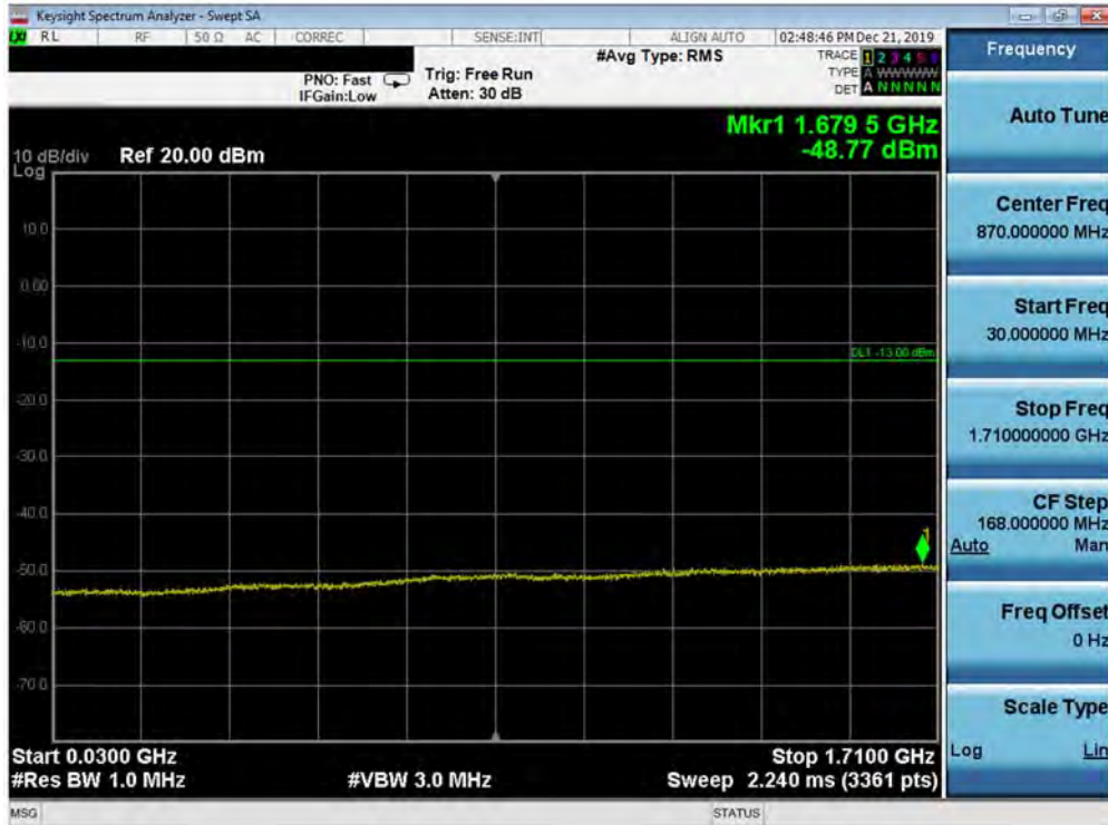
Plot 7-179. Conducted Spurious Plot (Band 66/4 - 20.0MHz QPSK - RB Size 1, RB Offset 0 - High Channel)
