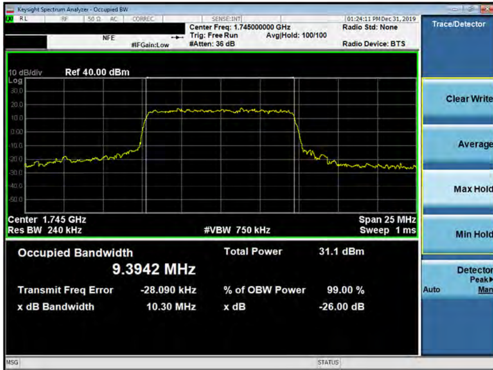
Plot 7-135. Occupied Bandwidth Plot (5G NR n66 - 10.0MHz 64-QAM - CP - Full RB Configuration)
