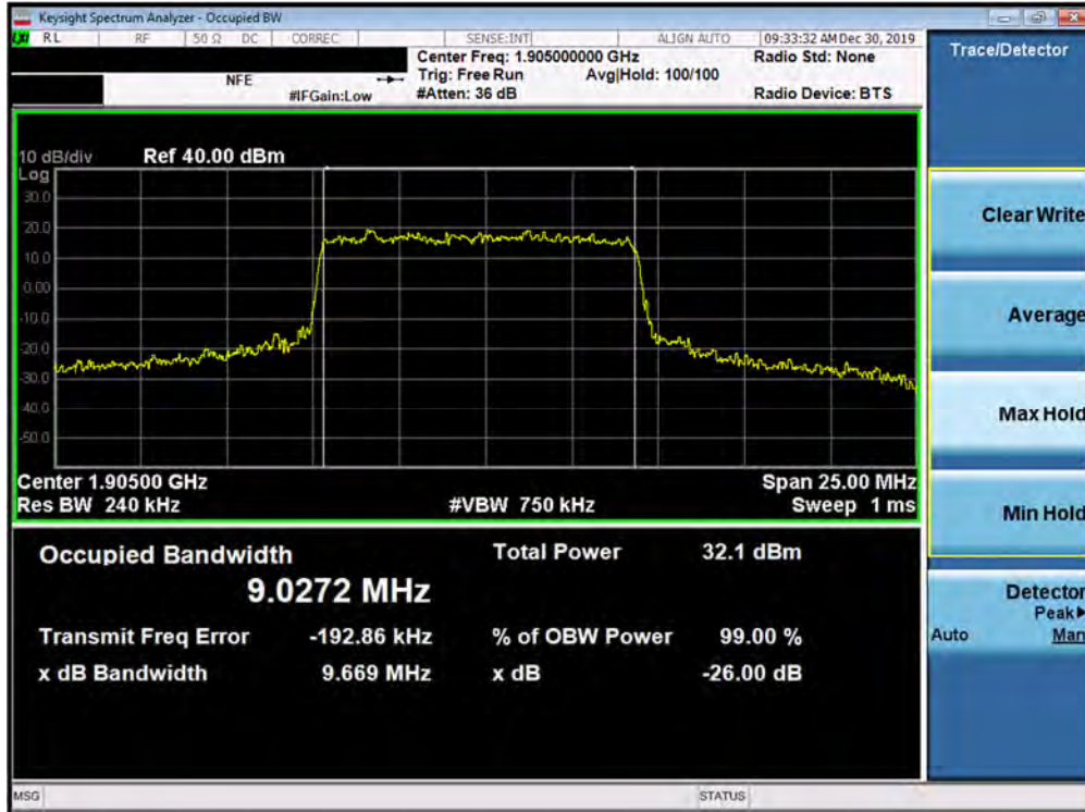
Plot 7-149. Occupied Bandwidth Plot (5G NR n2 - 10.0MHz QPSK - CP - CP - Full RB Configuration)
