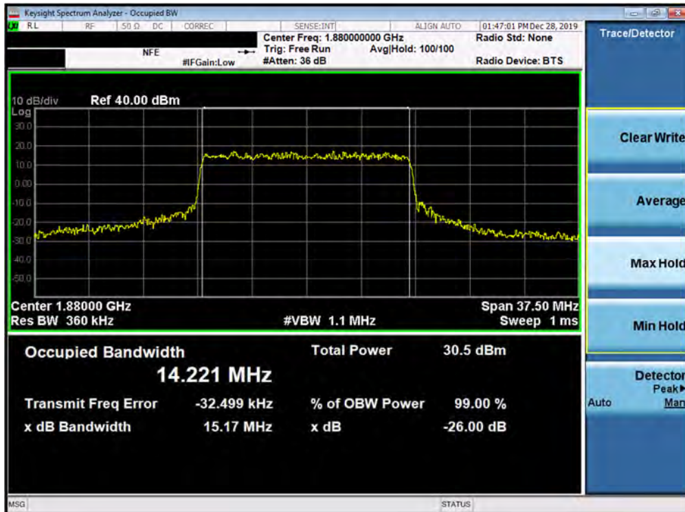
Plot 7-154. Occupied Bandwidth Plot (5G NR n2 - 15.0MHz 16-QAM - CP - Full RB Configuration)
