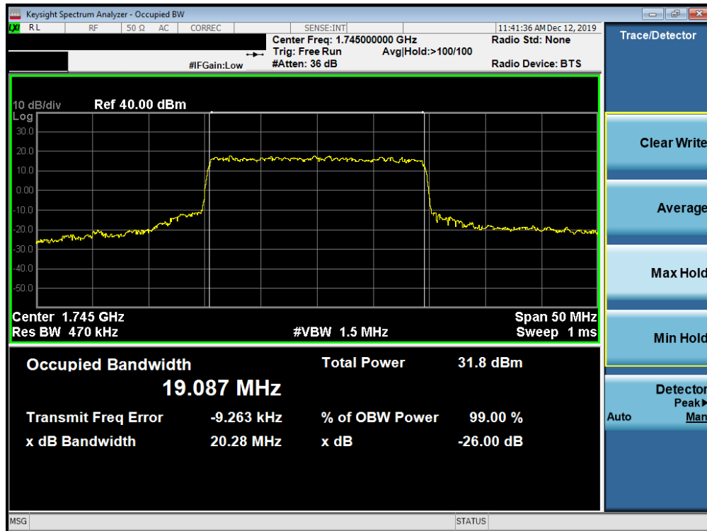
Plot 7-587. Occupied Bandwidth Plot (n66 20MHz 64QAM - CP-OFDM- Full RB Configuration)
