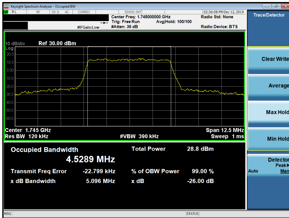
Plot 7-576. Occupied Bandwidth Plot (n66 5MHz 256QAM - CP-OFDM - Full RB Configuration)
