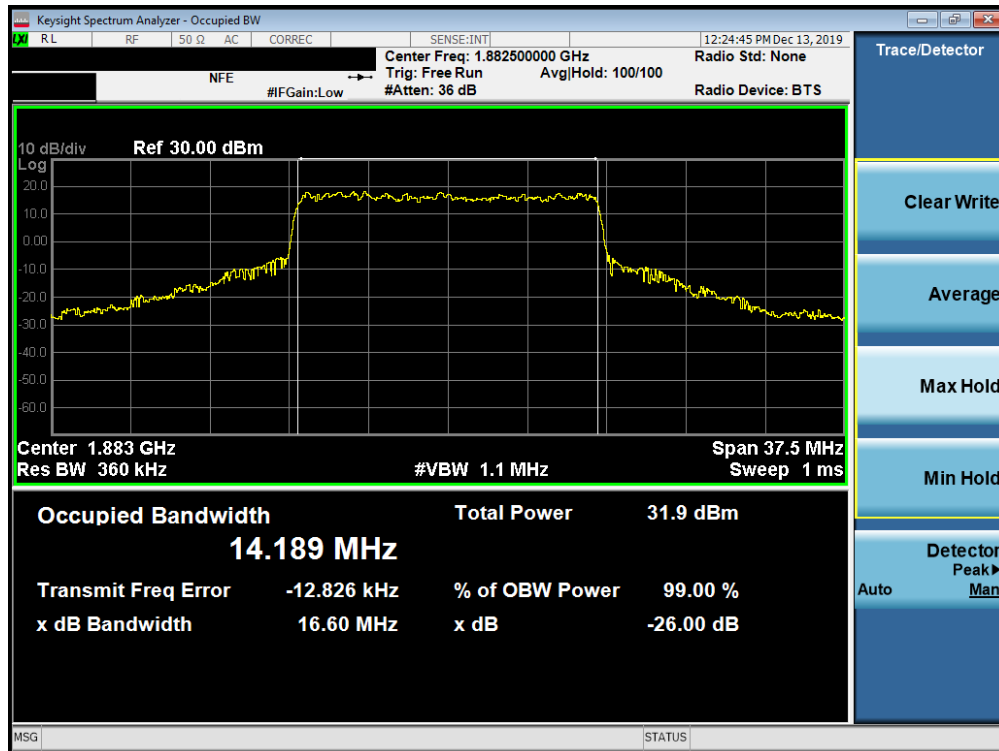
Plot 7-599. Occupied Bandwidth Plot (n25/2 15MHz 64QAM - CP-OFDM- Full RB Configuration)
