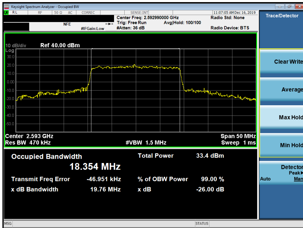
Plot 7-608. Occupied Bandwidth Plot (n41 (PC2) 20MHz 256QAM - CP-OFDM - Full RB Configuration)
