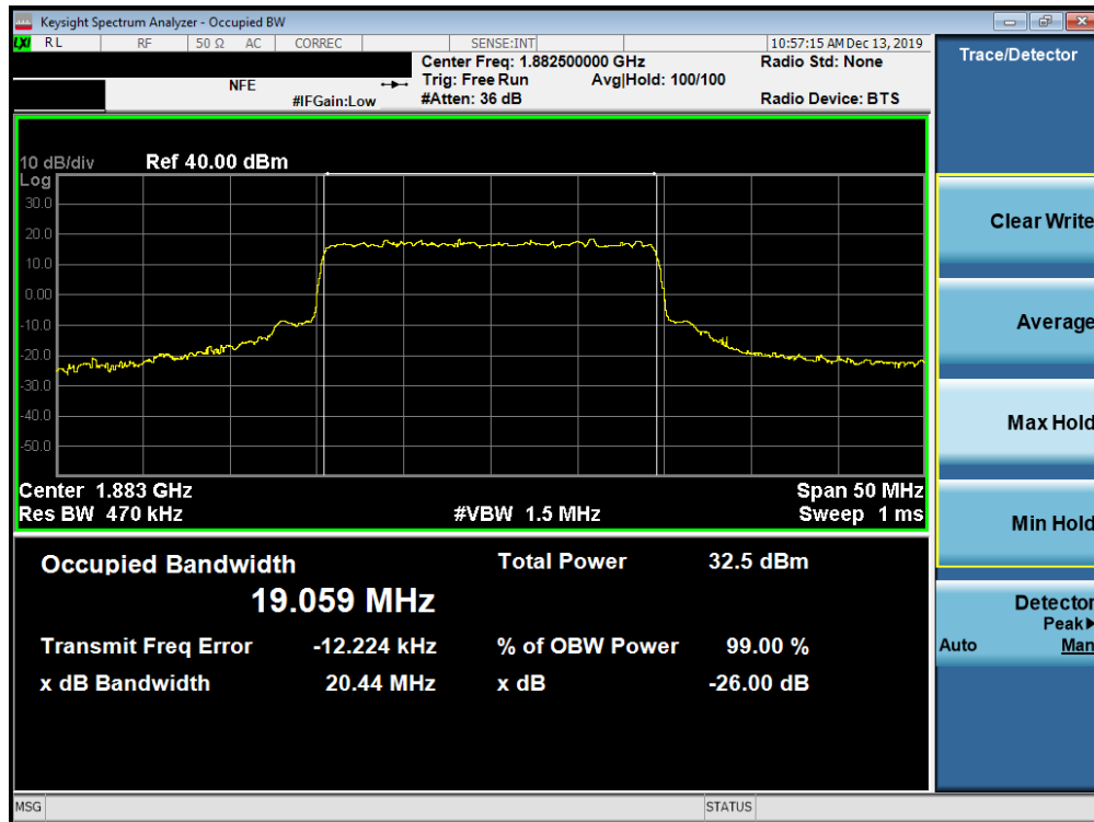
Plot 7-601. Occupied Bandwidth Plot (n25/2 20MHz QPSK - CP-OFDM - Full RB Configuration)
