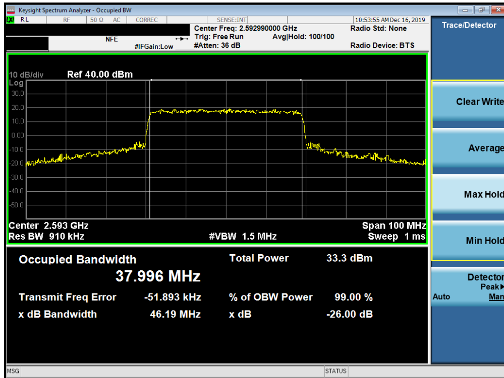
Plot 7-611. Occupied Bandwidth Plot (n41 (PC2) 40MHz 64QAM - CP-OFDM- Full RB Configuration)
