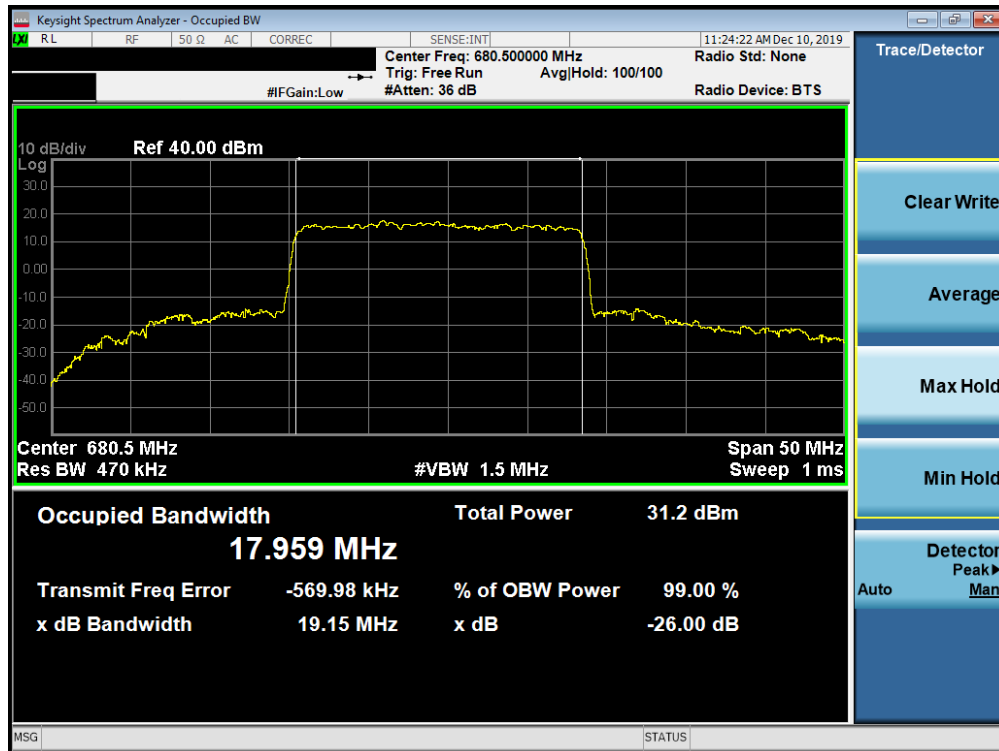
Plot 7-572. Occupied Bandwidth Plot (n71 20MHz 256QAM - CP-OFDM - Full RB Configuration)
