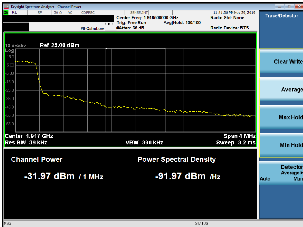
Plot 7-313. Upper Extended Band Edge Plot (Band 25 - 1.4MHz QPSK - Full RB Configuration)
