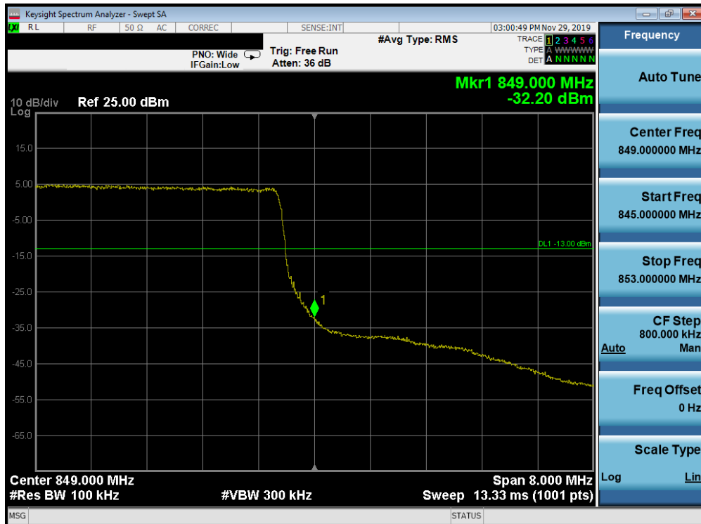
Plot 7-269. Upper Band Edge Plot (Band 26/5 - 10.0MHz QPSK - Full RB Configuration)
