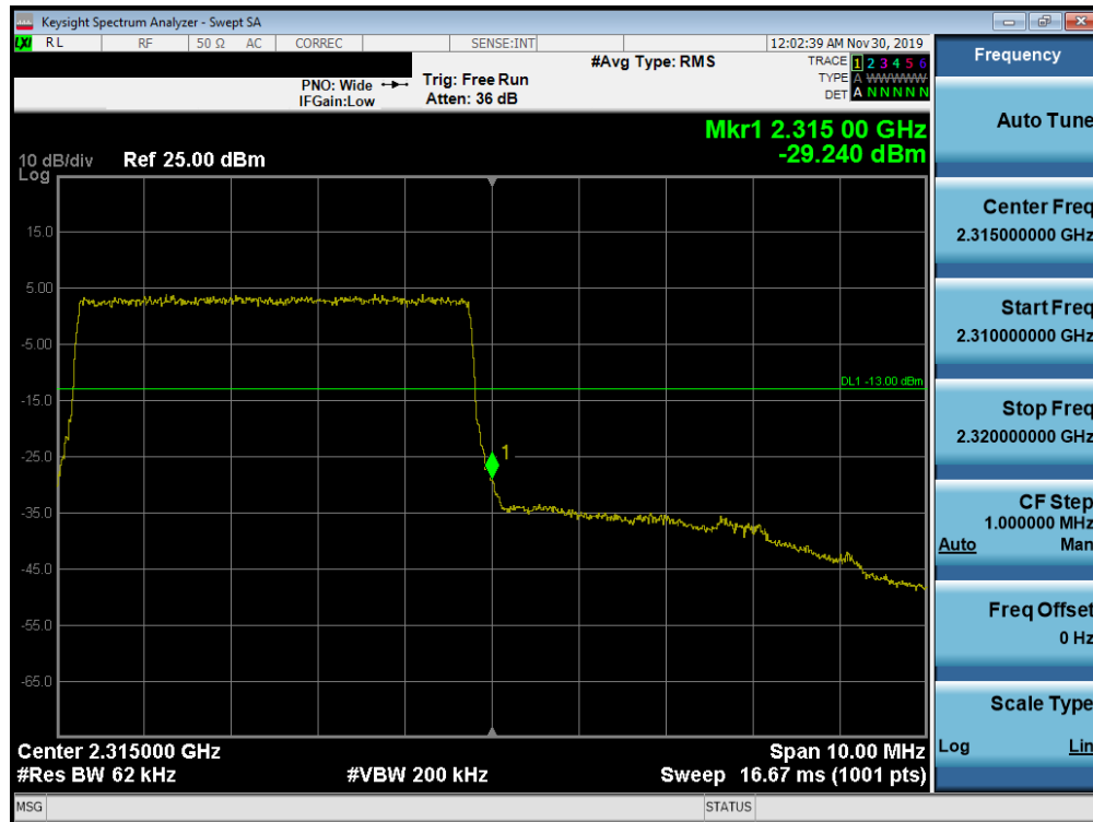
Plot 7-346. Upper Band Edge Plot (Band 30 - 5.0MHz QPSK - Full RB Configuration)
