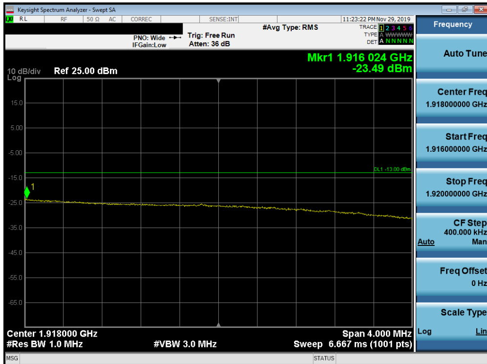
Plot 7-337. Upper Extended Band Edge Plot (Band 25 - 15.0MHz QPSK - Full RB Configuration)
