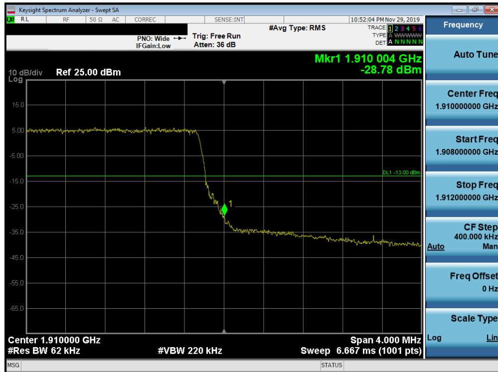
Plot 7-322. Upper Band Edge Plot (Band 2 - 5.0MHz QPSK - Full RB Configuration)
