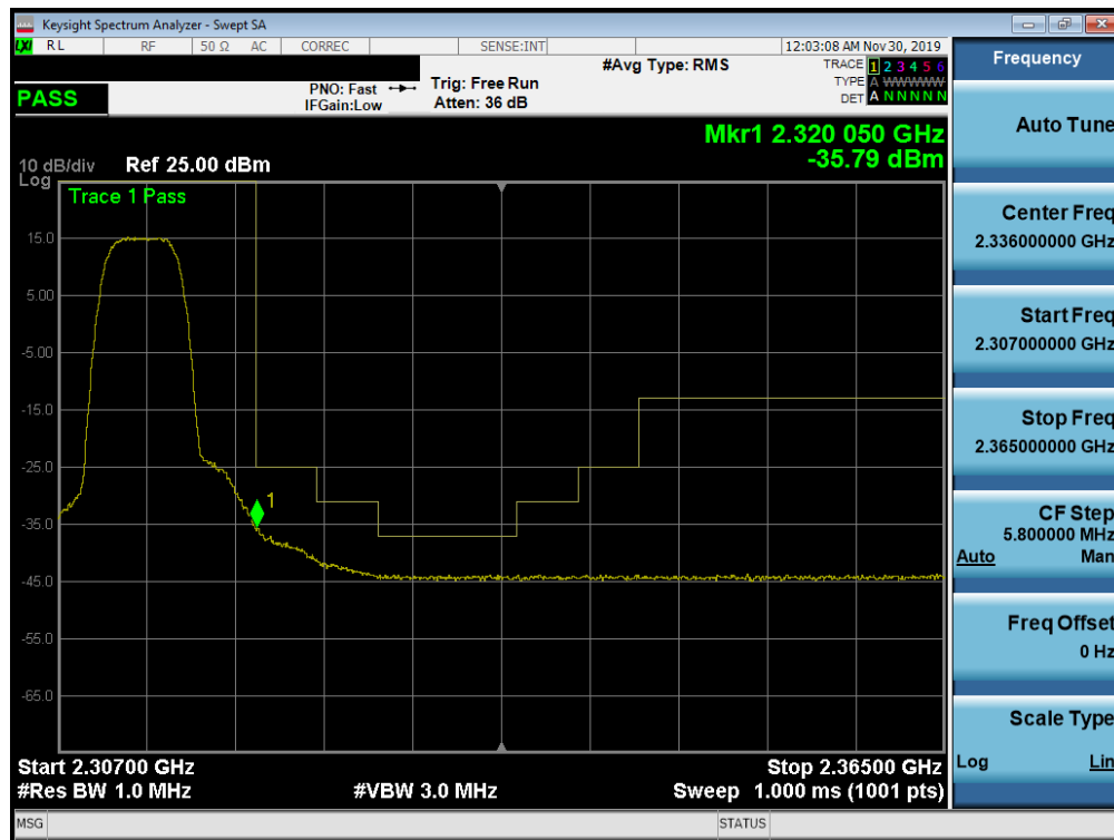
Plot 7-347. Upper Extended Band Edge Plot (Band 30 - 5.0MHz QPSK - Full RB Configuration)
