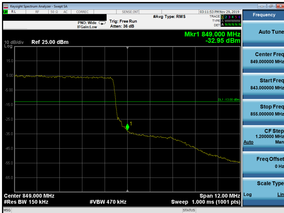
Plot 7-271. Upper Band Edge Plot (Band 26 - 15.0MHz QPSK - Full RB Configuration)
