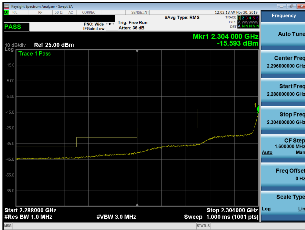
Plot 7-345. Lower Extended Band Edge Plot (Band 30 - 5.0MHz QPSK - Full RB Configuration)
