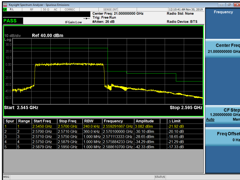
Plot 7-362. Higher ACP Plot (Band 7 - 20.0MHz QPSK - Full RB Configuration)
