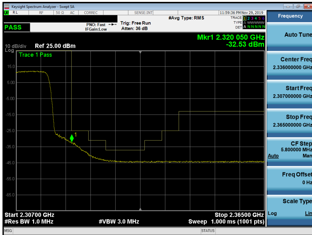
Plot 7-354. Upper Extended Band Edge Plot (Band 30 - 10.0MHz QPSK - Full RB Configuration)
