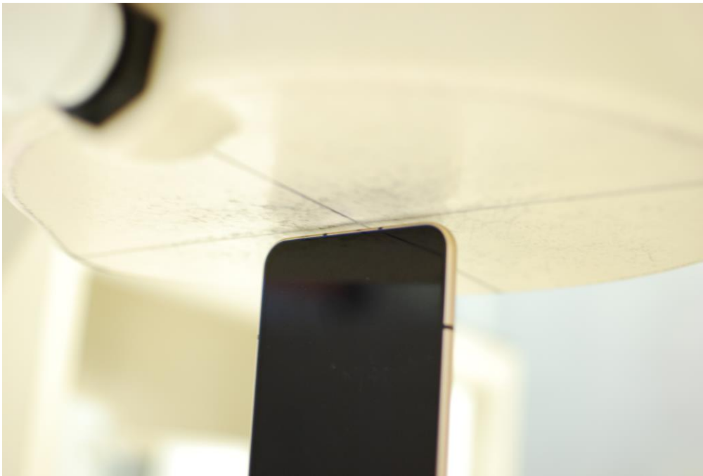
SAR Test Setup Photo 14 – Bottom Edge at 3
