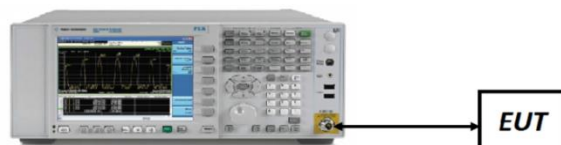
Figure 7-5. Test Instrument & Measurement Setup
