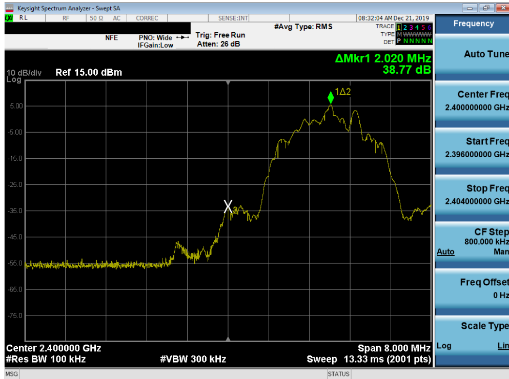
Plot 7-43. Band Edge Plot (Bluetooth (LE), 2Mbps – Ch. 0)
