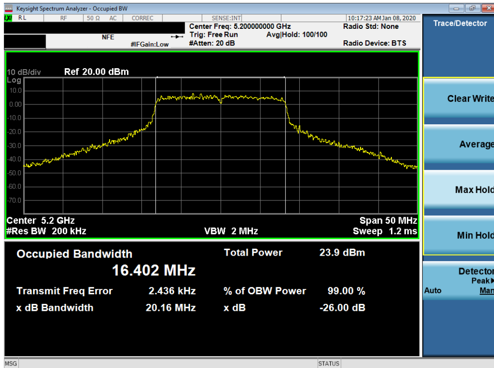
Plot 7-51. 26dB Bandwidth Plot SISO ANT2 (802.11a (UNII Band 1) – Ch. 40)
