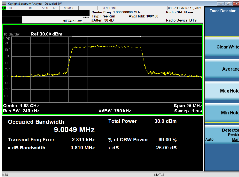
Plot 7-71. Occupied Bandwidth Plot (Band 2 - 10.0MHz 64-QAM - Full RB Configuration)
