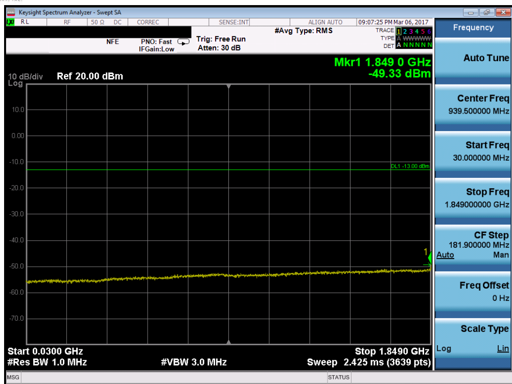
Plot 7-67. Conducted Spurious Plot (Band 2 – 15MHz QPSK – RB Size 1, RB Offset 0 – Low Channel)
