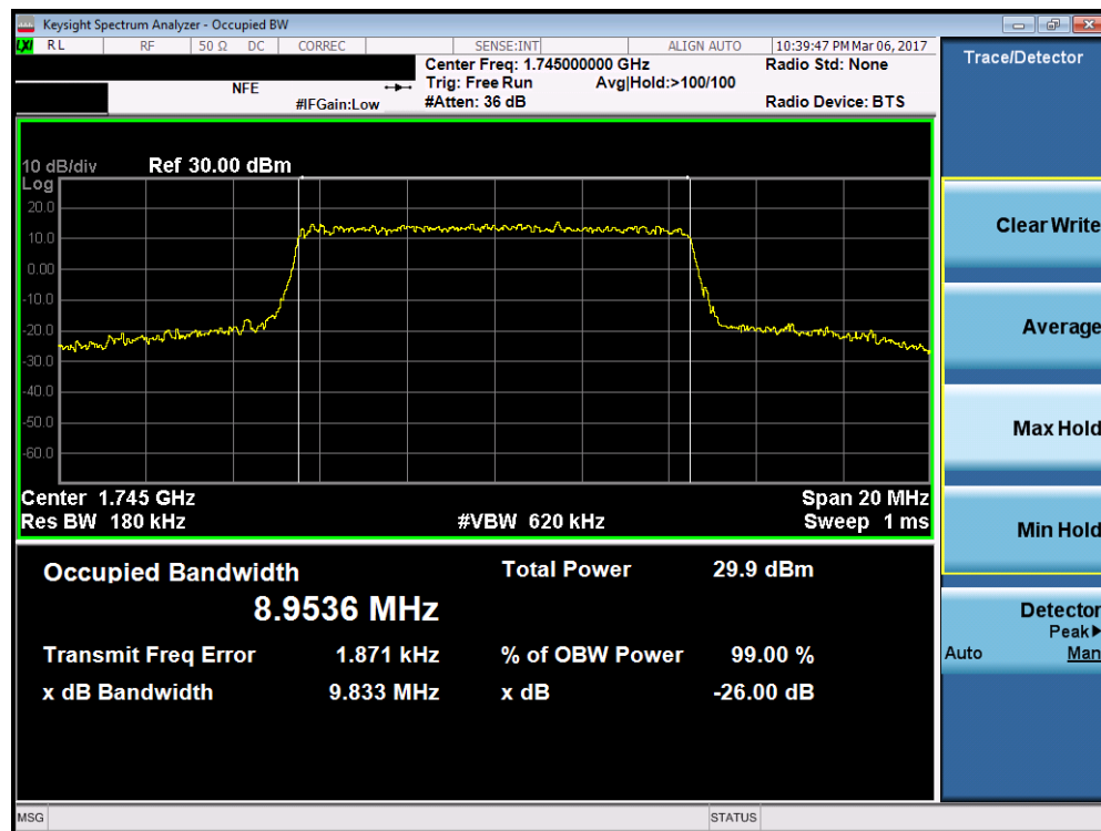
Plot 7-36. Occupied Bandwidth Plot (Band 66 – 10.0MHz 16-QAM – RB Size 50)
