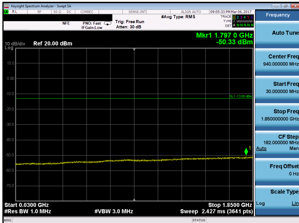
Plot 7-70. Conducted Spurious Plot (Band 2 – 15MHz QPSK – RB Size 1, RB Offset 0 – Mid Channel)
