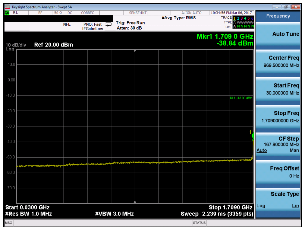
Plot 7-76. Conducted Spurious Plot (Band 66 – 5.0MHz QPSK – RB Size 1, RB Offset 0 – Low Channel)
