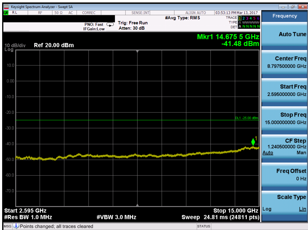
Plot 7-92. Conducted Spurious Plot (Band 7 – 10.0MHz QPSK – RB Size 1, RB Offset 0 – High Channel)
