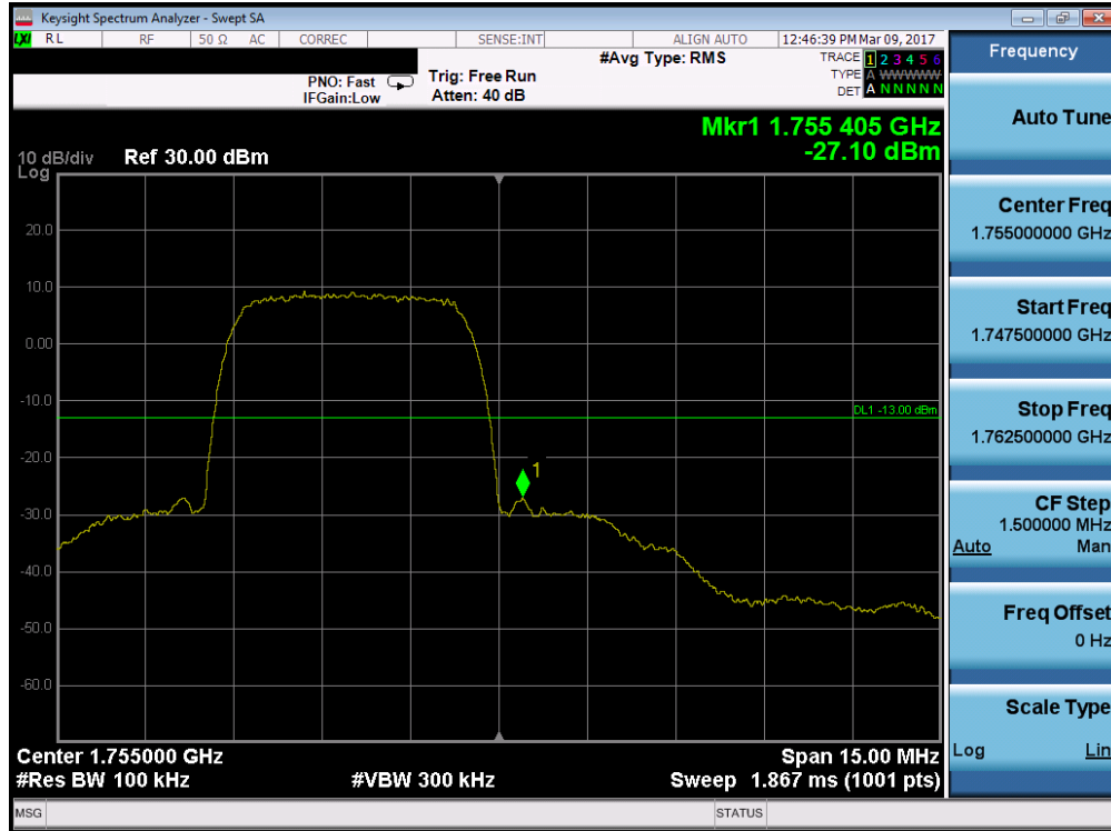
Plot 7-35. Band Edge Plot (AWS WCDMA Mode – Ch. 1513)
