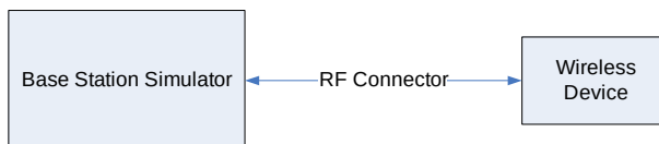
Figure 8-1 Power Measurement Setup
