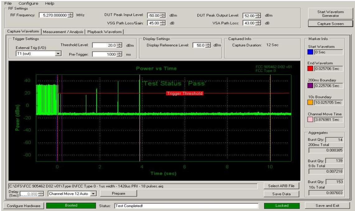
Figure 5-5. Band 2A Move Time and Aggregate Time
