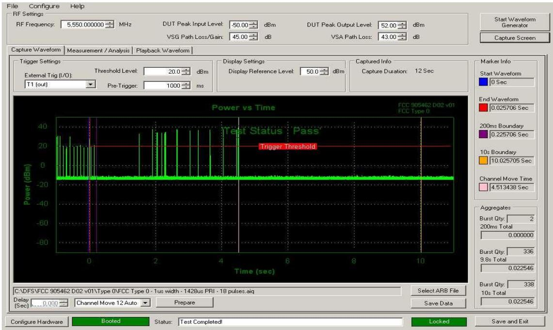
Figure 5-6. Band 2C Move Time and Aggregate Time
