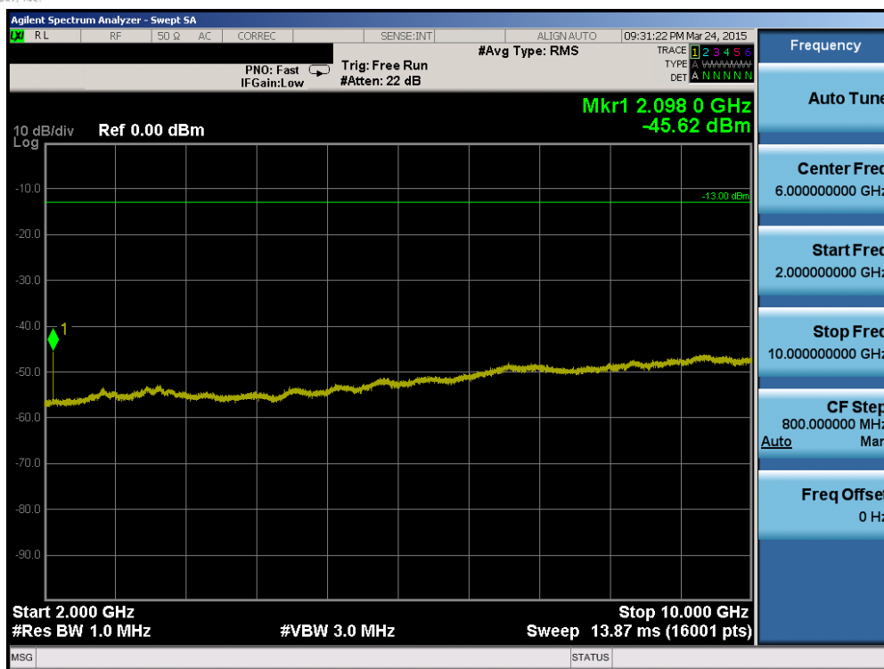
Plot 6-35. Conducted Spurious Plot (Band 12 – 3.0MHz QPSK – RB Size 1, RB Offset 0 – Low Channel)
