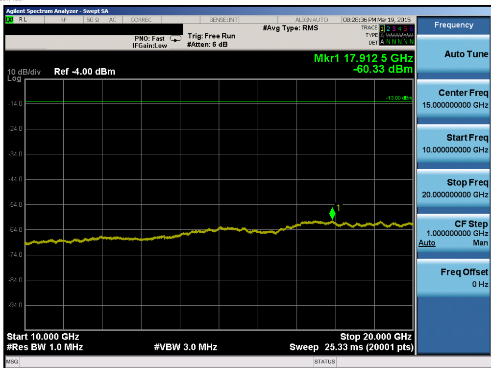
Plot 6-59. Conducted Spurious Plot (Band 2 – 1.4MHz QPSK – RB Size 1, RB Offset 0 – High Channel)
