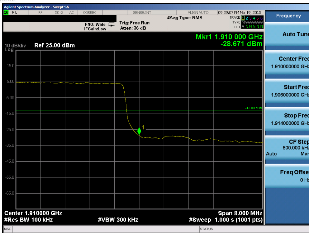
Plot 6-114. Upper Band Edge Plot (Band 2 – 10.0MHz QPSK – RB Size 50)
