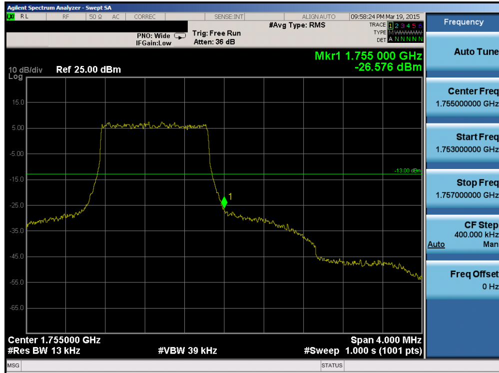
Plot 6-78. Upper Band Edge Plot (Band 4 – 1.4MHz QPSK – RB Size 6)
