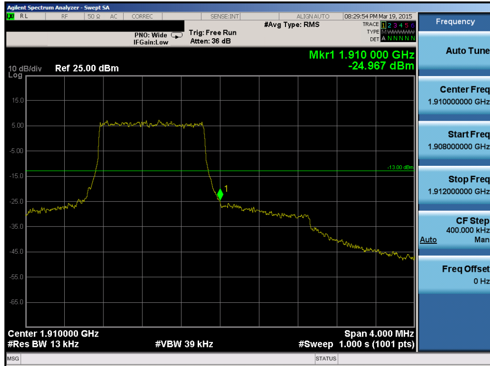
Plot 6-102. Upper Band Edge Plot (Band 2 – 1.4MHz QPSK – RB Size 6)
