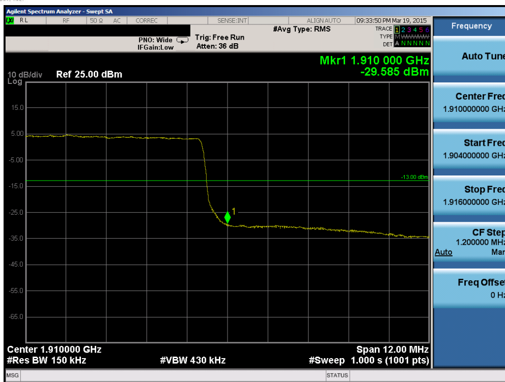
Plot 6-118. Upper Band Edge Plot (Band 2 – 15.0MHz QPSK – RB Size 75)
