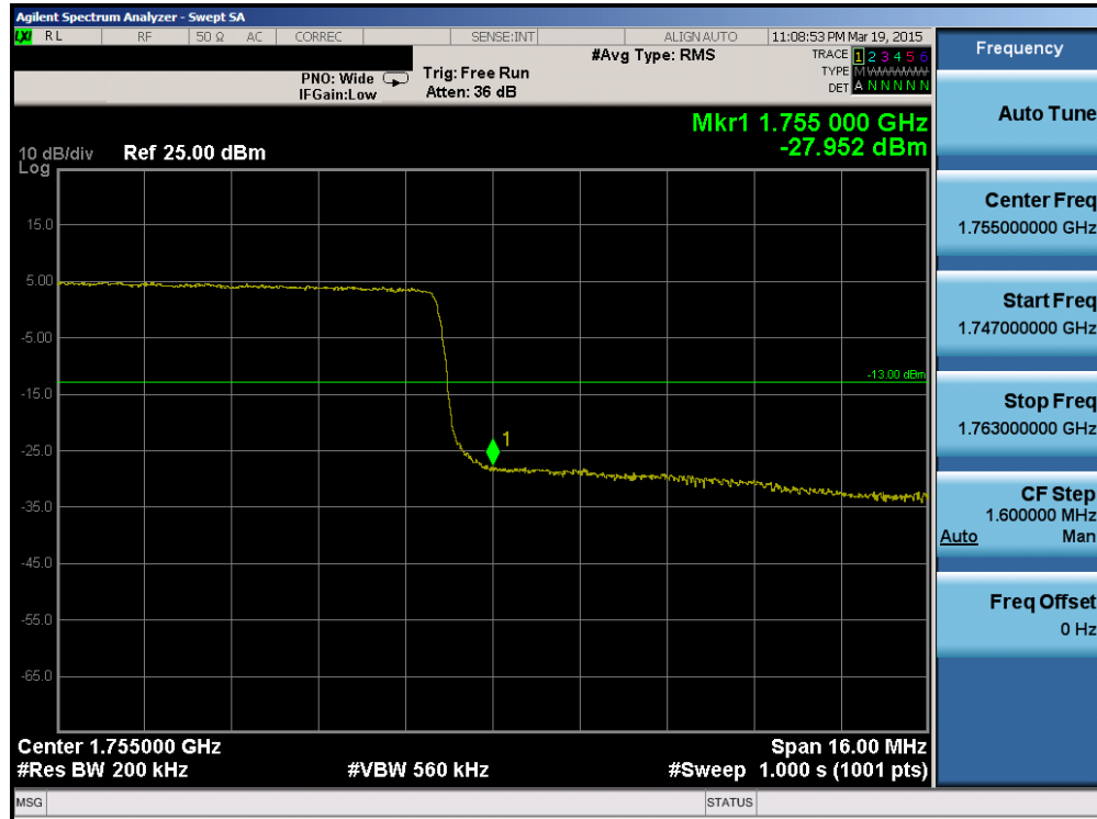
Plot 6-98. Upper Band Edge Plot (Band 4 – 20.0MHz QPSK – RB Size 100)
