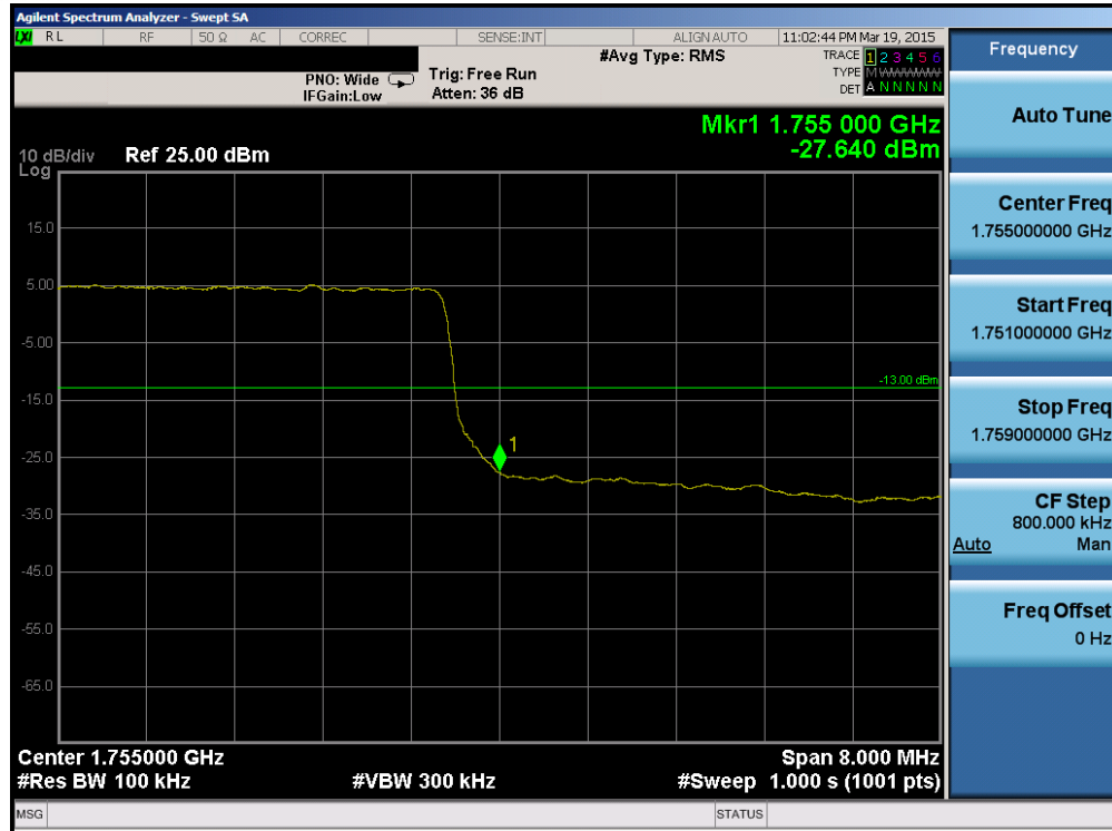
Plot 6-90. Upper Band Edge Plot (Band 4 – 10.0MHz QPSK – RB Size 50)
