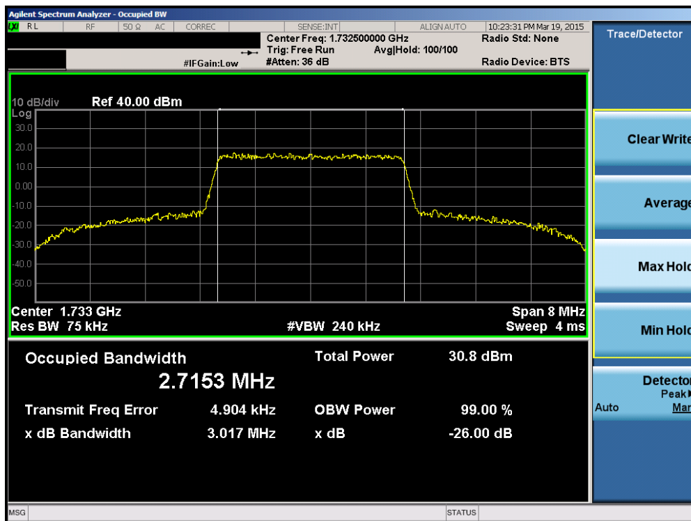
Plot 6-12. Occupied Bandwidth Plot (Band 4 – 3.0MHz 16-QAM – RB Size 15)
