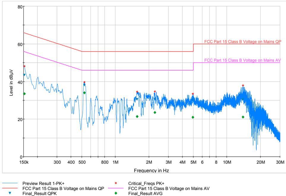
**Plot 6-97. Line Conducted Plot with 802.11a UNII Band 1 (L1)**
