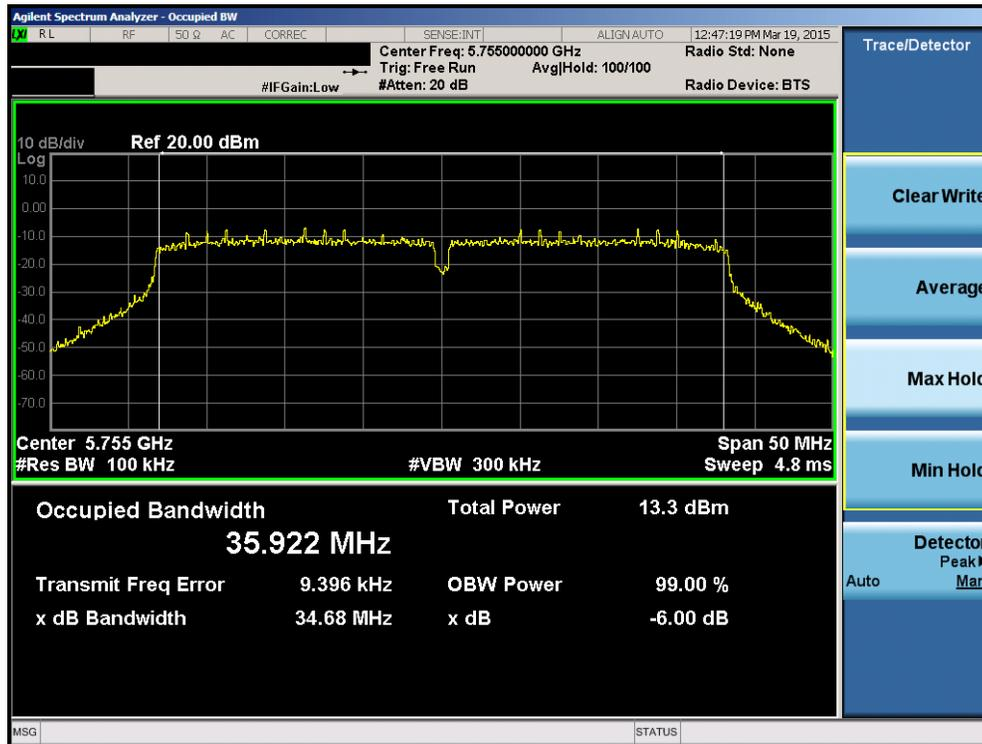
Plot 6-32. 6dB Bandwidth Plot (802.11n (UNII Band 3) – Ch. 151)
