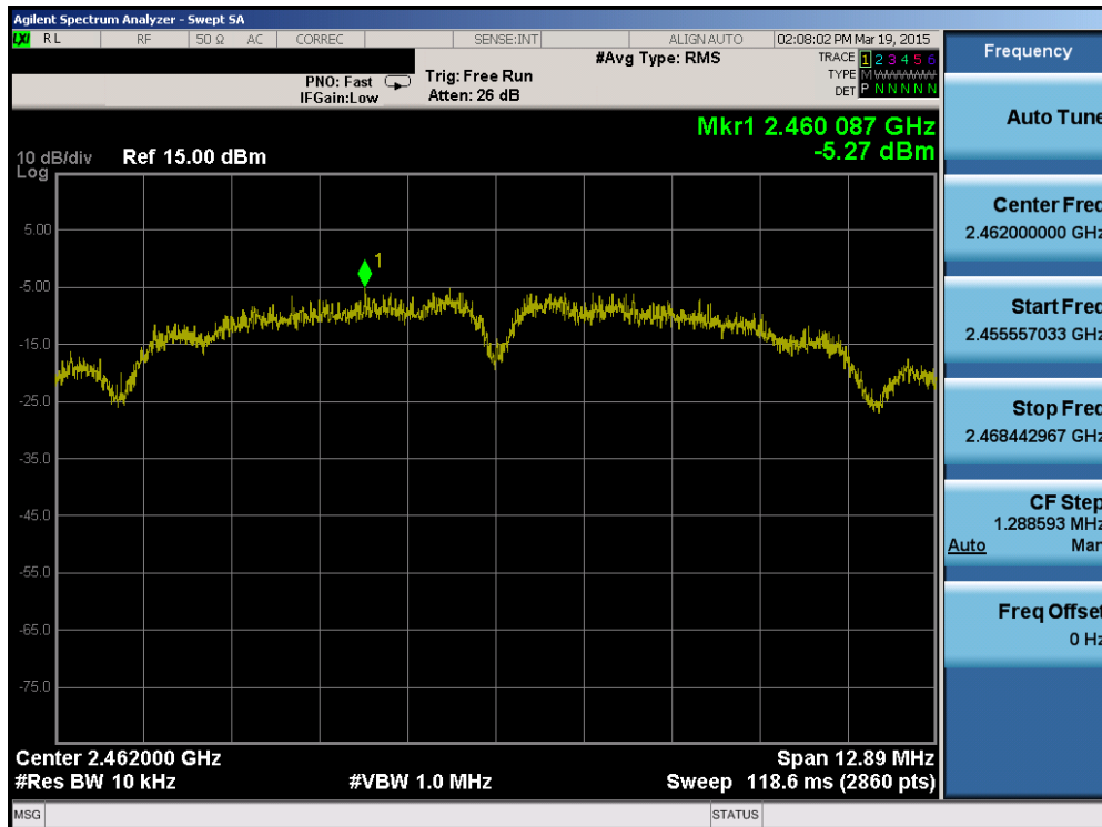
Plot 6-12. Power Spectral Density Plot (802.11b – Ch. 11)
