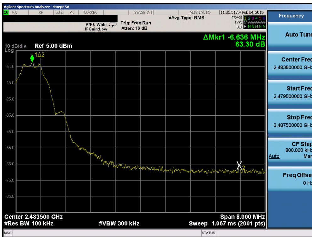
Plot 6-11. Band Edge Plot (Bluetooth (LE) – Ch. 39)
