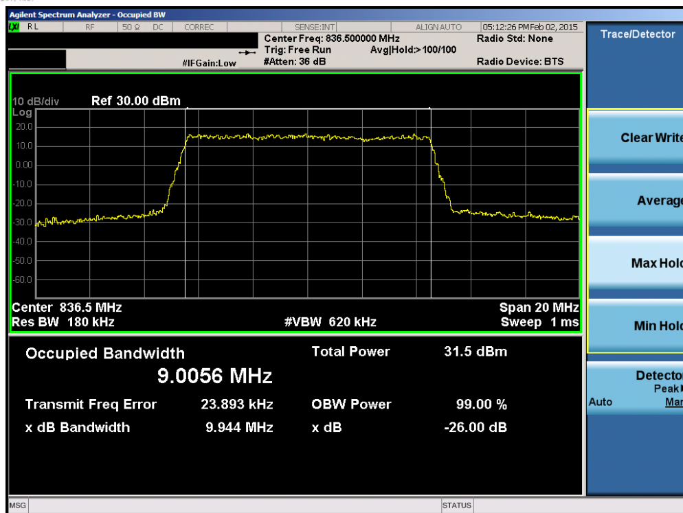
Plot 6-15. Occupied Bandwidth Plot (Band 5 – 10.0MHz QPSK – RB Size 50)
