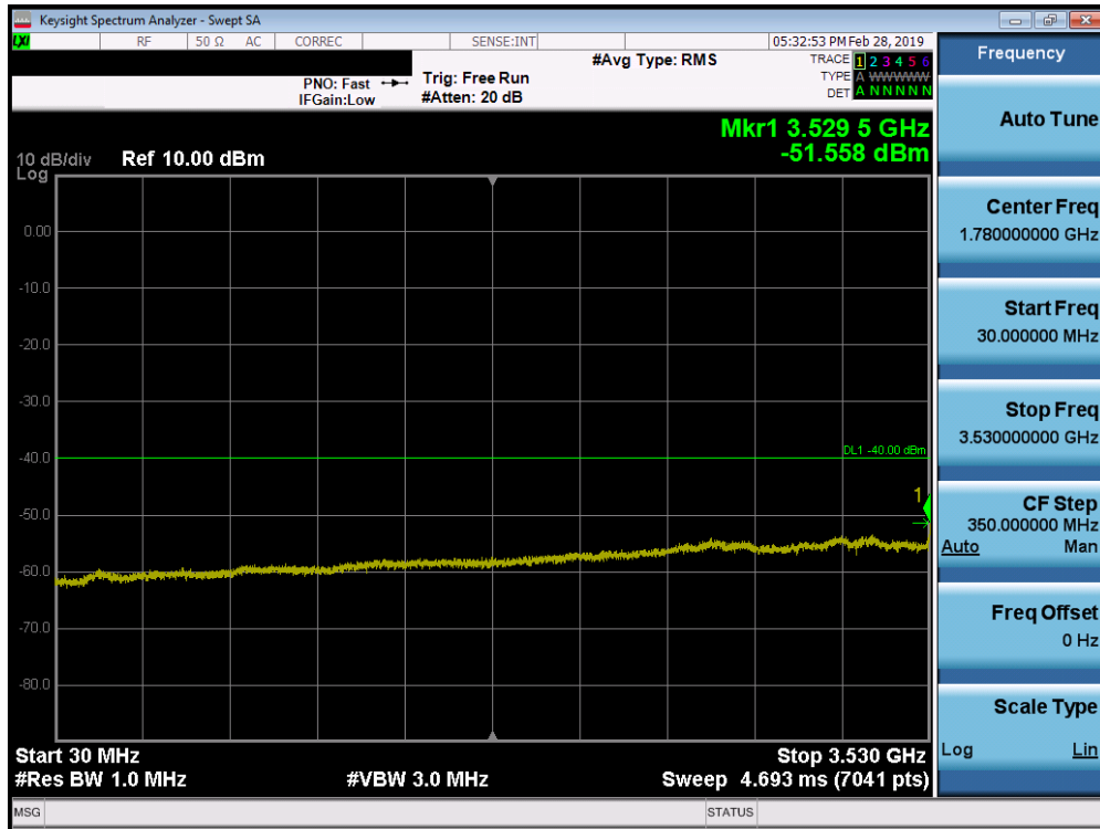
Plot 7-13. Conducted Spurious Plot (Band 48 - 15.0MHz QPSK - RB Size 1, RB Offset 0 - Low Channel)
