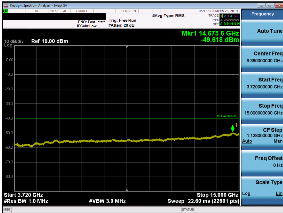
Plot 7-14. Conducted Spurious Plot (Band 48 - 15.0MHz QPSK - RB Size 1, RB Offset 0 - Low Channel)
