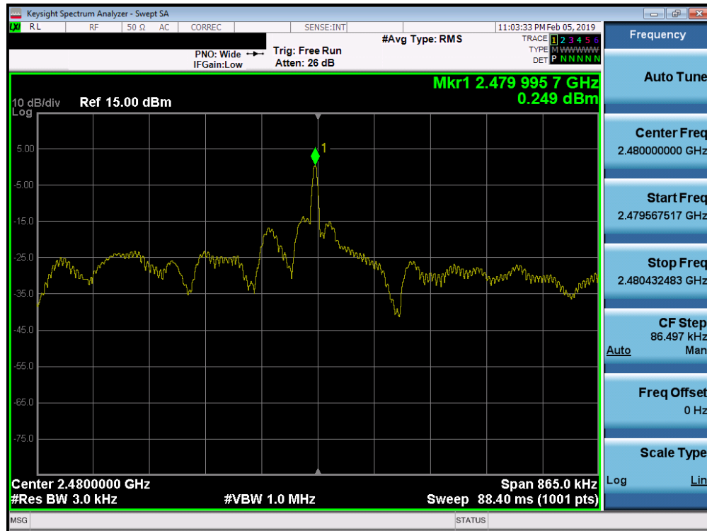
Plot 7-18. Power Spectral Density Plot (Bluetooth (LE), 2Mbps – Ch. 39)
