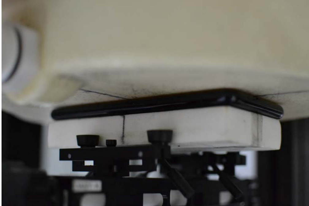
SAR Test Setup Photo 9 – Front Side at 1mm
