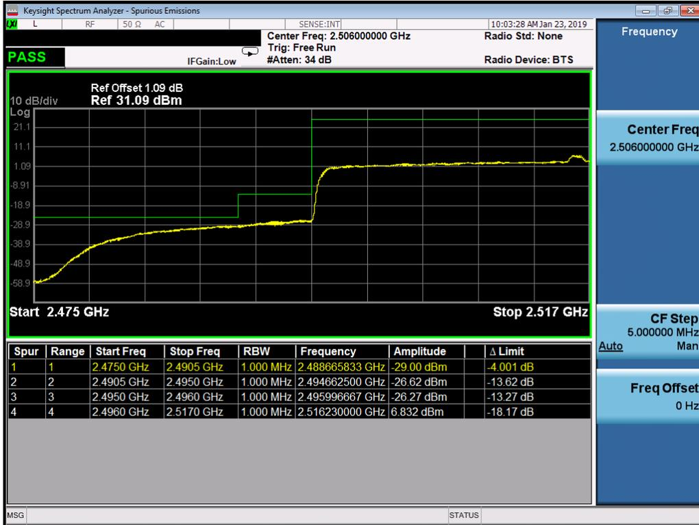
Plot 33. Lower Band Edge Plot (n41 - 40MHz CP-16QAM - Full RB Configuration)
