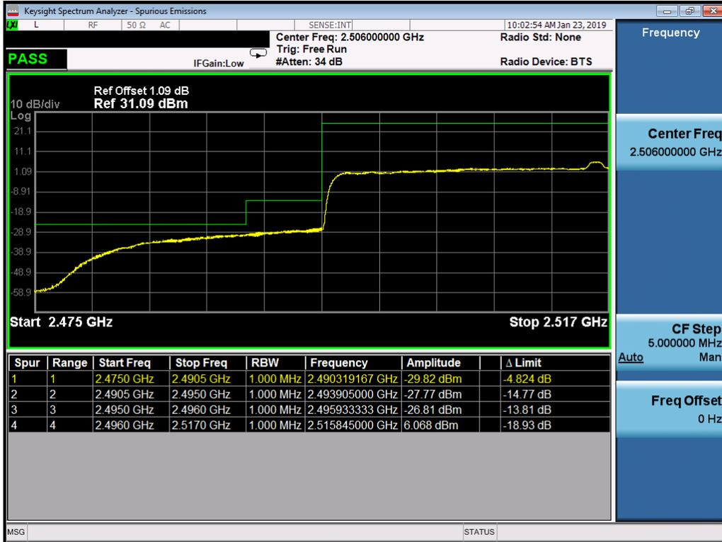
Plot 35. Lower Band Edge Plot (n41 - 40MHz CP-64QAM - Full RB Configuration)
