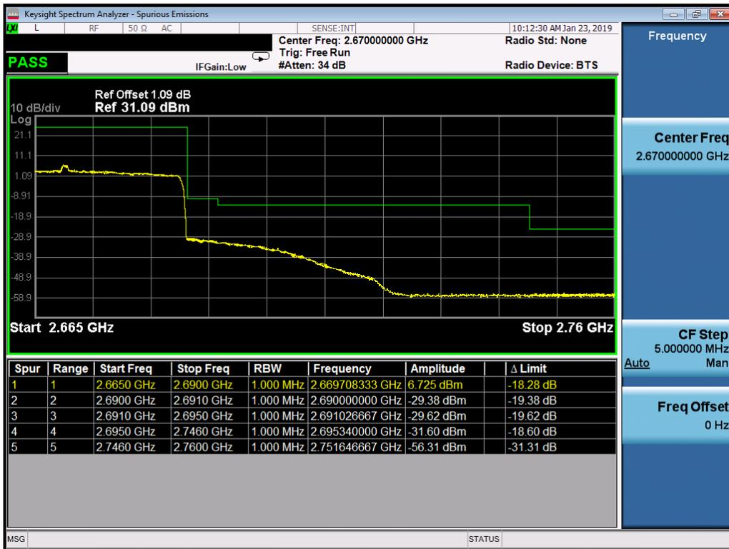
Plot 34. Upper Band Edge Plot (n41 - 40MHz CP-16QAM - Full RB Configuration)
