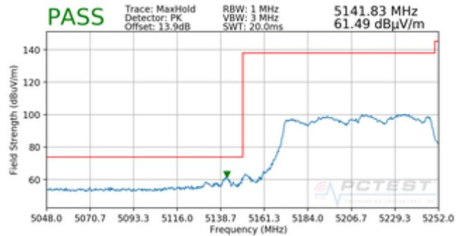
**Plot 7-98. Radiated Lower Band Edge Plot MIMO (Peak – UNII Band 1)**
