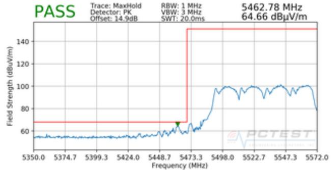
**Plot 7-102. Radiated Lower Band Edge Plot MIMO (Peak – UNII Band 2C)**
