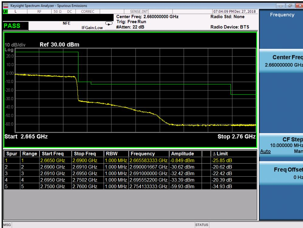
Plot 329. Upper Band Edge Plot (n41 - 60MHz CP-64QAM - Full RB Configuration)
