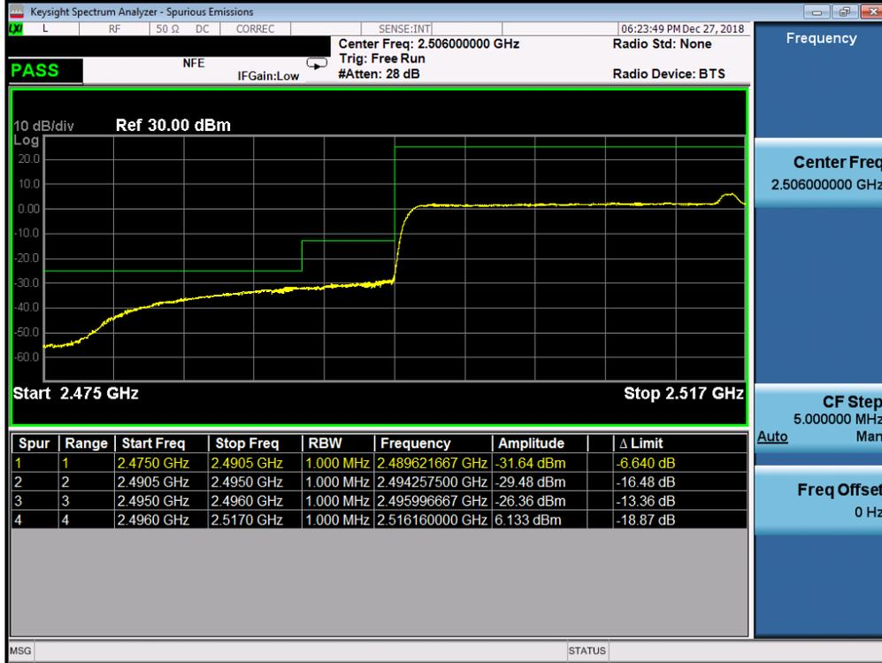
Plot 334. Lower Band Edge Plot (n41 - 40MHz CP-64QAM - Full RB Configuration)
