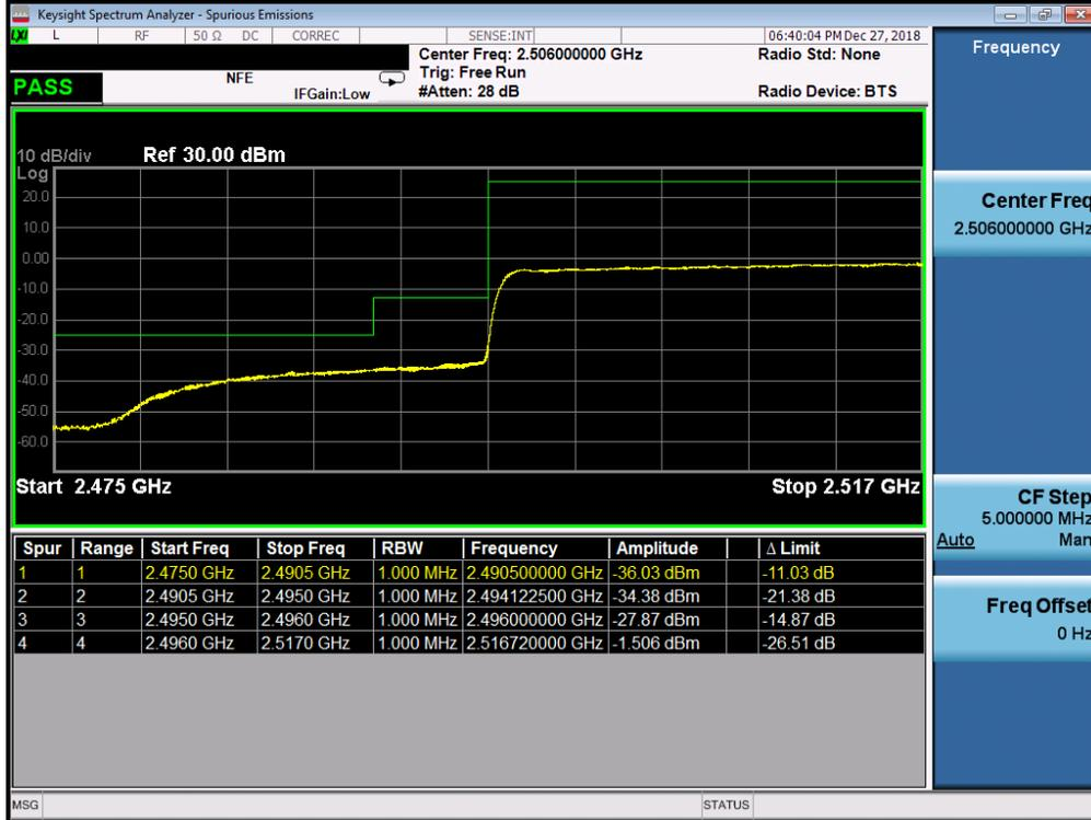
Plot 324. Lower Band Edge Plot (n41 - 60MHz CP-QPSK - Full RB Configuration)
