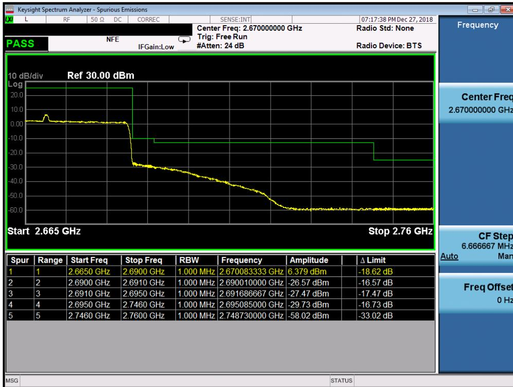
Plot 335. Upper Band Edge Plot (n41 - 40MHz CP-64QAM - Full RB Configuration)
