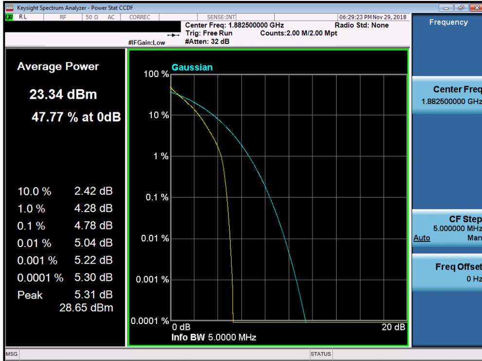
Plot 7-270. PAR Plot (Band 25/2 - 5.0MHz QPSK - Full RB Configuration)
