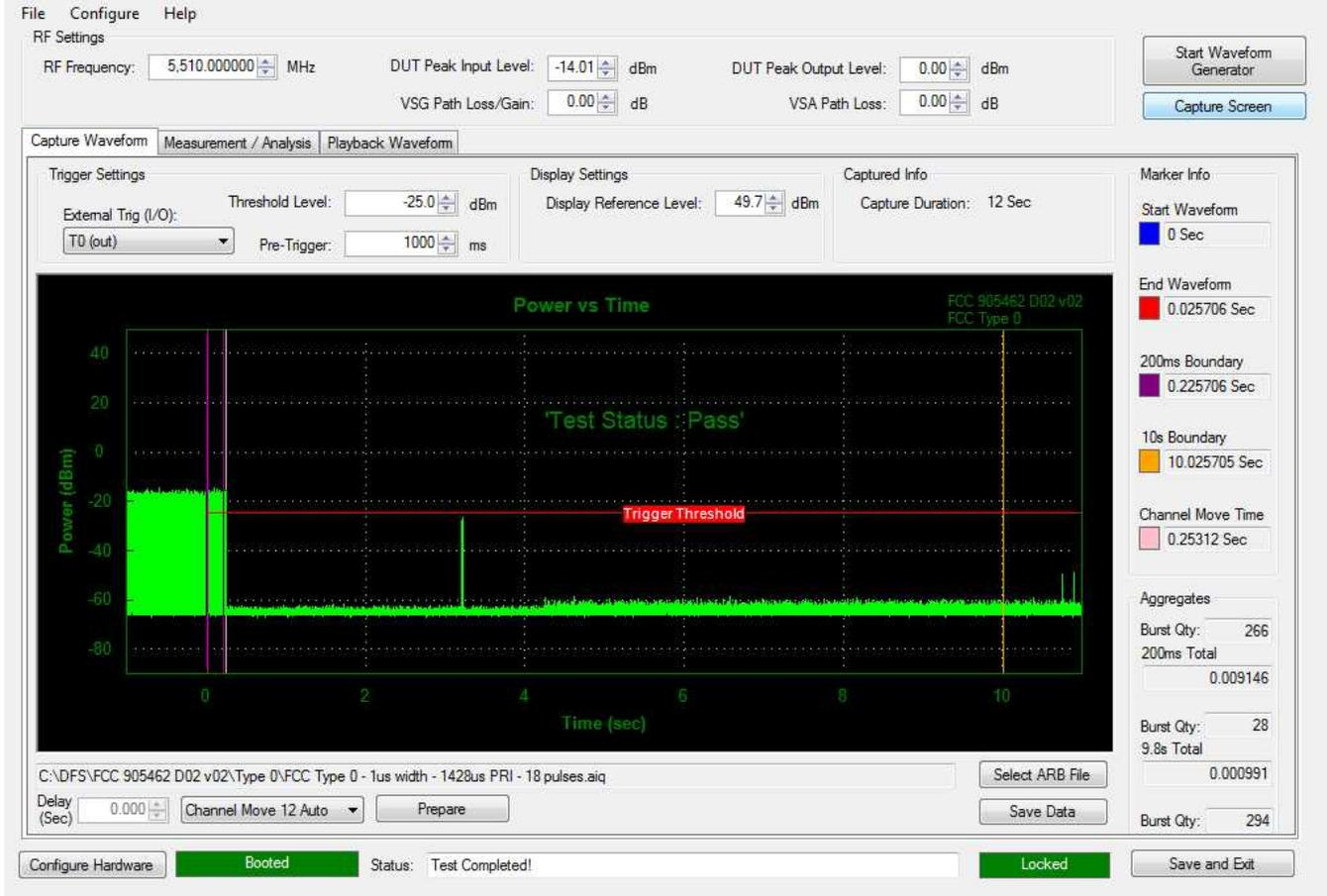
**Figure 5-4. Band 2C Move Time and Aggregate Time**
