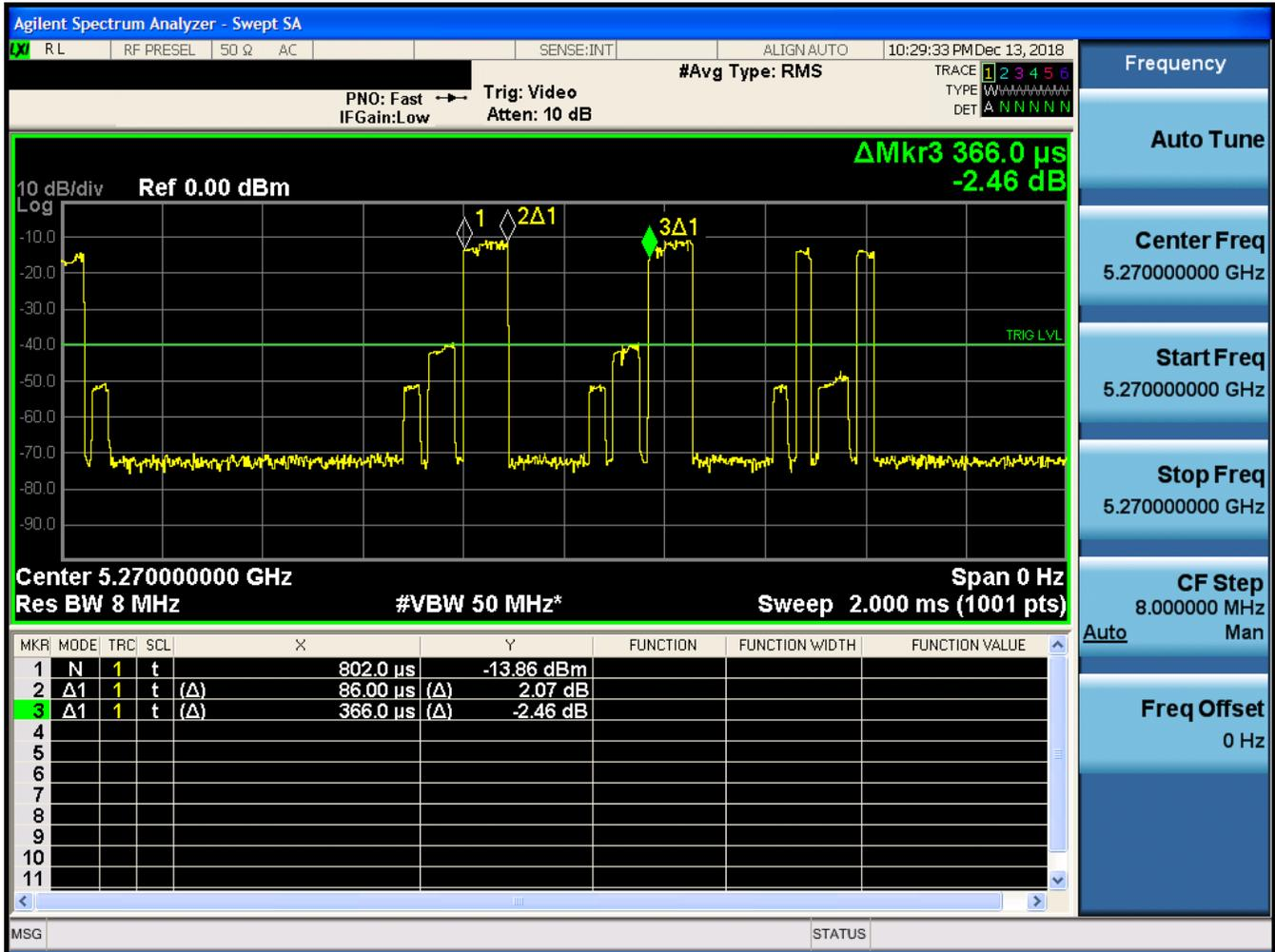
Figure 5-1. Band 2A Pulse Width and Period
