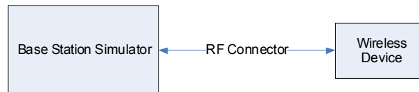
Figure 8-1 Power Measurement Setup
