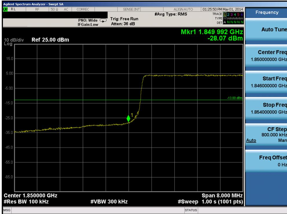
Plot 6-65. Lower Band Edge Plot (Band 2 – 10.0MHz QPSK – RB Size 50)
