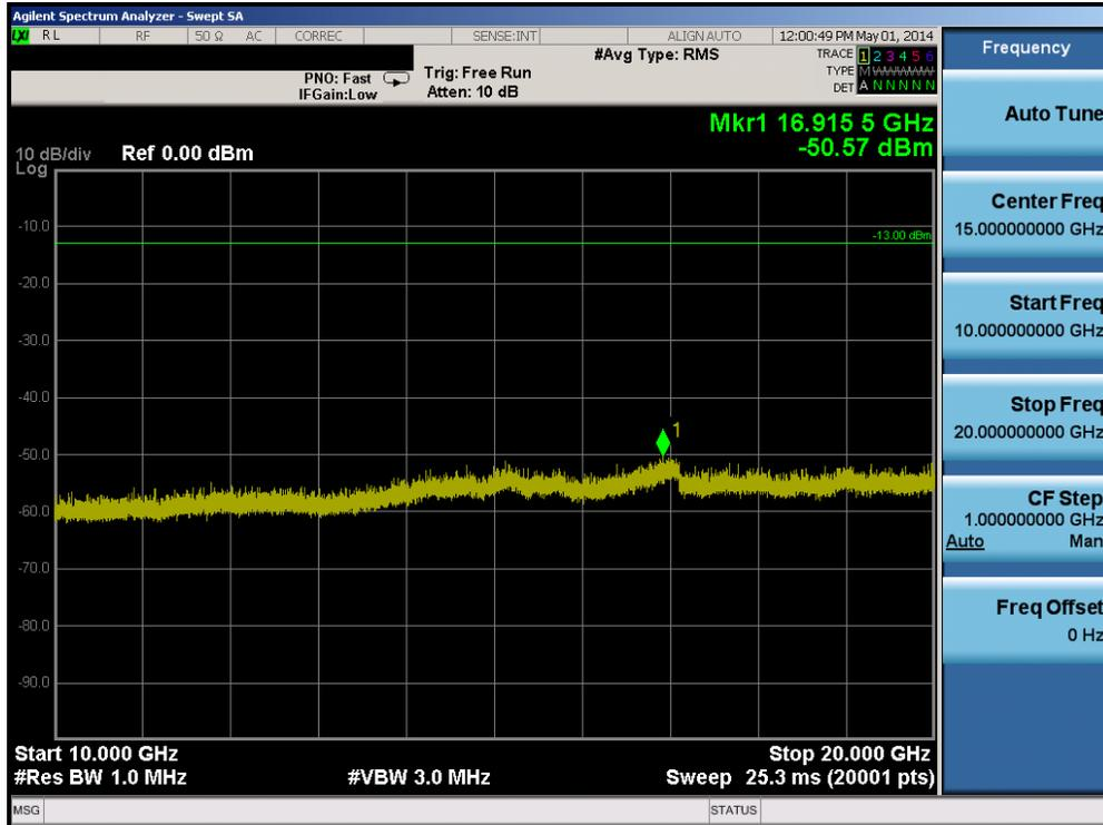
Plot 6-36. Conducted Spurious Plot (Band 2 – 5.0MHz QPSK – RB Size 1, RB Offset 0 – Low Channel)
