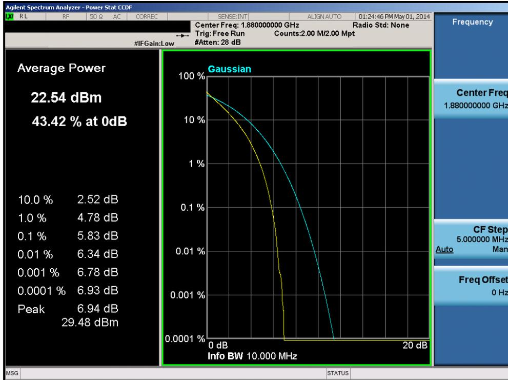
Plot 6-75. PAR Plot (Band 2 – 10.0MHz QPSK – RB Size 50)
