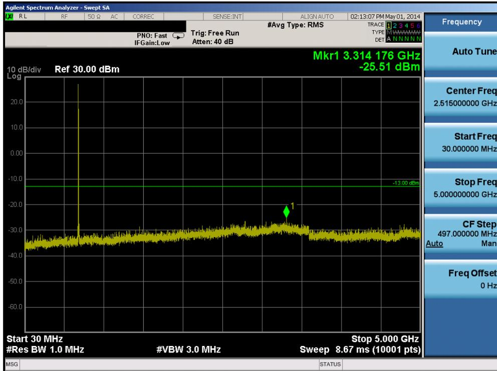
Plot 6-17. Conducted Spurious Plot (Band 17 – 10.0MHz QPSK – RB Size 1, RB Offset 0– Low Channel)
