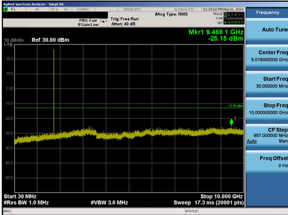
Plot 6-33. Conducted Spurious Plot (Band 4 – 5.0MHz QPSK – RB Size 1, RB Offset 0 – High Channel)
