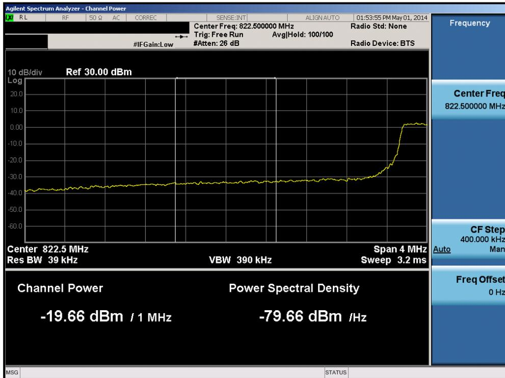
Plot 6-48. Lower Extended Band Edge Plot (Band 5 – 5.0MHz QPSK – RB Size 25)
