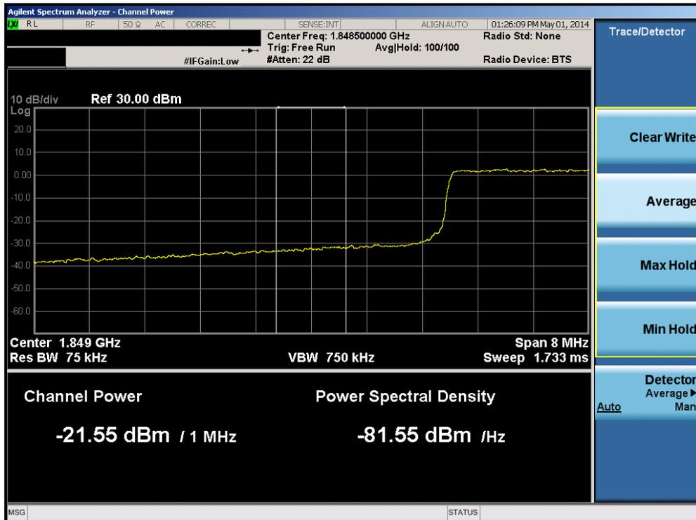
Plot 6-66. Lower Extended Band Edge Plot (Band 2 – 10.0MHz QPSK – RB Size 50)
