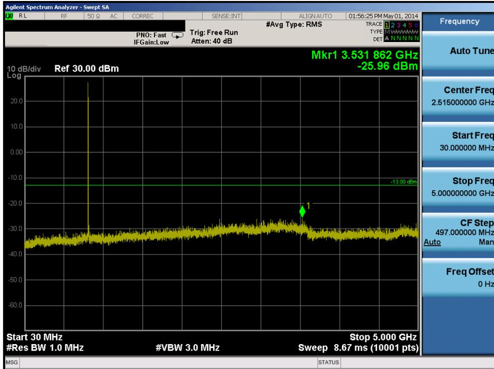
Plot 6-25. Conducted Spurious Plot (Band 5 – 10.0MHz QPSK – RB Size 1, RB Offset 0 – Mid Channel)
