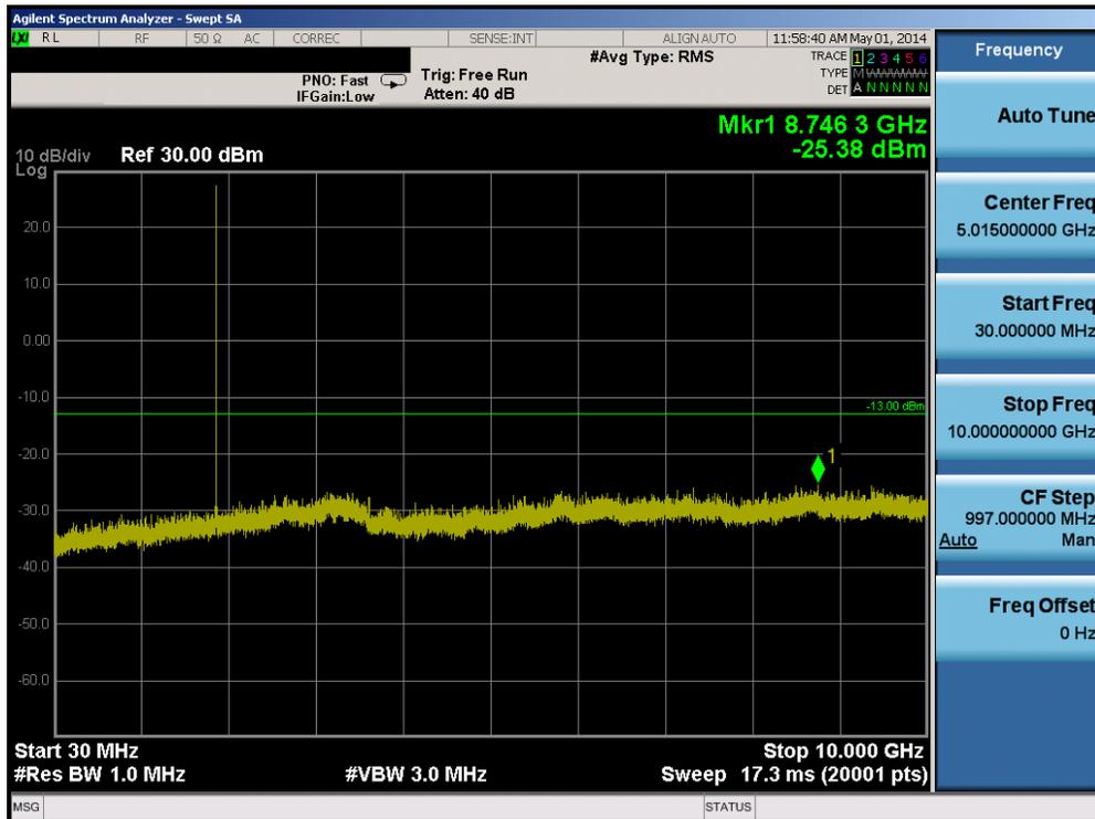
Plot 6-37. Conducted Spurious Plot (Band 2 – 5.0MHz QPSK – RB Size 1, RB Offset 0 – Mid Channel)
