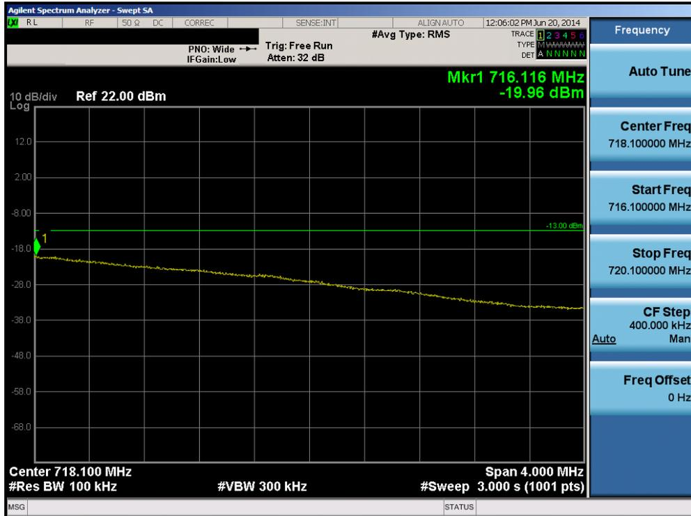
Plot 6-44. Upper Extended Band Edge Plot (Band 17 – 5.0MHz QPSK – RB Size 25)
