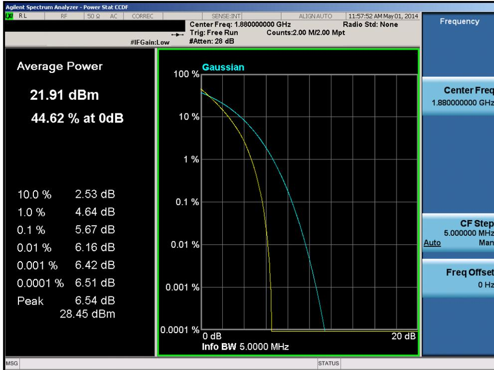
Plot 6-73. PAR Plot (Band 2 – 5.0MHz QPSK – RB Size 25)
