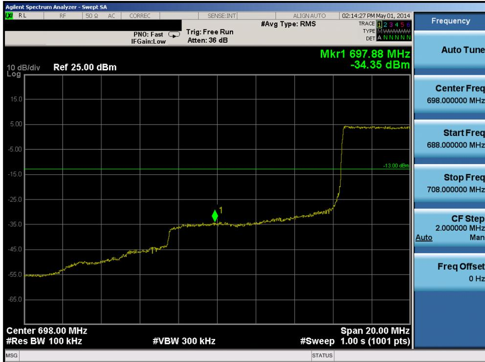
Plot 6-45. Lower Band Edge Plot (Band 17 – 10.0MHz QPSK – RB Size 50)
