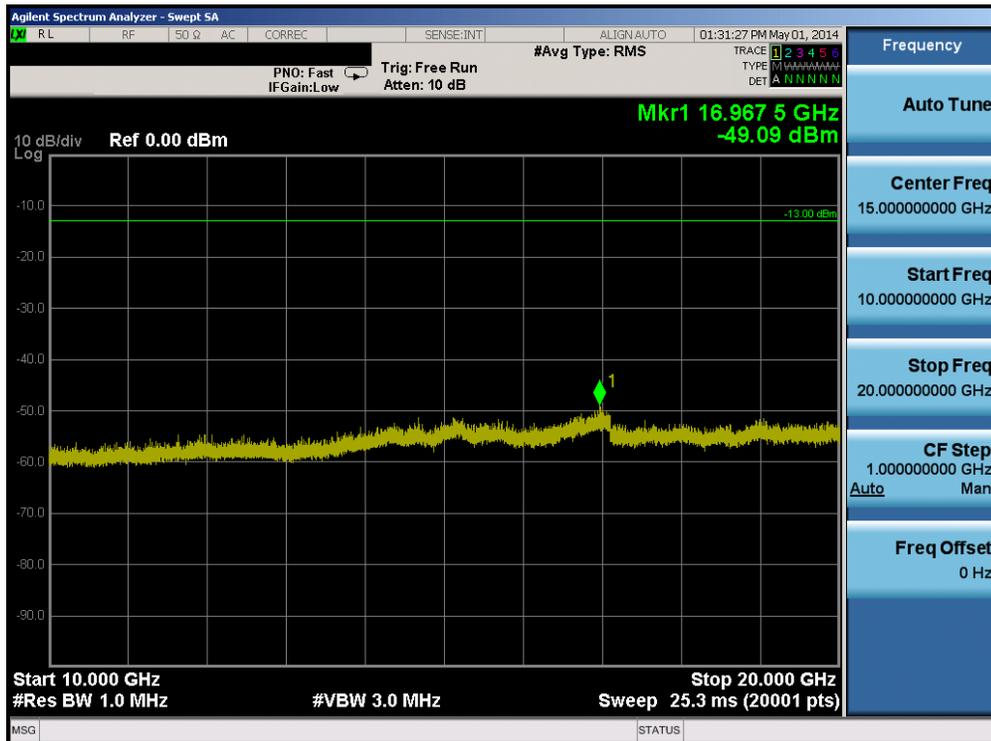
Plot 6-30. Conducted Spurious Plot (Band 4 – 5.0MHz QPSK – RB Size 1, RB Offset 0 – Low Channel)
