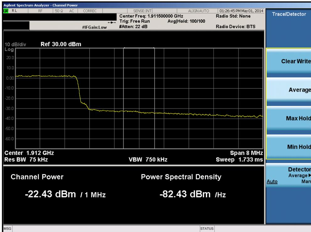
Plot 6-68. Upper Extended Band Edge Plot (Band 2 – 10.0MHz QPSK – RB Size 50)
