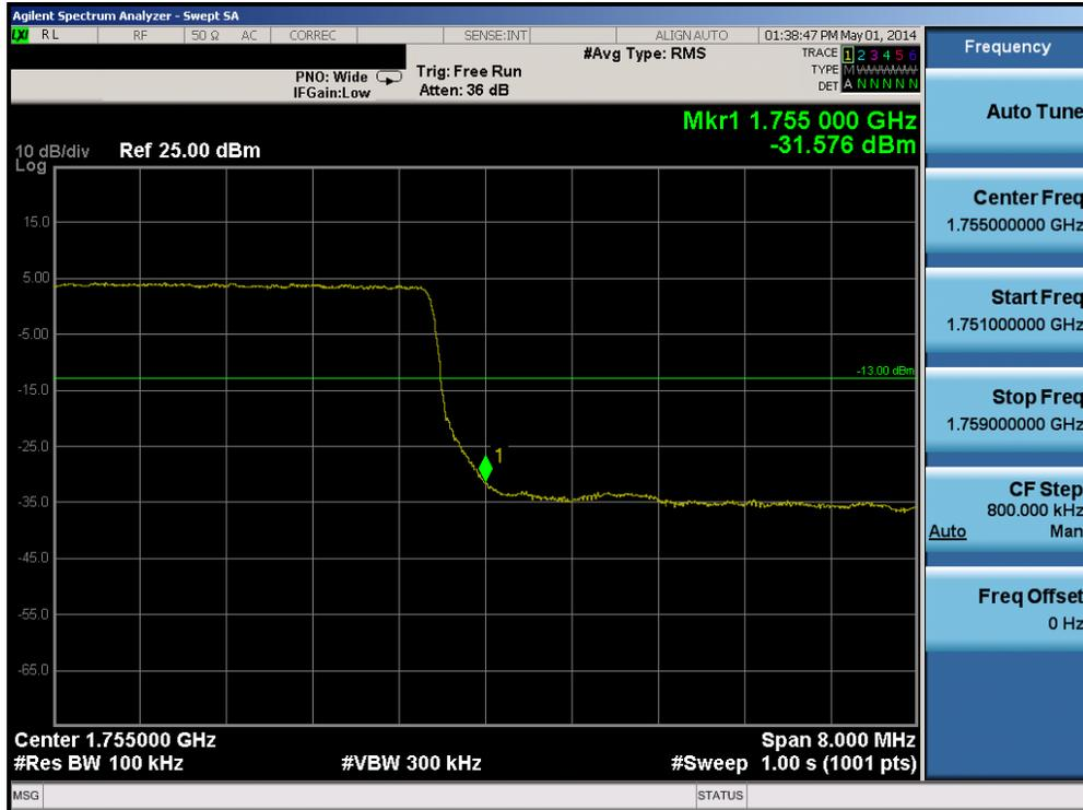
Plot 6-59. Upper Band Edge Plot (Band 4 – 10.0MHz QPSK – RB Size 50)
