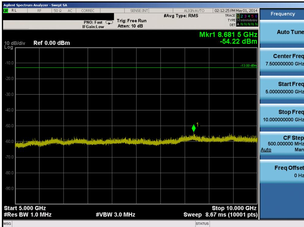
Plot 6-20. Conducted Spurious Plot (Band 17 – 10.0MHz QPSK – RB Size 1, RB Offset 0 – Mid Channel)
