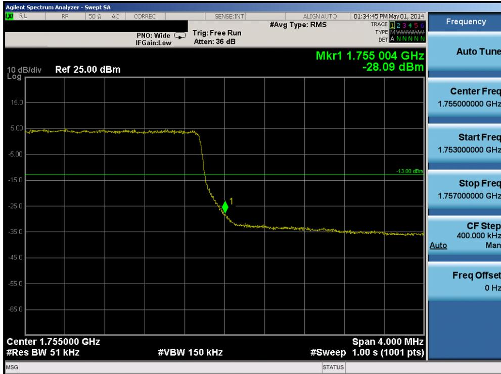
Plot 6-55. Upper Band Edge Plot (Band 4 – 5.0MHz QPSK – RB Size 25)
