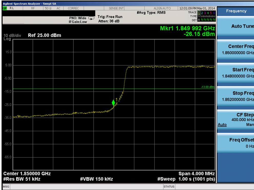
Plot 6-61. Lower Band Edge Plot (Band 2 – 5.0MHz QPSK – RB Size 25)
