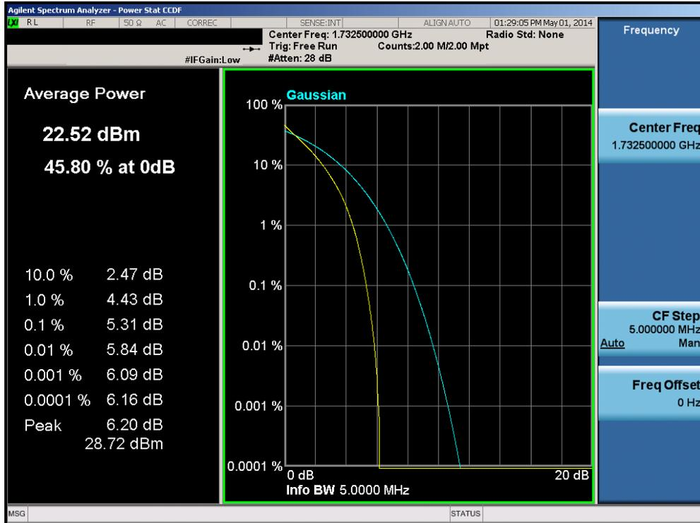
Plot 6-69. PAR Plot (Band 4 – 5.0MHz QPSK – RB Size 25)
