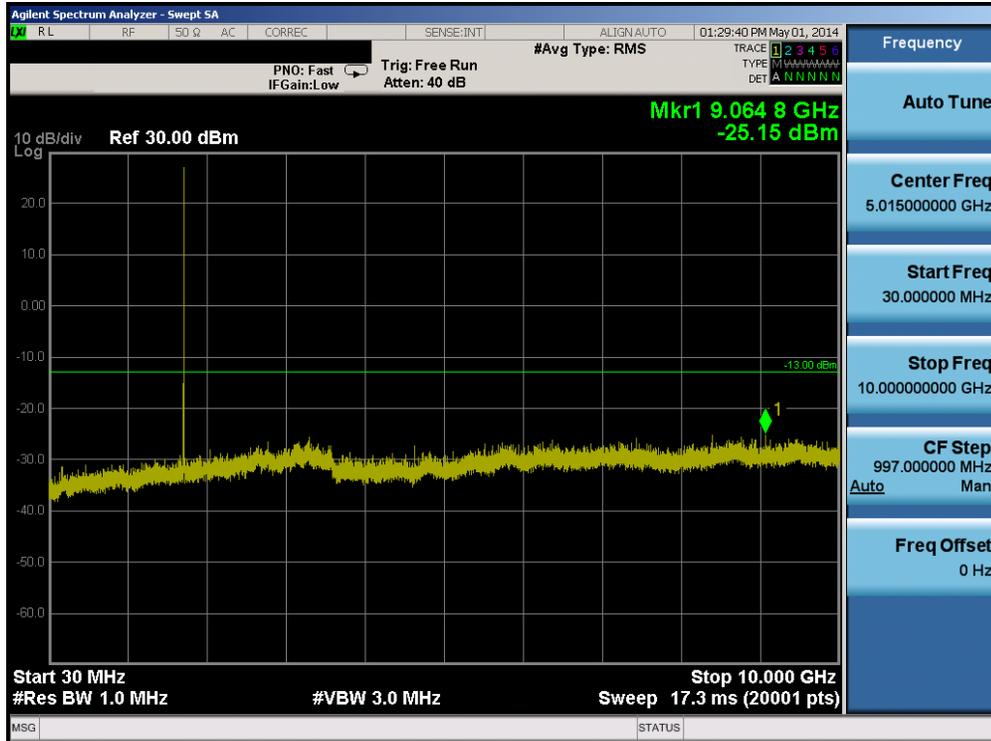
Plot 6-31. Conducted Spurious Plot (Band 4 – 5.0MHz QPSK – RB Size 1, RB Offset 0 – Mid Channel)
