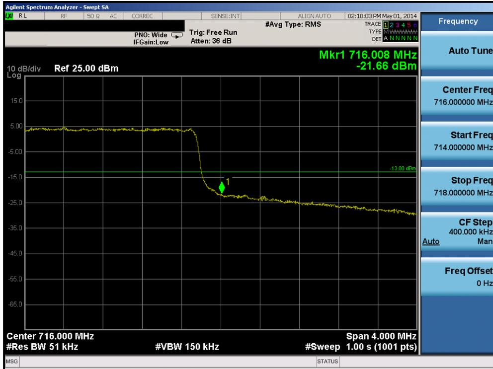
Plot 6-43. Upper Band Edge Plot (Band 17 – 5.0MHz QPSK – RB Size 25)
