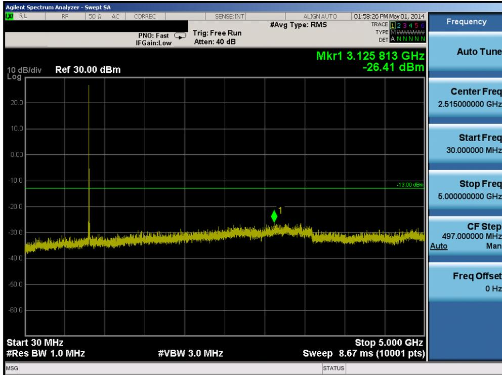
Plot 6-23. Conducted Spurious Plot (Band 5 – 10.0MHz QPSK – RB Size 1, RB Offset 0– Low Channel)
