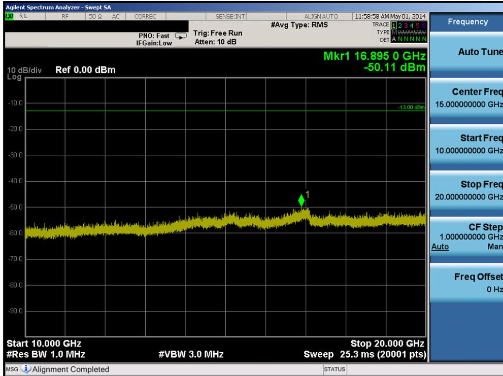
Plot 6-38. Conducted Spurious Plot (Band 2 – 5.0MHz QPSK – RB Size 1, RB Offset 0 – Mid Channel)
