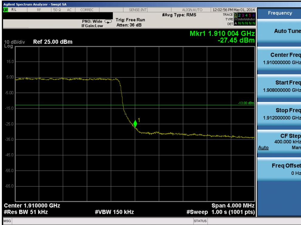
Plot 6-63. Upper Band Edge Plot (Band 2 – 5.0MHz QPSK – RB Size 25)
