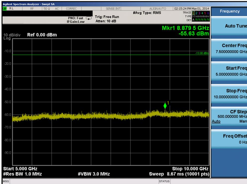
Plot 6-22. Conducted Spurious Plot (Band 17 – 10.0MHz QPSK – RB Size 1, RB Offset 0 – High Channel)
