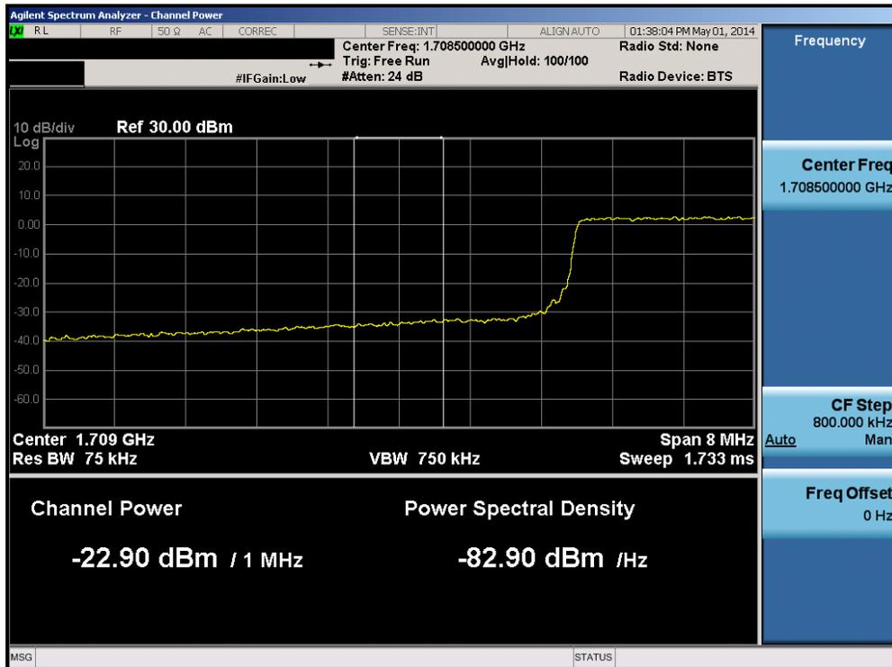
Plot 6-58. Lower Extended Band Edge Plot (Band 4 – 10.0MHz QPSK – RB Size 50)
