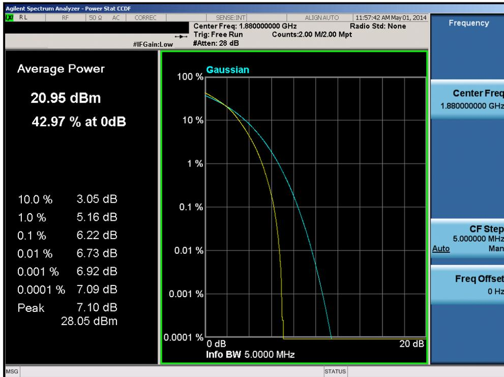
Plot 6-74. PAR Plot (Band 2 – 5.0MHz 16-QAM – RB Size 25)
