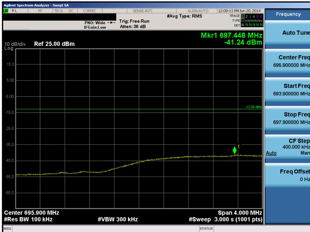
Plot 6-42. Lower Extended Band Edge Plot (Band 17 – 5.0MHz QPSK – RB Size 25)
