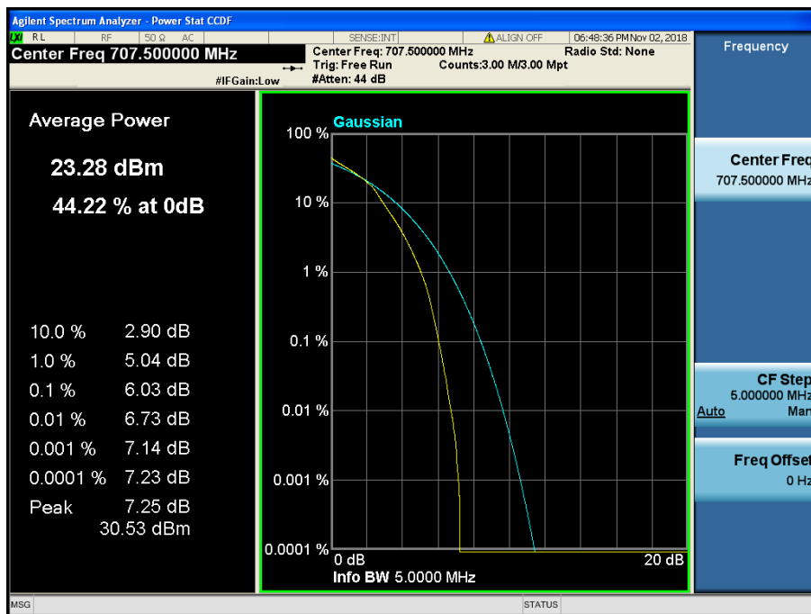
LTE Band 12,17 / 5 MHz / 16QAM - RB Size 25
