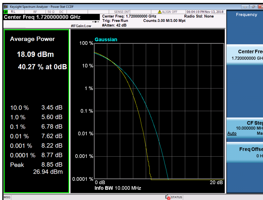
LTE Band 4 / 20 MHz / 16QAM - RB Size 100
