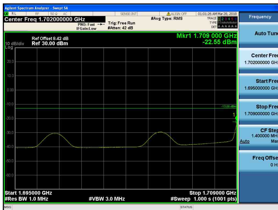
LTE Band 4 / 15MHz / QPSK - RB Size/Offset (1/0)
