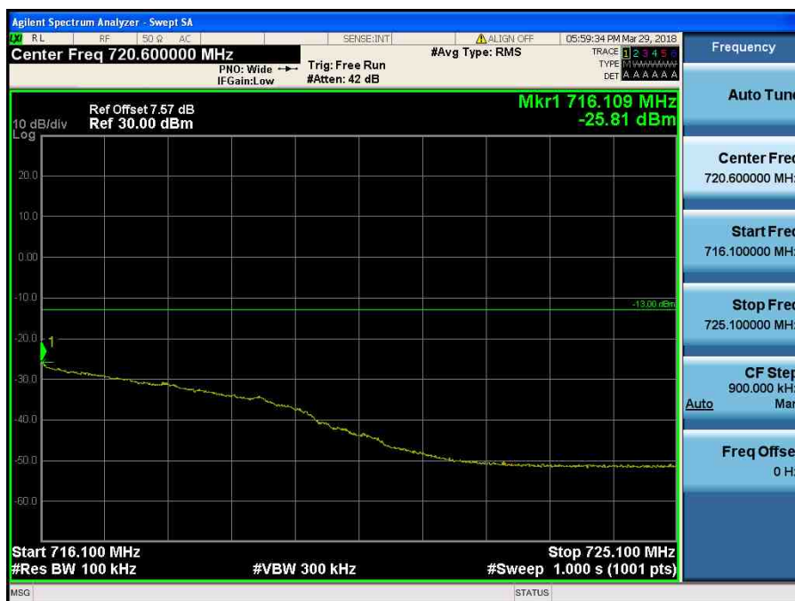
LTE Band 12,17 / 10MHz / QPSK - RB Size/Offset (25/25)
