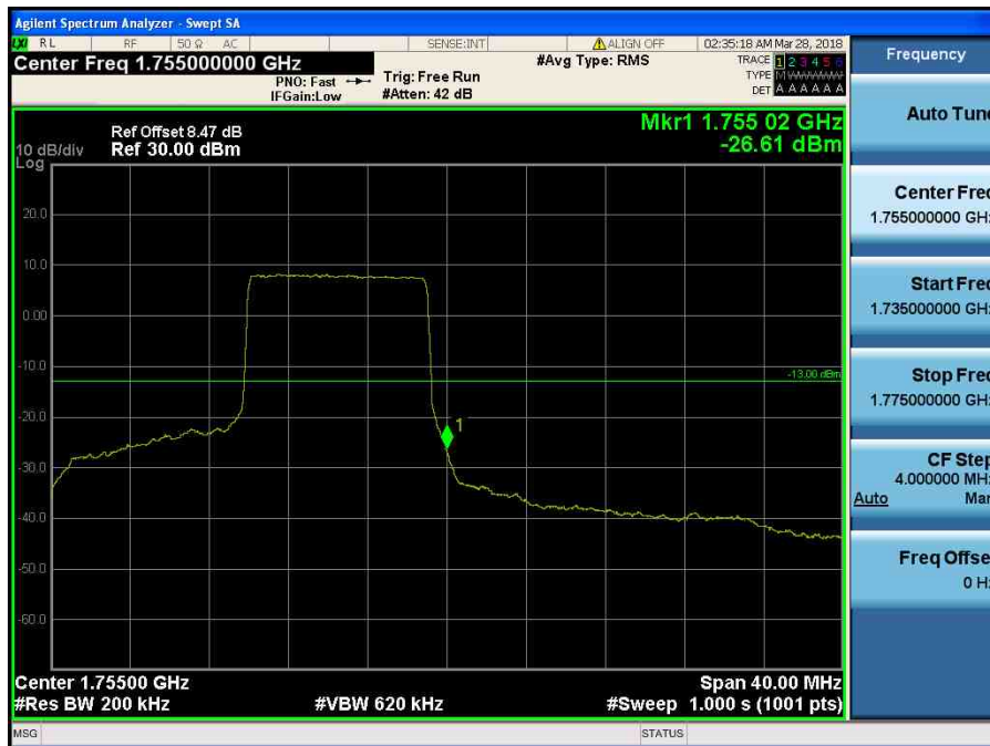
LTE Band 4 / 20MHz / QPSK - RB Size/Offset (50/50)
