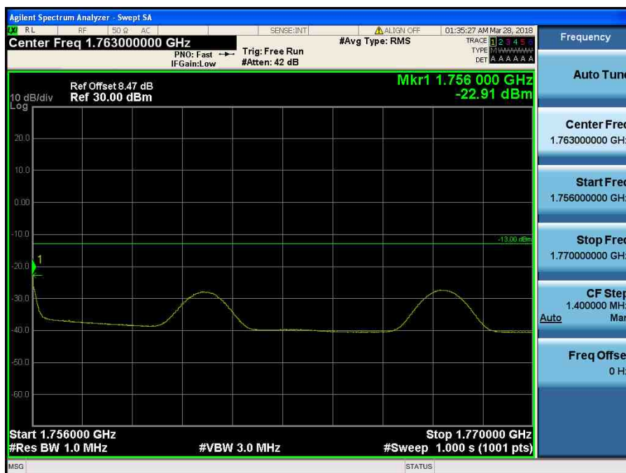
LTE Band 4 / 15MHz / QPSK - RB Size/Offset (1/74)
