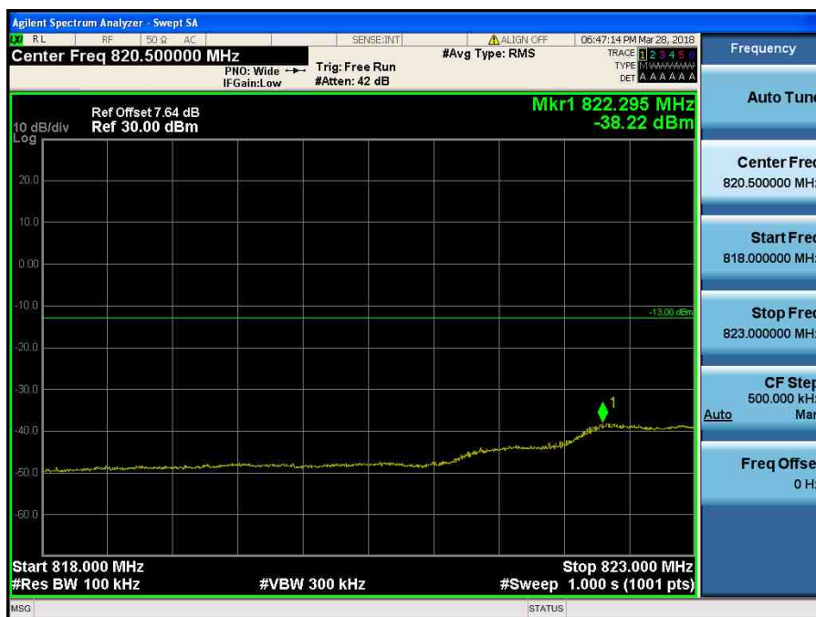
LTE Band 5 / 1.4MHz / QPSK - RB Size/Offset (6/0)
