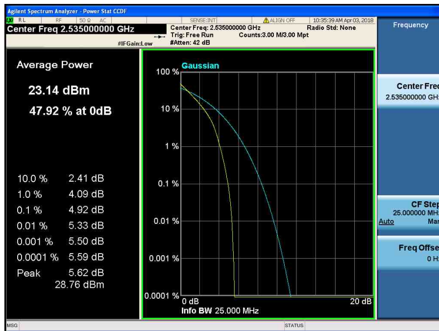
LTE Band 7 / 15 MHz / QPSK - RB Size 75
