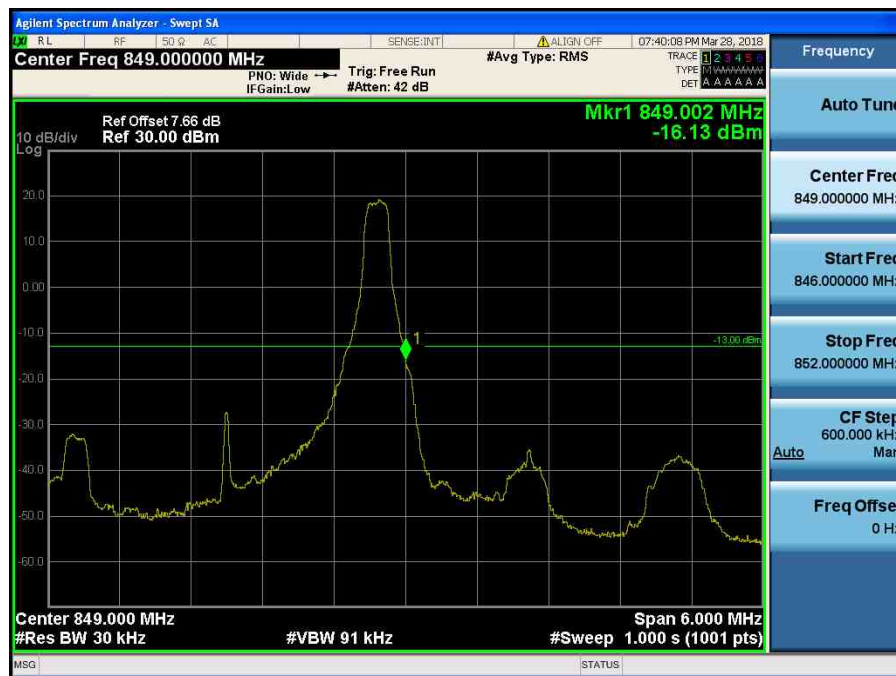
LTE Band 5 / 3MHz / QPSK - RB Size/Offset (1/14)
