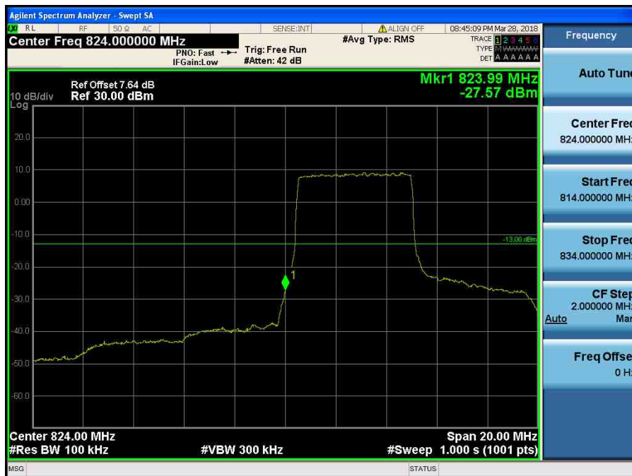
LTE Band 5 / 10MHz / QPSK - RB Size/Offset (25/0)
