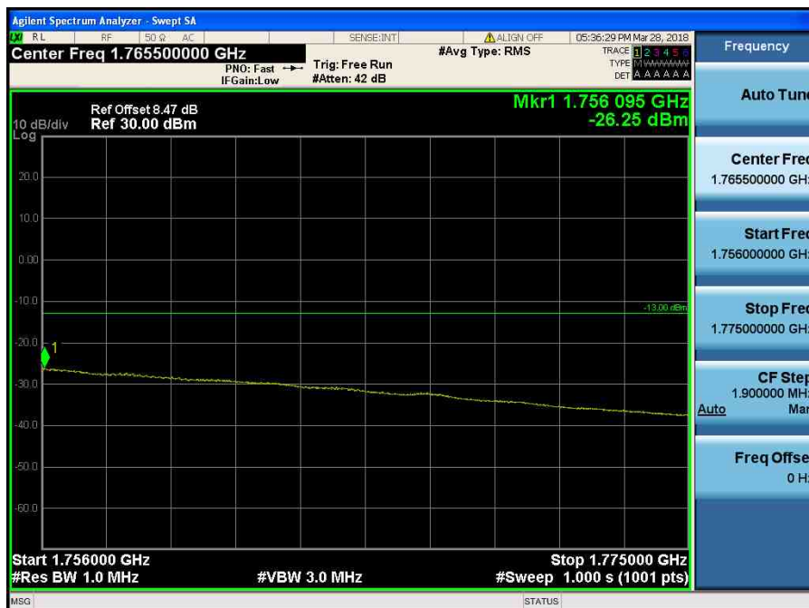
LTE Band 4 / 20MHz / 64QAM - RB Size/Offset (50/50)
