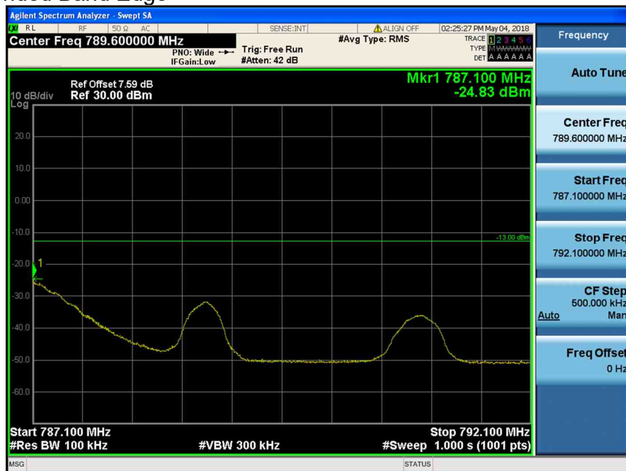
LTE Band 13 / 5MHz / QPSK - RB Size/Offset (1/24)
