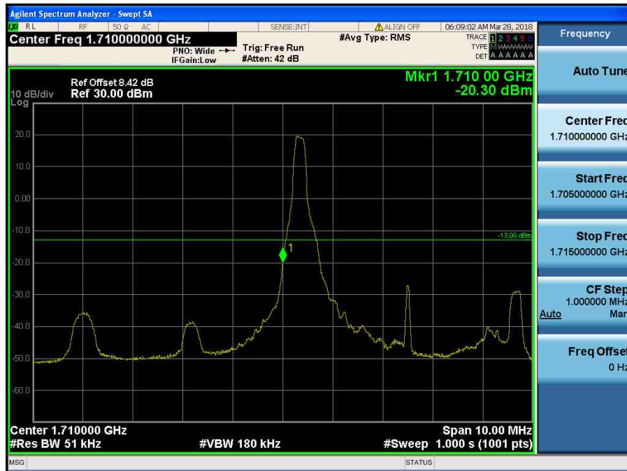
LTE Band 4 / 5MHz / 16QAM Offset/Size (1/0)
