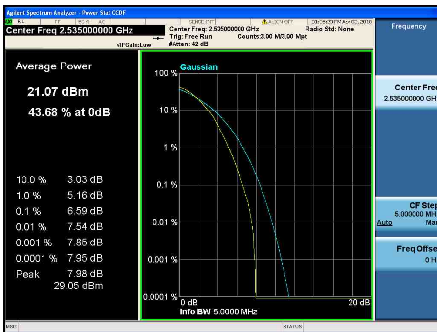
LTE Band 7 / 5 MHz / 64QAM - RB Size 25
