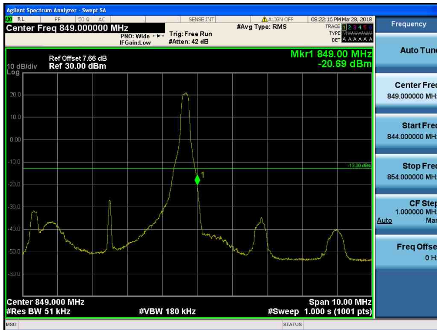
LTE Band 5 / 5MHz / QPSK - RB Size/Offset (1/24)
