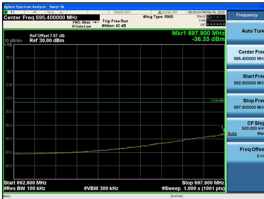
LTE Band 12 / 1.4MHz / 64QAM - RB Size/Offset (6/0)
