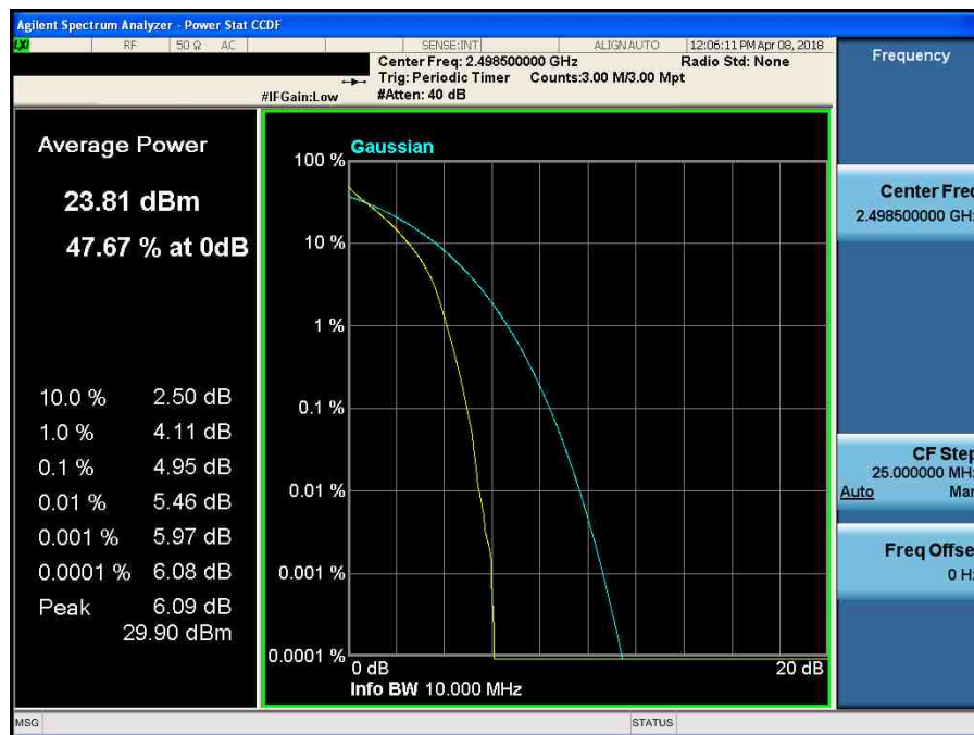
LTE Band 41 / 5 MHz / QPSK - RB Size 25
