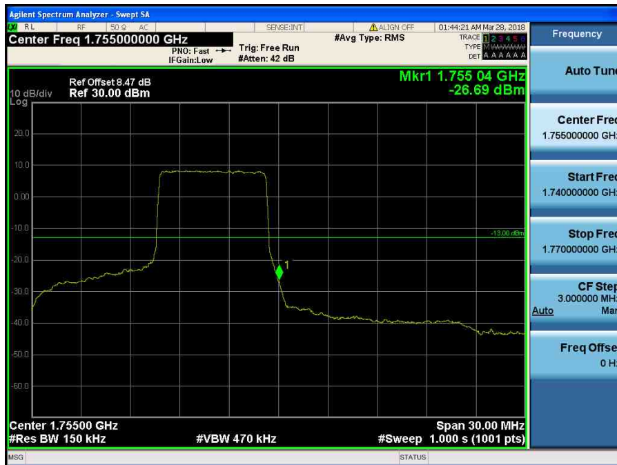
LTE Band 4 / 15MHz / QPSK - RB Size/Offset (36/39)
