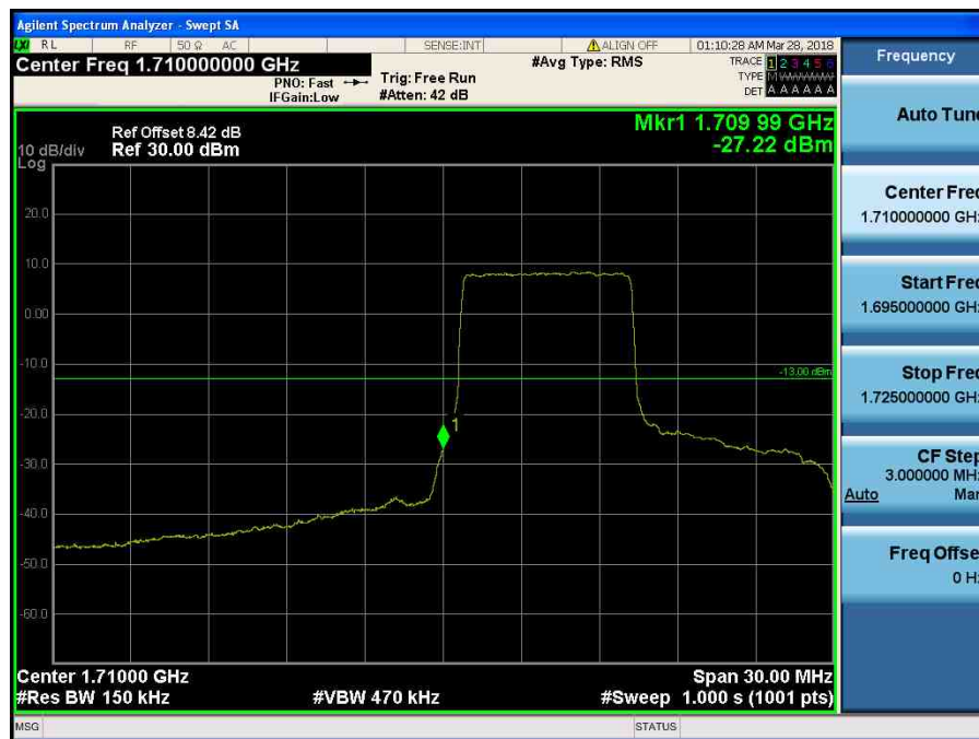
LTE Band 4 / 15MHz / QPSK - RB Size/Offset (36/0)
