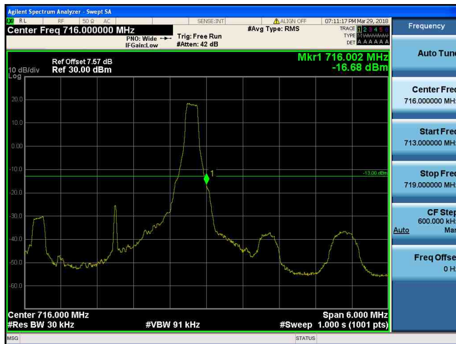
LTE Band 12 / 3MHz / 16QAM - RB Size/Offset (1/14)
