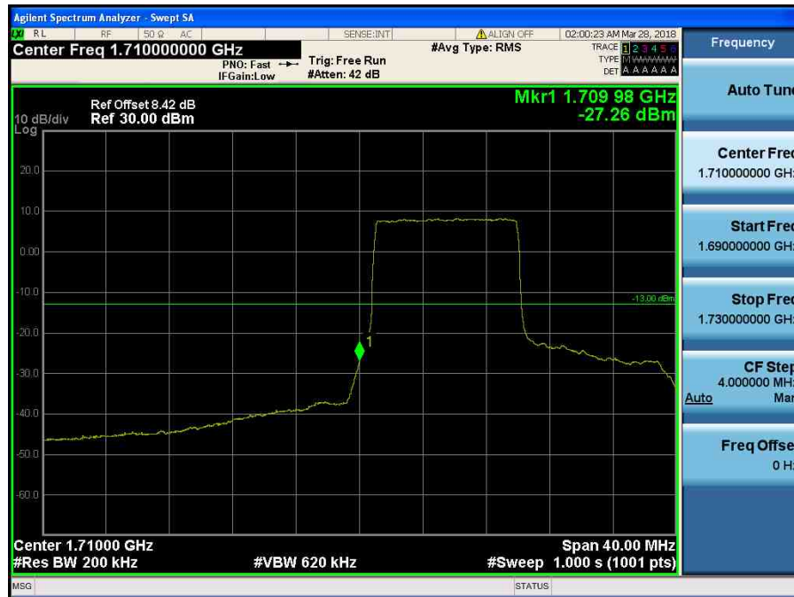
LTE Band 4 / 20MHz / QPSK - RB Size/Offset (50/0)
