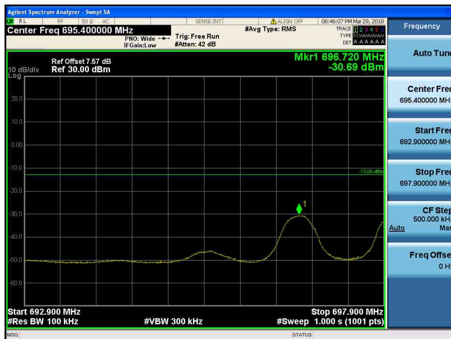
LTE Band 12 / 3MHz / 16QAM - RB Size/Offset (1/0)
