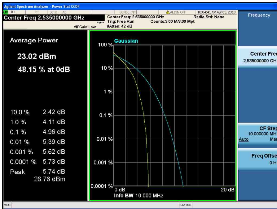
LTE Band 7 / 10 MHz / QPSK - RB Size 50
