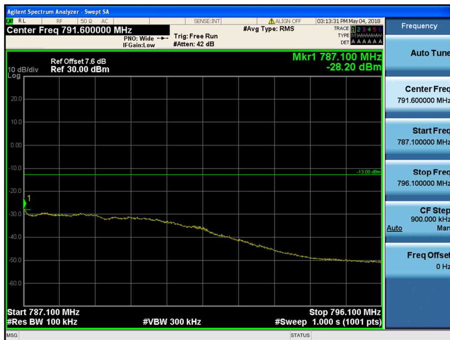
LTE Band 13 / 10MHz / QPSK - RB Size/Offset (50/0)
