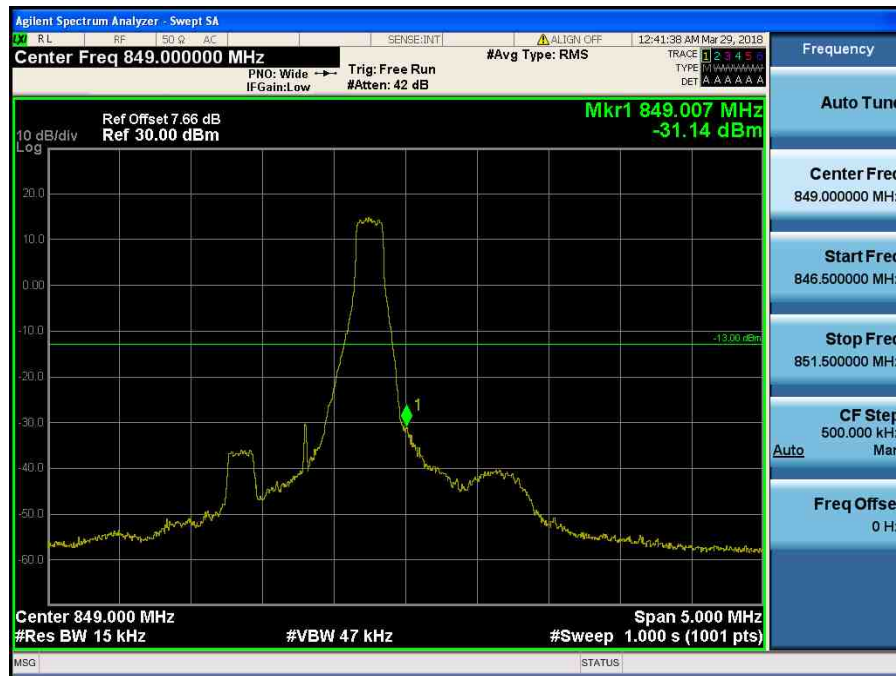
LTE Band 5 / 1.4MHz / 64QAM - RB Size/Offset (1/5)
