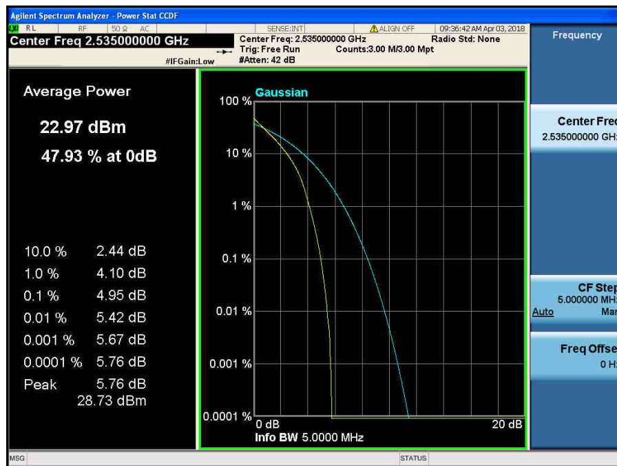
LTE Band 7 / 5 MHz / QPSK - RB Size 25
