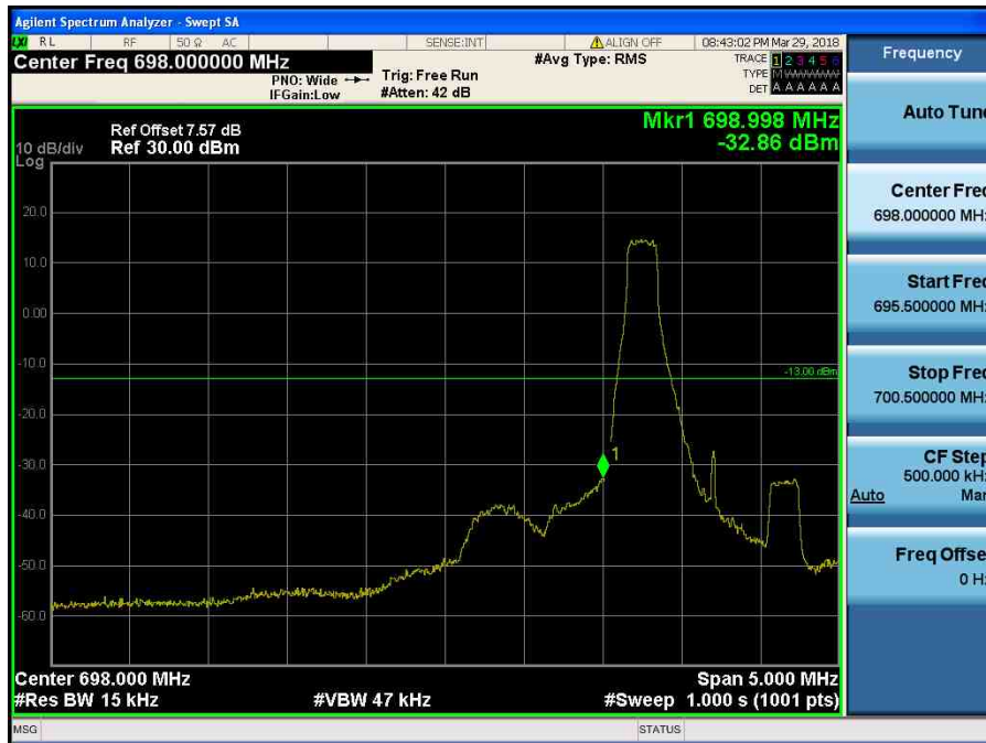
LTE Band 12 / 1.4MHz / 64QAM - RB Size/Offset (1/0)
