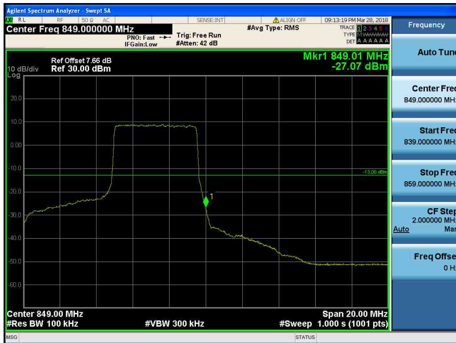
LTE Band 5 / 10MHz / QPSK - RB Size/Offset (25/25)
