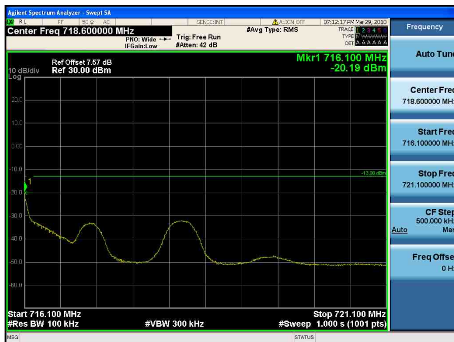
LTE Band 12 / 3MHz / 16QAM - RB Size/Offset (1/14)
