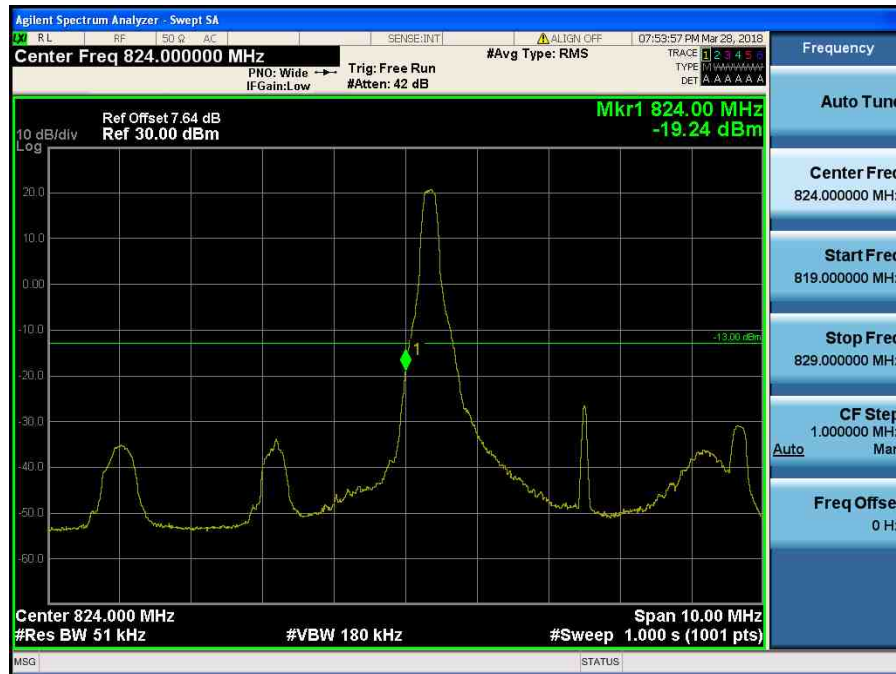
LTE Band 5 / 5MHz / QPSK Offset/Size (1/0)
