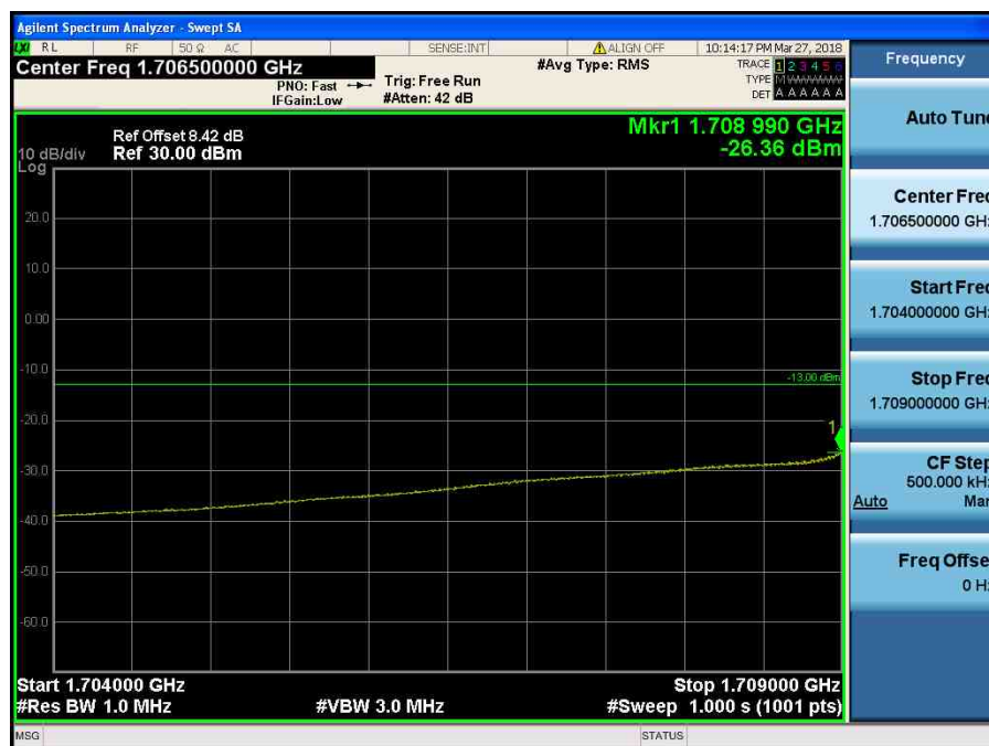
LTE Band 4 / 3MHz / QPSK - RB Size/Offset (8/4)
