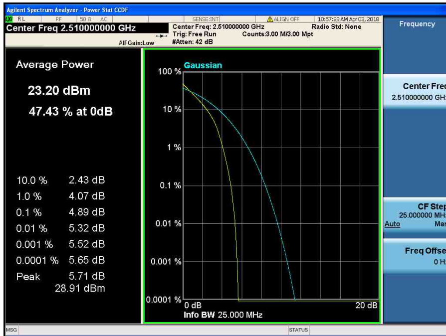
LTE Band 7 / 20 MHz / QPSK - RB Size 100
