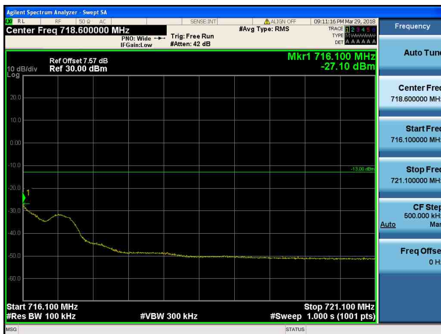
LTE Band 12 / 1.4MHz / 64QAM - RB Size/Offset (1/5)
