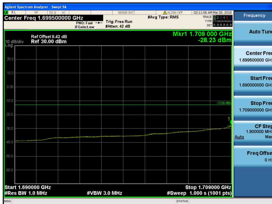
LTE Band 4 / 20MHz / QPSK - RB Size/Offset (100/0)
