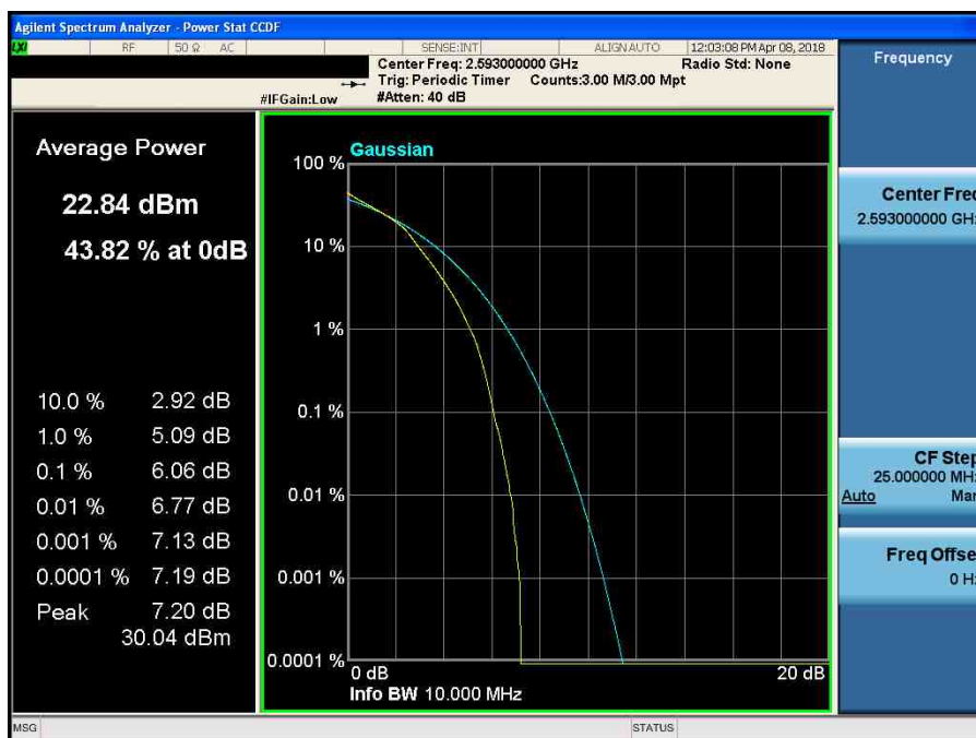
LTE Band 41 / 10 MHz / 16QAM - RB Size 50
