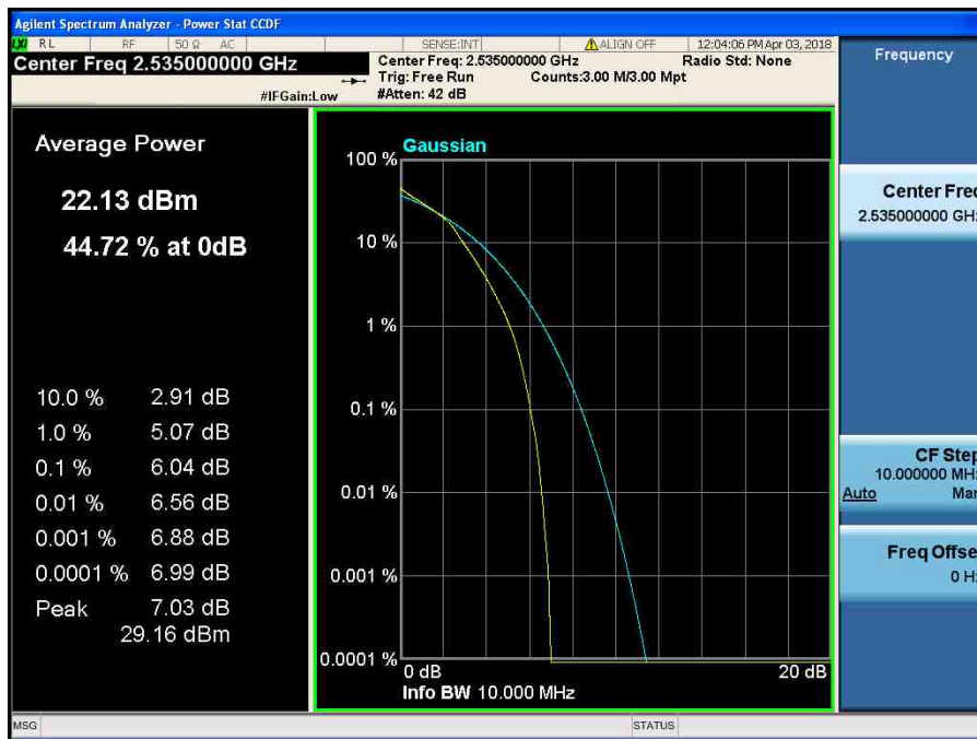
LTE Band 7 / 10 MHz / 16QAM - RB Size 50
