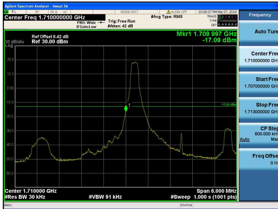
LTE Band 4 / 3MHz / QPSK - RB Size/Offset (1/0)
