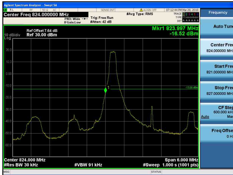
LTE Band 5 / 3MHz / QPSK - RB Size/Offset (1/0)
