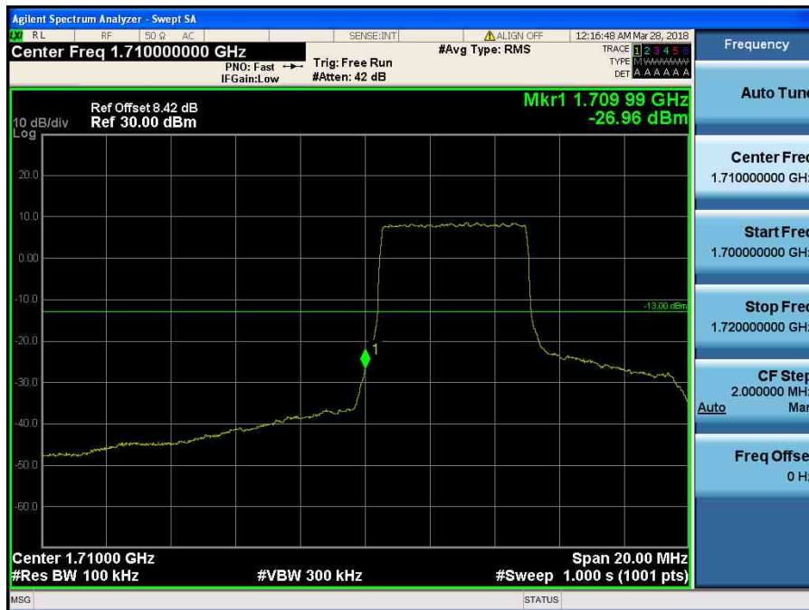
LTE Band 4 / 10MHz / QPSK - RB Size/Offset (25/0)
