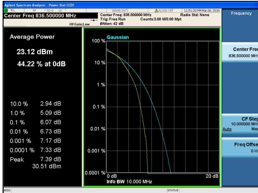
LTE Band 5 / 10 MHz / 16QAM - RB Size 50
