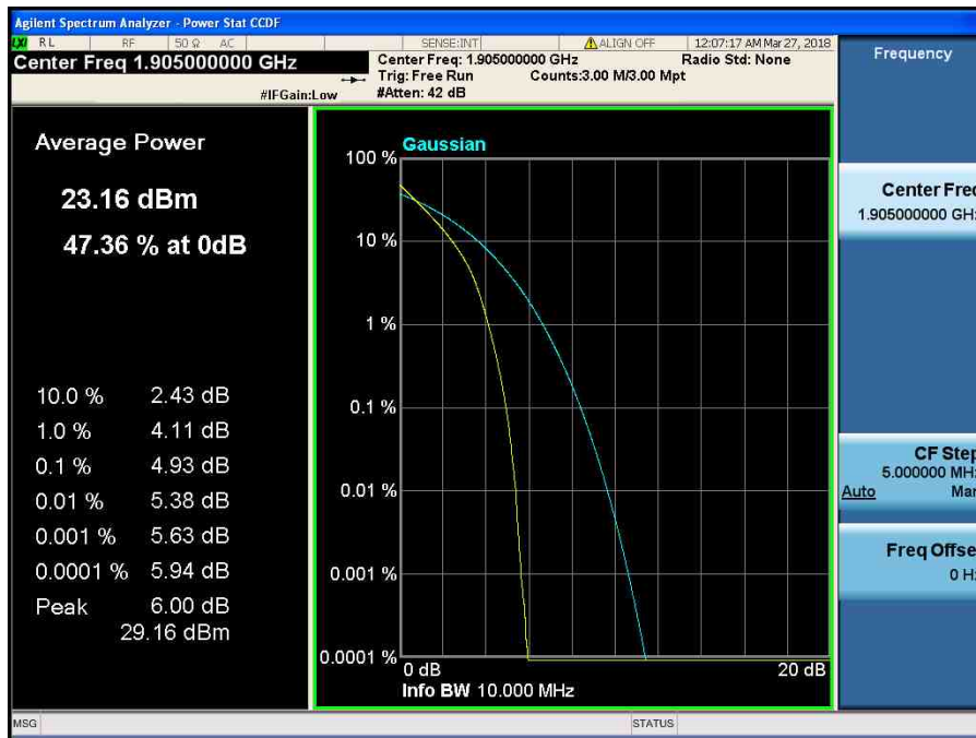
LTE Band 2 / 10 MHz / QPSK - RB Size 50
