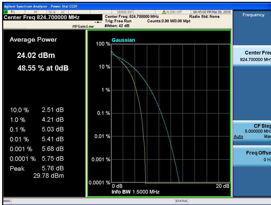
LTE Band 5 / 1.4 MHz / QPSK - RB Size 6
