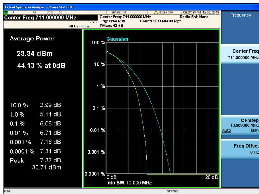
LTE Band 12,17 / 10 MHz / 16QAM - RB Size 50
