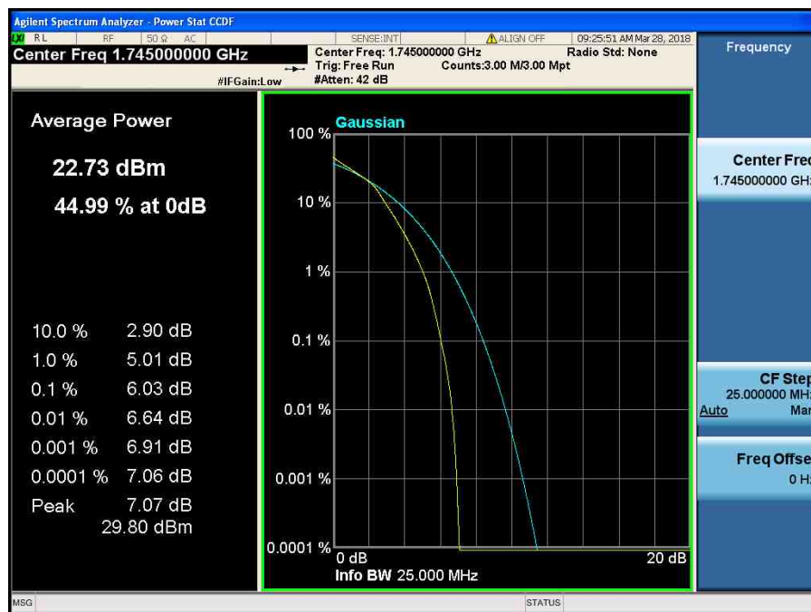
LTE Band 4 / 20 MHz / 16QAM - RB Size 100
