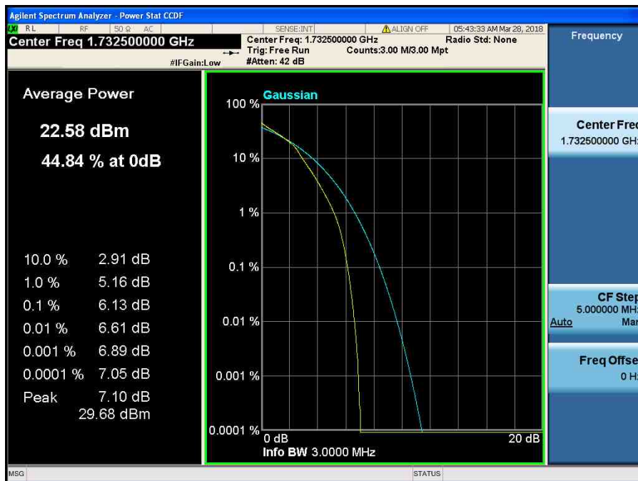
LTE Band 4 / 3 MHz / 16QAM - RB Size 15
