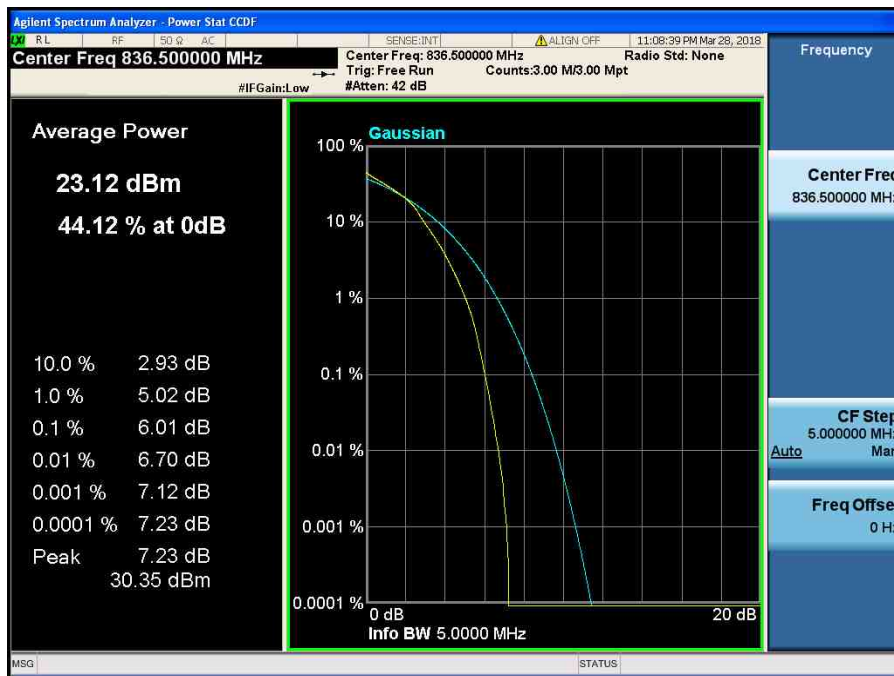
LTE Band 5 / 5 MHz / 16QAM - RB Size 25
