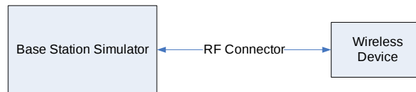
Figure 9-2 Power Measurement Setup
