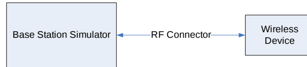
Figure 9-4 Power Measurement Setup
