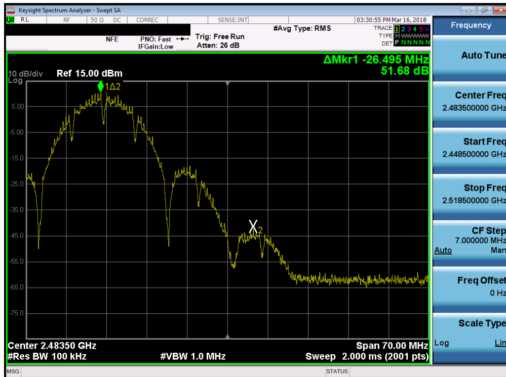
Plot 7-44. Band Edge Plot (802.11b – Ch. 11)
