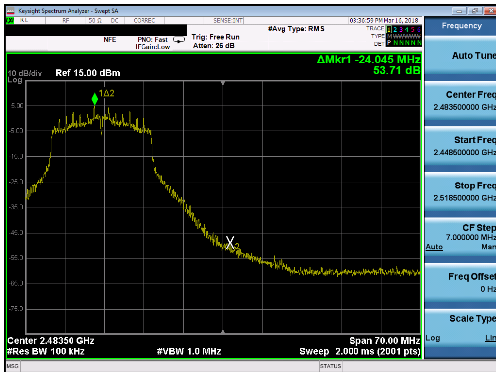
Plot 7-48. Band Edge Plot (802.11n (2.4GHz) – Ch. 11)
